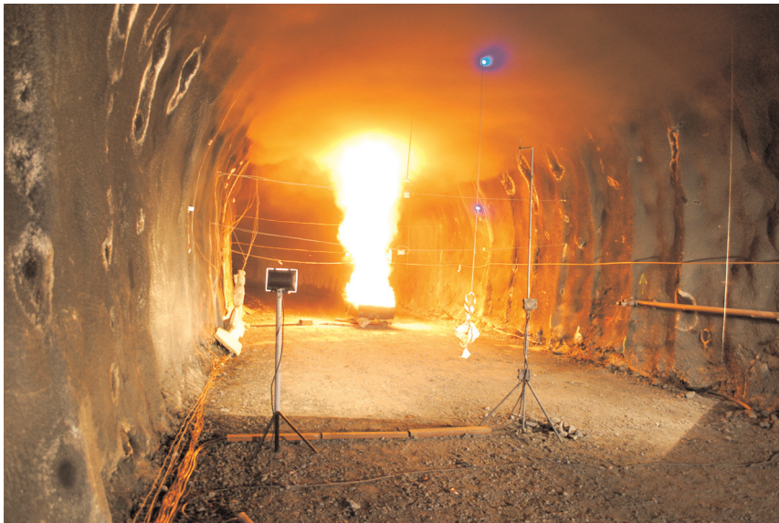
Figure 12.4 Pool fire test in La Ribera del Folgoso Tunnel (Photograph courtesy of Jimmy Jönsson, ArupFire Madrid)
