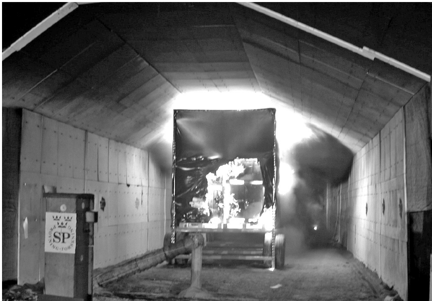
Figure 12.3 Fire experiment (test 3) in the Runehamar Tunnel, Norway (Photograph courtesy of Haukur Ingason)
