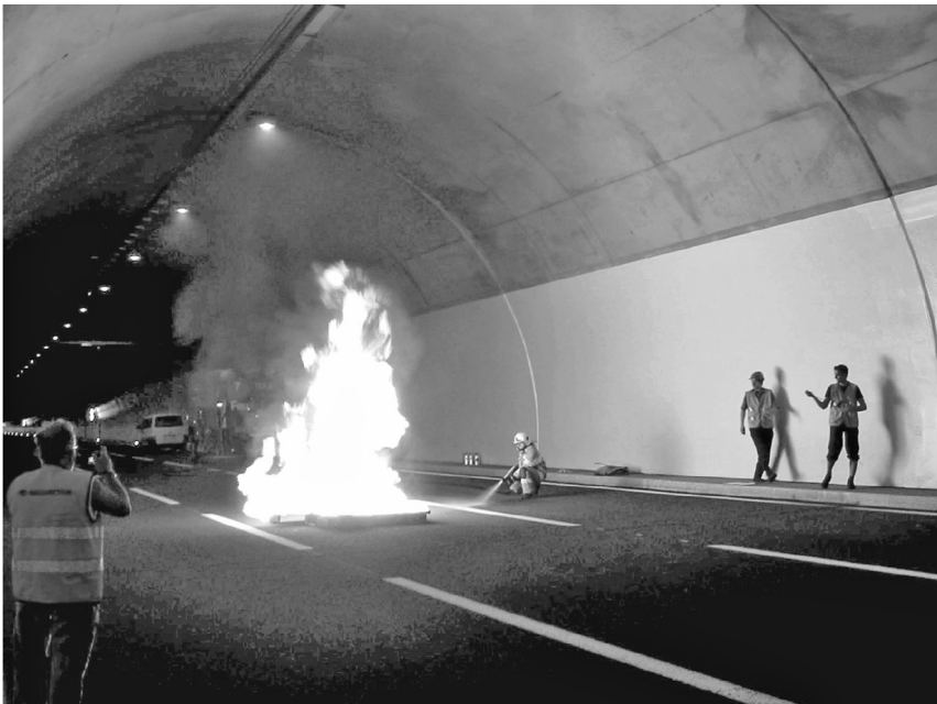
Figure 12.5 Fire experiment carried out to test/commission the linear fire-detection system in the Baregg Tunnel, near Baden, Switzerland (Photograph courtesy of John Day)
