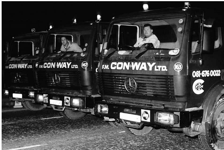
Figure 5.4 Loaded lorries in use as a load test.
