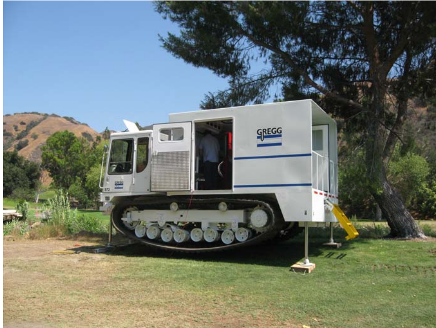
Figure 11 Track mounted 20 ton CPT unit
