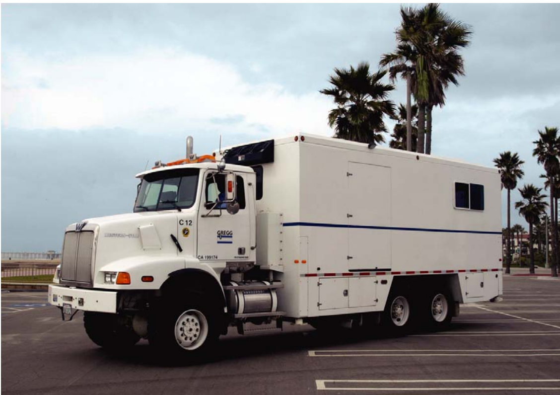
Figure 10 Truck mounted 25 ton CPT unit
