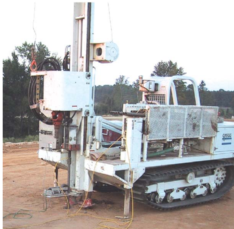
Figure 12 Small anchored drill-rig unit
