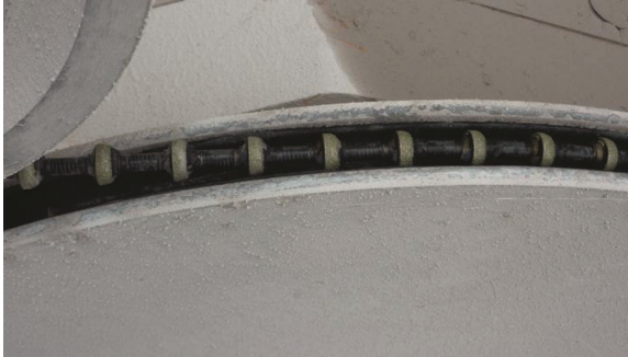
Fig. 8. Diamond wire inside flywheel.
