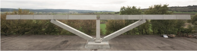
Fig. 15. Large-scale model of the balanced lift part of the Lafnitz Bridge
