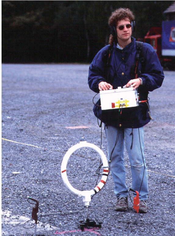
Fig. 10.2. The scalar RMT instrument developed by the Centre of Hydrogeology at the University of Neuchâtel (CHYN)
