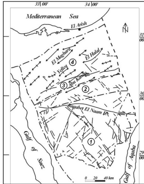
Fig. 14.25. Structural map of Central Sinai (after Shata 1956); 1: the stable foreland, 2: the gently folded zone, 3: the fractured zone, 4: the strongly folded zone
