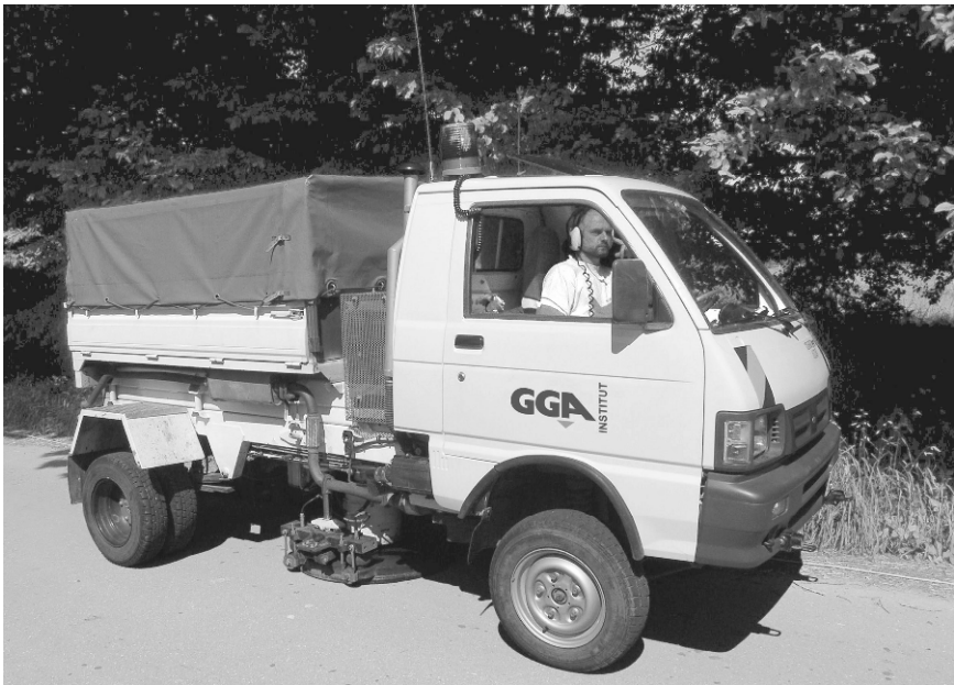
Fig. 2.5. Example for seismic sources applied in near surface prospecting: small Vibroseis ® truck (GGA-Institut, Hannover)
