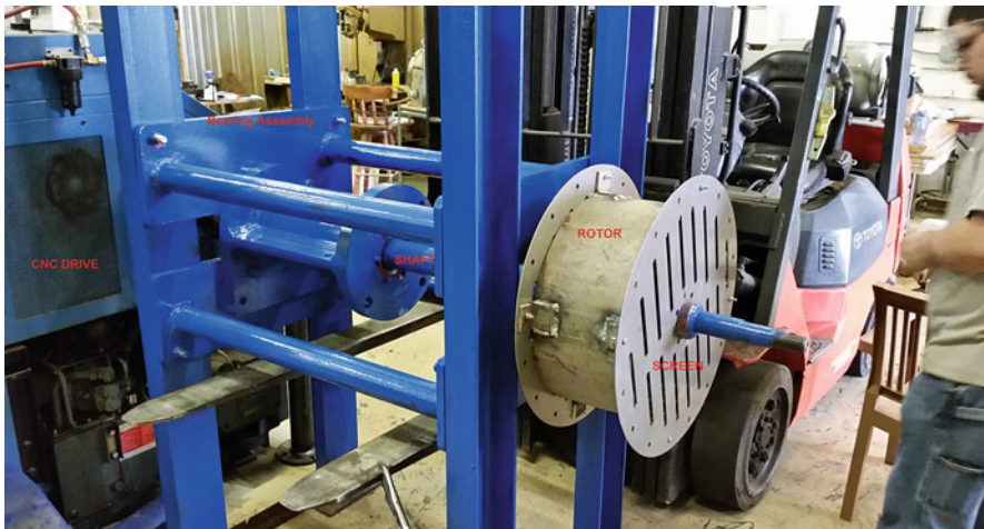
Fig. 5 Construction ablation machine connected to Siemens computer numerical control drive
