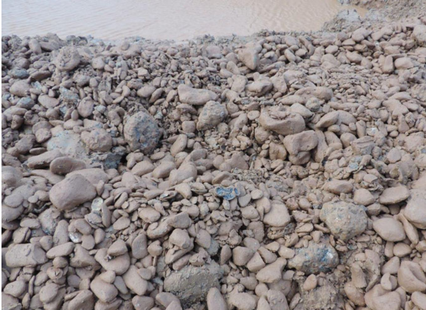
Fig. 5 Balls of clays formed during dredging with a range of diameter of 125–200 mm
