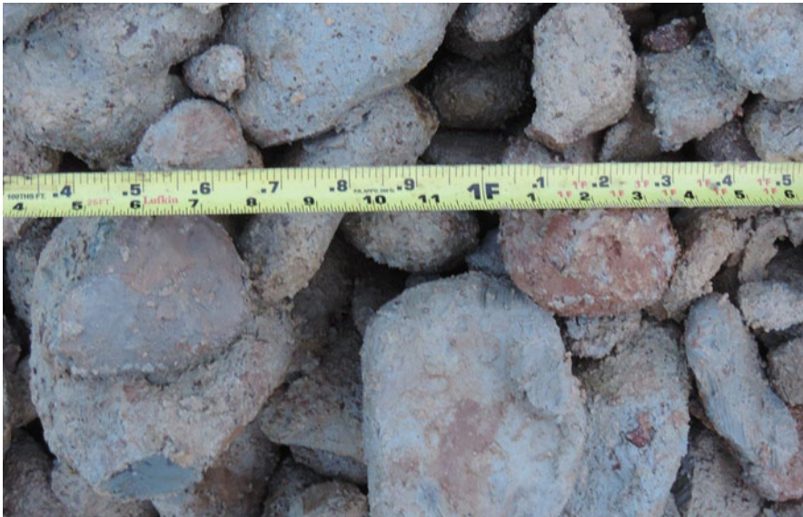
Fig. 2 Ball of clays formed during dredging high-plasticity clays in Texas. Scale is in feet (1F = 304 mm) and inches (25.4 mm)
