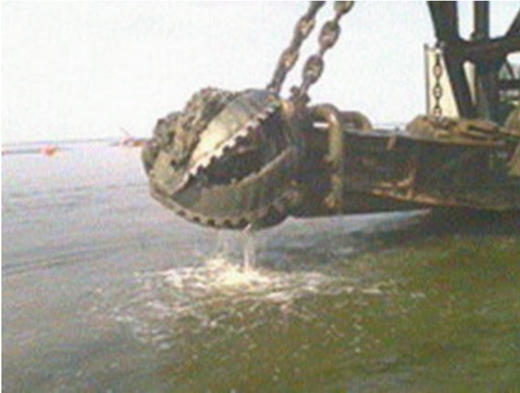
Fig. 3 Cutter and collected samples of clay from hydraulic dredging barge in Texas (USA)
