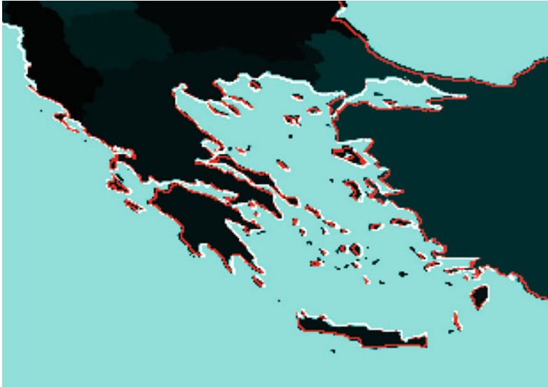
Fig. 1.13 Zoomed-in part of the final image produced by the georegistration procedure. It can be seen that the image of the Mediterranean countries has been spatially matched with the image of the Mediterranean coastline (Fig. 1.11a)
