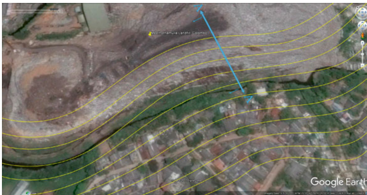
Fig. 3 Contours indicating the movement of failed wedge in the southwest direction ( Source Google Earth)
