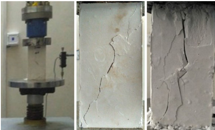
Fig. 9 Crack growth study in gypsum plaster specimen with pre-existing single and double flaws under uniaxial loading
