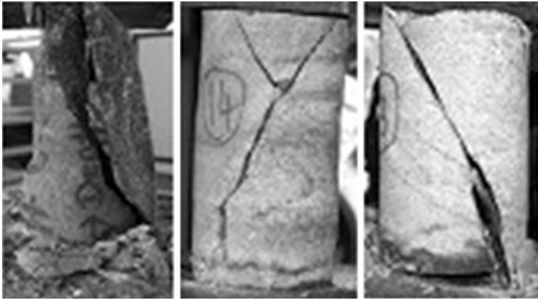
Fig. 3 Some typical failure modes of granulate rock specimens observed after axial compression testing
