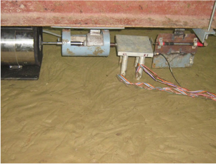
Fig. 5 Experimental setup for lateral dynamic load test (Chandrasekaran et al. 2013)
