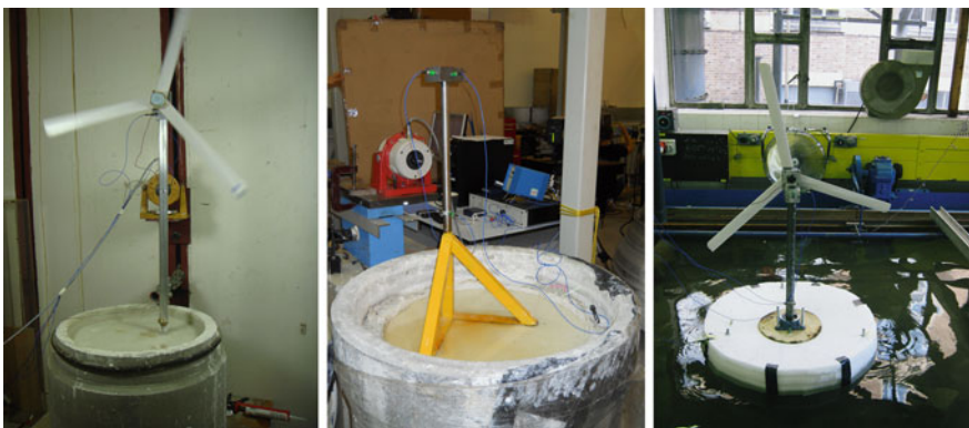
Fig. 15 Examples of scaled model tests; a monopile-supported wind turbine with blades; b asymmetric tripod-supported wind turbine where the RNA mass is simulated by a top mass; c model of a floating turbine
