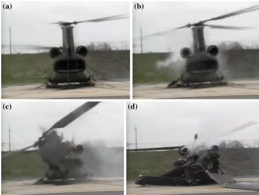
Fig. 12 Ground resonance due to a helicopter
