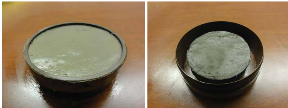
Figure 4.11 Shrinkage limit equipment and test.
