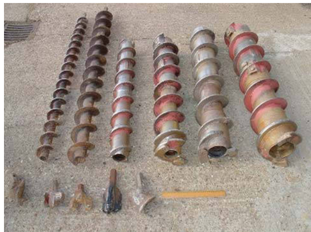
Figure 6.4 Hollow stem augers. (Courtesy of C. Jeffries, Environmental Sampling Ltd.)
