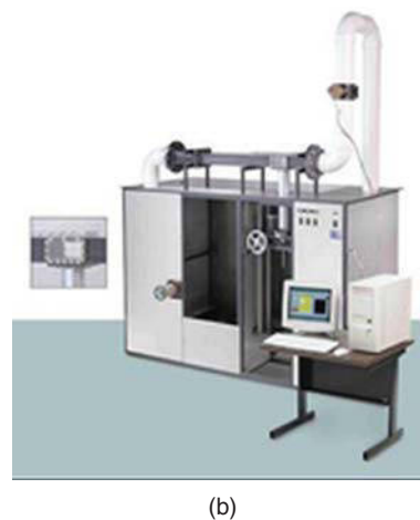
Figure 23.3 Erosion function apparatus to measure erodibility (Briaud et al. 1999).
