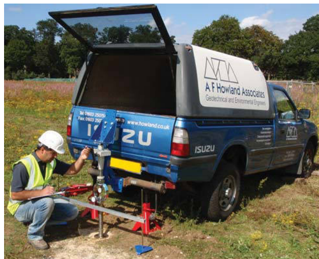
Figure 7.27 CBR test in the field. (Courtesy of A F Howland Company.)
