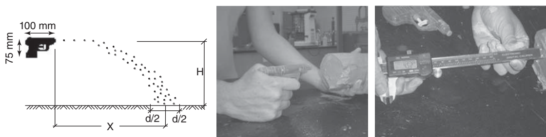
Figure 7.29 Pocket erodometer test.
