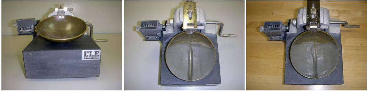
Figure 4.9 Liquid limit apparatus and test.
