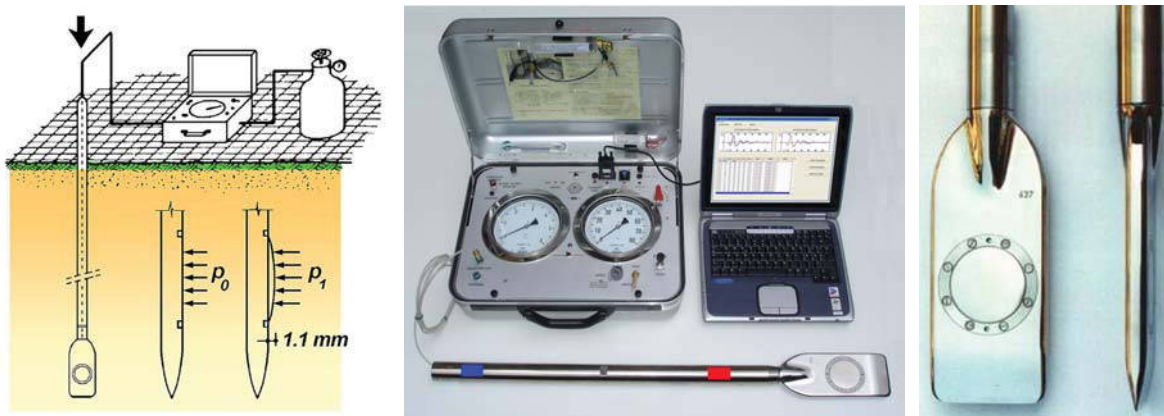
Figure 7.15 Dilatometer test and equipment. (Courtesy of Dr. Sylvano Marchetti, www.marchetti-dmt.it )
