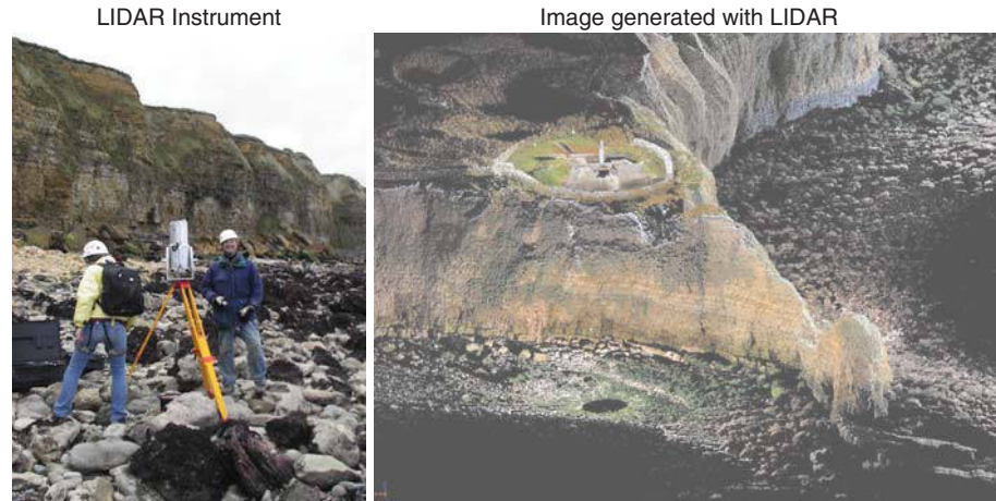
Figure 8.21 Example of LIDAR instrument and result: (a) LIDAR instrument. (b) Image generated with LIDAR. (Courtesy of Professor Robert Warden, Texas A&M University)
