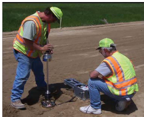
Figure 7.35 Falling weight deflectometer for soil modulus: (a) Principle. (b) Equipment. (b: Courtesy of Minnesota Department of Transportation.)
