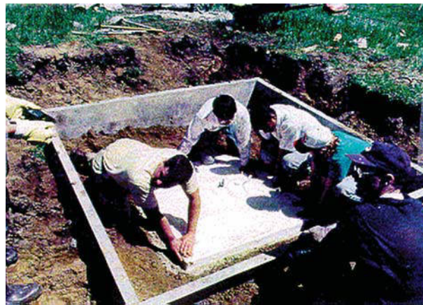
Figure 7.45 Sealed double-ring infiltrometer. (Courtesy of Professor Xiaodong Wang, University of Wisconsin, USA.)
