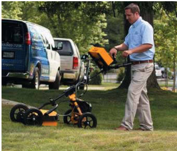
Figure 8.18 GPR testing and results. (Courtesy of Dig Smart of Maine)
