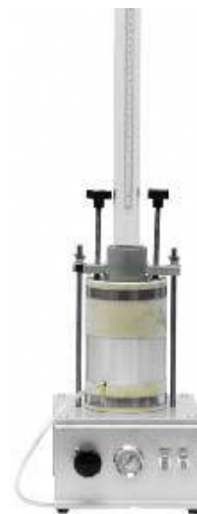
Figure 9.73 Falling head permeameter equipment: (a) Principle. (b) Equipment. (a: After FHWA. b: Courtesy of Gilson Company, Inc.)
