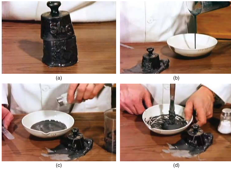
Figure 13.10 Rissa landslide clay, Norway 1978: (a) Intact quick clay. (b) Remolded clay. (c) Adding salt to remolded clay. (d) Remolded clay strengthened by salt. (Pictures/images are from the film The Quick Clay Landslide in Rissa, Norway , Made by Norwegian Geotechnical Institute [NGI])
