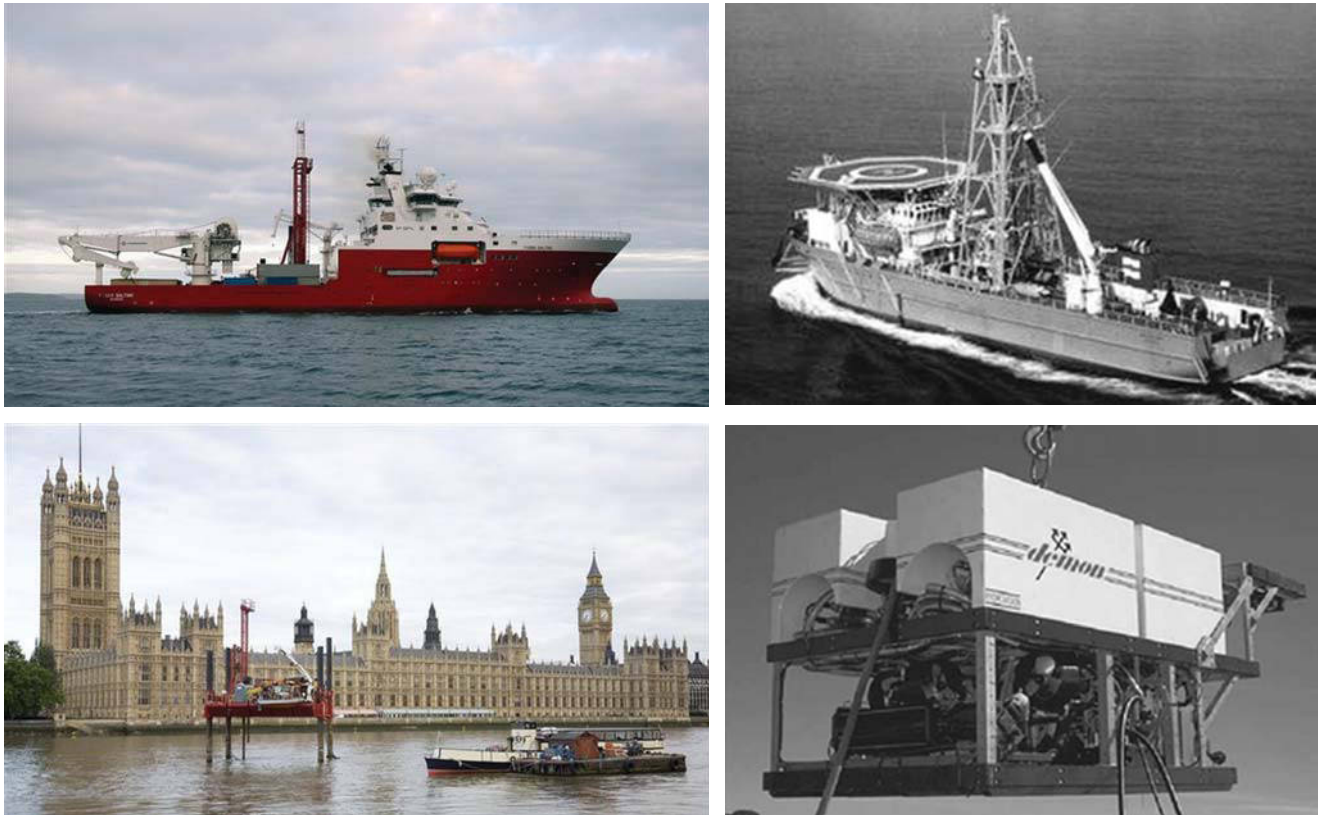
Figure 6.17 Ships, jack-up rig, and remotely operated vehicle (ROV) for offshore investigations. (a, and c: Courtesy of FUGROSeacore., b and d: Courtesy of the ISSMGE Technical Committee on Offshore Geotechnics)
