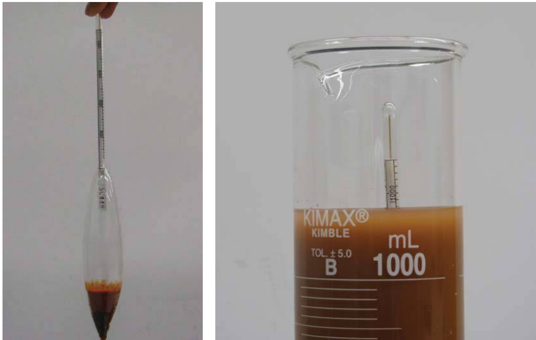
Figure 4.5 Hydrometer and hydrometer reading.
