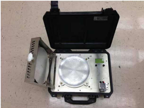
Figure 7.34 Field oven test (FOT) for water content.
