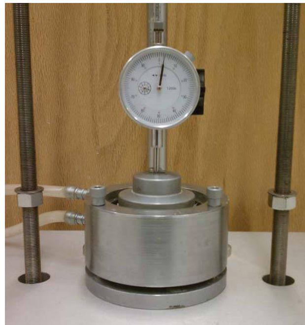
Figure 4.13 Free swell test for swell limit of undisturbed sample.
