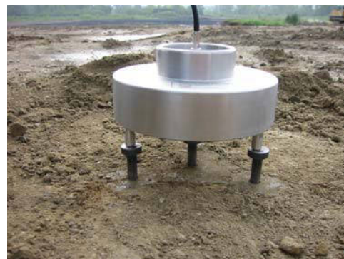
Figure 8.20 Example of time domain reflectometry field probe. (Courtesy of Professor Vincent Drnevich, Purdue University)
