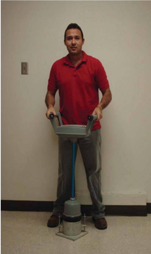
Figure 20.6 BCD-Proctor laboratory compaction test for modulus determination.
