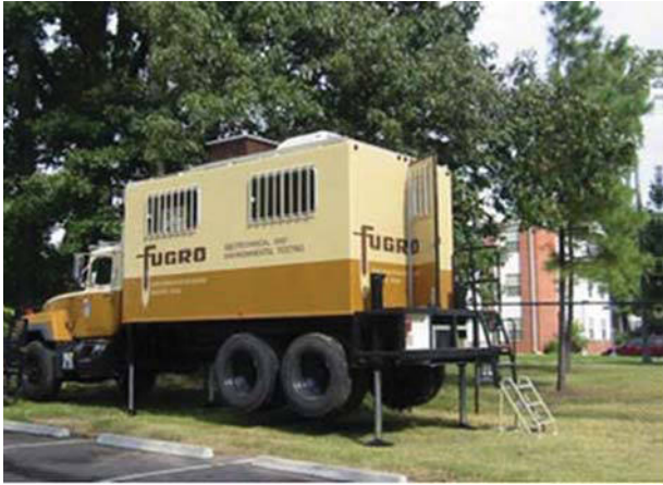
Figure 7.6 Cone penetrometer truck. (From Mayne 2007a. Courtesy of Professor Paul Mayne, Georgia Institute of Technology.)
