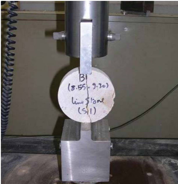
Figure 5.13 Brazilian tension test on Pointe du Hoc limestone.
