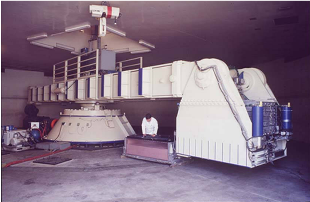
Figure 11.47 Geotechnical centrifuge. (Courtesy of the Center for Geotechnical Modeling, University of California-Davis, USA.)
