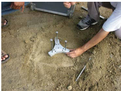
Figure 8.20 Example of time domain reflectometry field probe. (Courtesy of Professor Vincent Drnevich, Purdue University)
