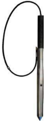
Figure 24.4 LED-induced fluorescence cone penetrometer probe. (Courtesy of Vertek, A Division of Applied Research Associates, Inc.)
