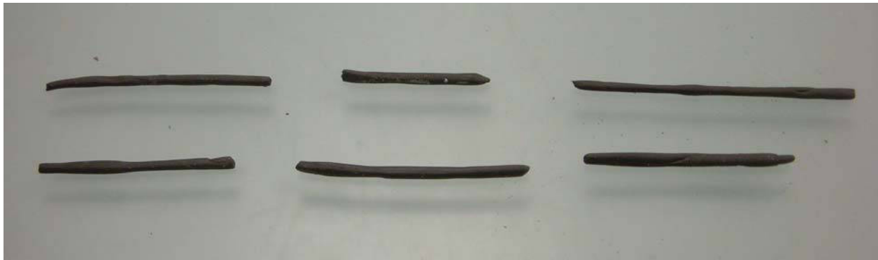
Figure 4.10 Plastic limit test and soil threads.
