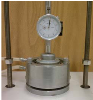
Figure 9.33 Swell test equipment.
