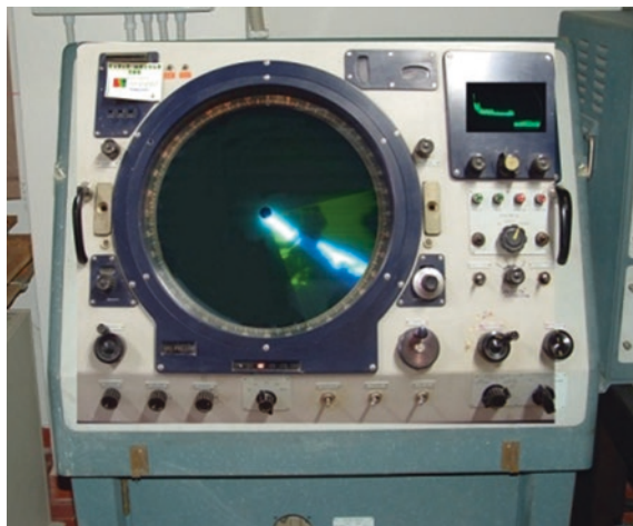
Fig. 10.2 Console of the meteorological radar meteor 200 mod. RMT 1S-2S (1961)
