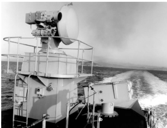
Fig. 7.25 The monopulse, coherent Fire Control naval radar RTN 30 X
