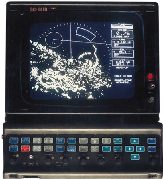
Fig. 7.54 The BX-132/732/1048 scan converter radar system with circular CRT (1985)
