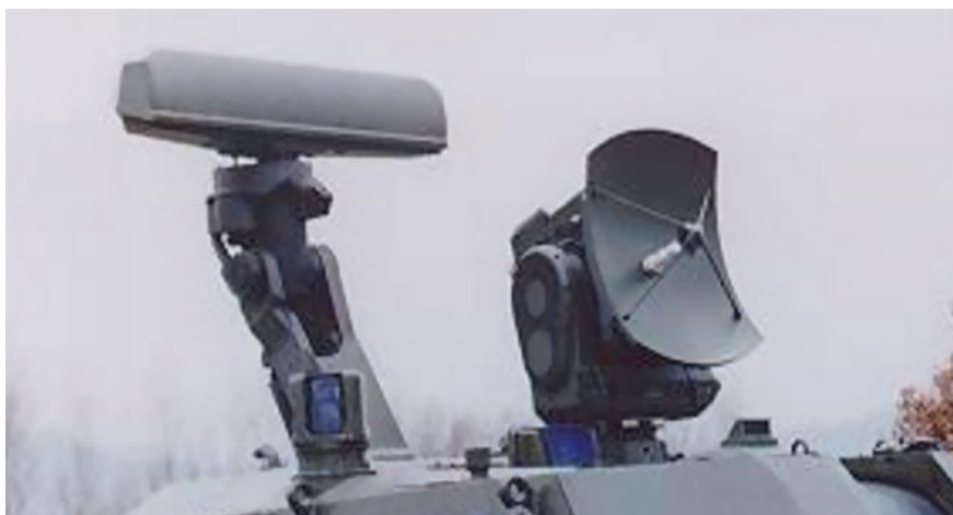
Fig. 7.9 Selex Galileo (SMA), 1980s: radars in S-band (search) and in K_a band (fire control) for the Otomatic tank
