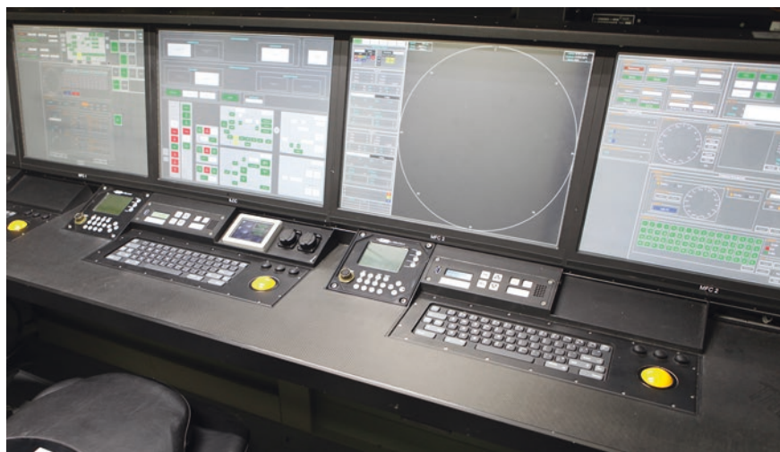
Fig. 10.3 The new console (2010s) of the kronos defense radar
