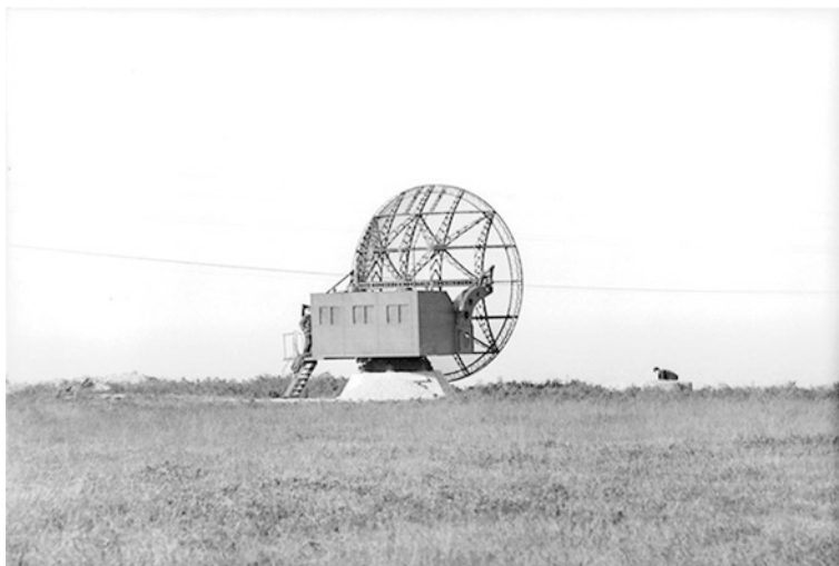
Fig. 5.4 The radar FuMG 65 “Würzburg-Riese“ (Giant Würzburg) with its parabolic reflector of 7.5 m in diameter
