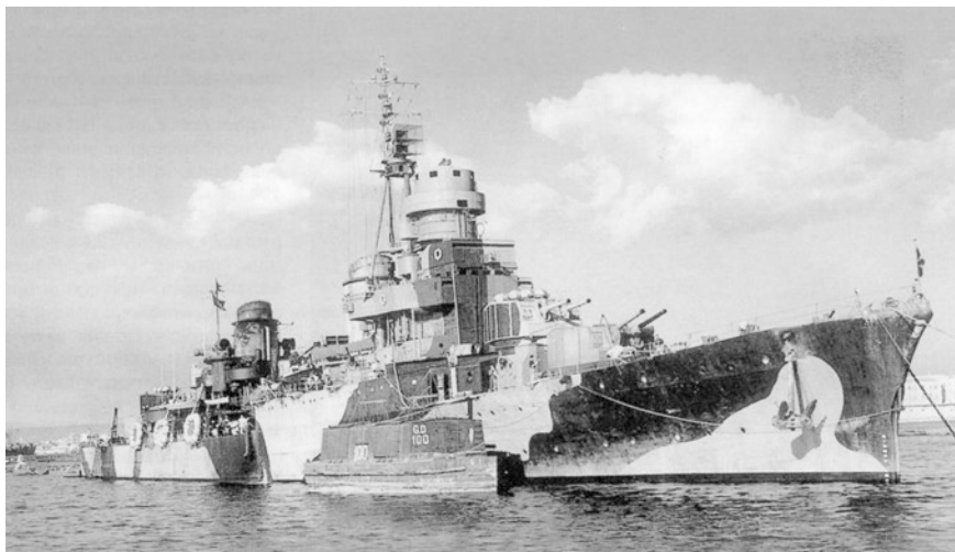
Fig. 2.36 The Cruiser Scipione Africano with the radar Gufo (October 1943)
