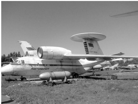
Fig. 6.35 The aircraft An-71 AWACS at the Aviation museum, Kiev. Features (from the display panel): two turbojet engines with 7500 kg of thrust each, maximum take-off weight 32 tons, cruising speed 530 km/h (maximum speed, 650 km/h), maximum height 10,800 m, up to 5 h endurance, 6 members crew, radar coverage: 360° in azimuth, from 0 to 30 km in altitude, up to 370 km in range. Photo by the author
