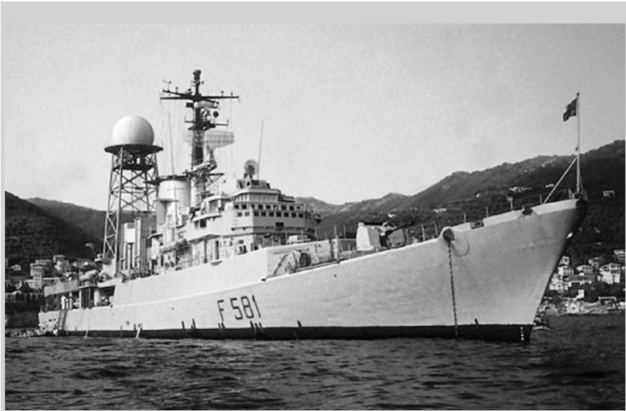
Fig. 7.37 The Carabiniere with the MFR-1C/EMPAR radar installed for tests
