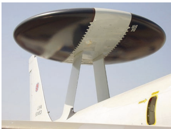
Fig. 6.33 Radome of the antenna of its AN/APY-1/2 radar, diameter 9.1 m, maximum thickness 1.8 m, rotation rate 6 rpm
