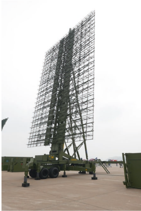
Fig. 9.2 The VHF AESA radar JY-27 A, developed in China (From: Aviation Week and Space Technology, Nov. 17, 2014, pp. 38–39, Courtesy of the Publisher)
