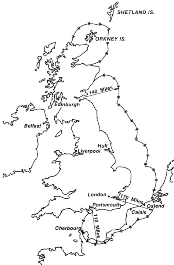
Fig. 4.5 The chain home coverage at the height of 5 km at the beginning of the Second World War
