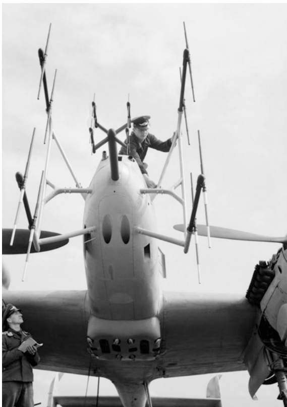
Fig. 6.16 The SN2 airborne interception radar on board a Messerschmitt Bf 110G night fighter at Grove, Denmark, August 1945
