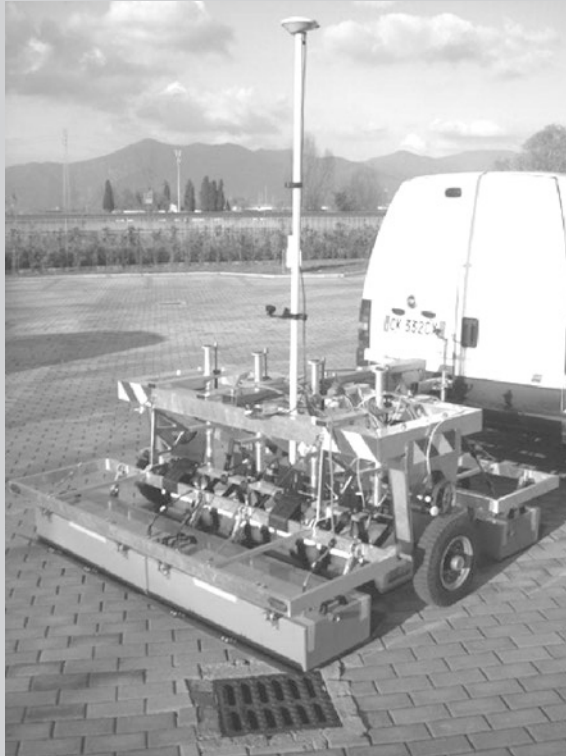
Fig. 7.32 Multi-antenna ground probing radar GPR (2009) model Stream Street by IDS
