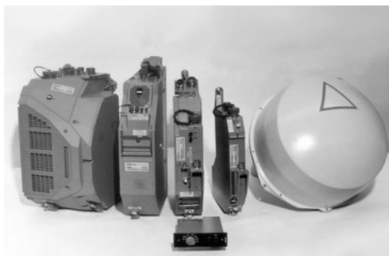
Fig. 7.8 Selex Galileo (SMA), 1980s: multimode airborne radar SCP-01 developed in cooperation with the Brazilian Air Force
