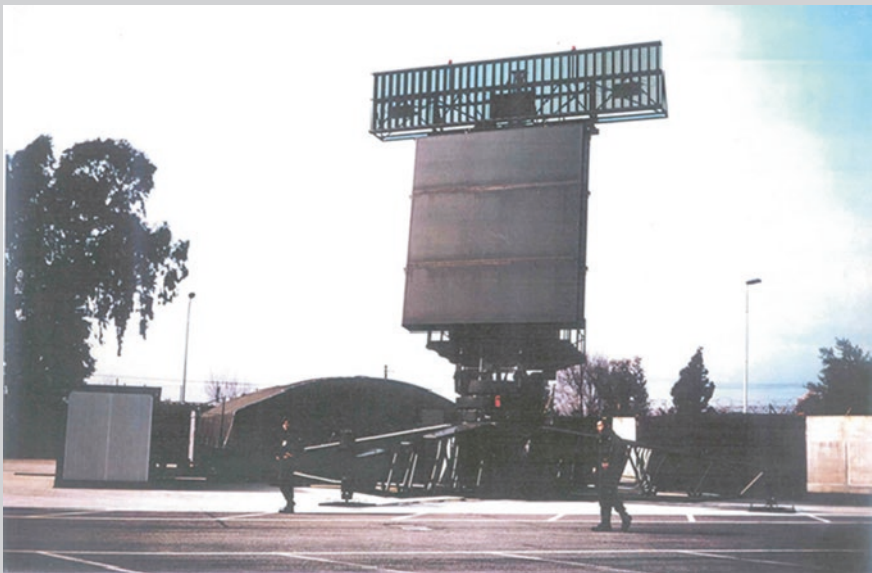
Fig. 7.33 The Selenia 3D radar (the S-band multi-beam antenna of the 3D radar has a co-rotating L-band, open-array IFF antenna on its top )
