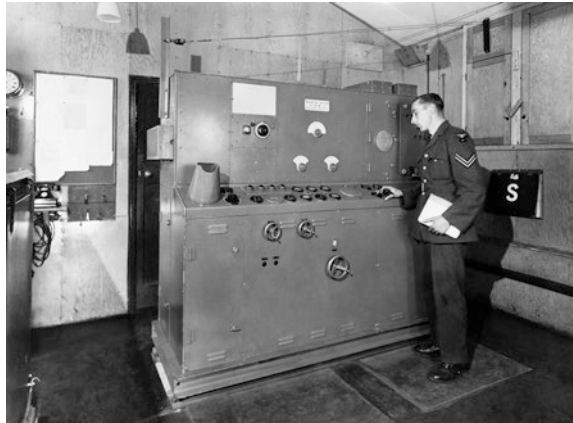
Fig. 4.7 Chain home low: the interior of a transmitter room at a CHL station. A corporal checks the settings on a Metro Vick Type T3026 transmitter
