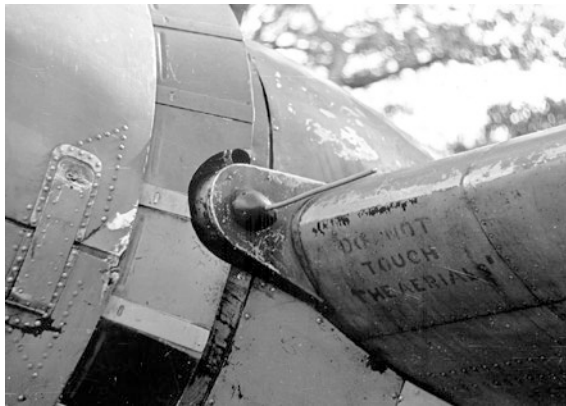
Fig. 6.6 Azimuth monopole of the Blenheim fighter I f
