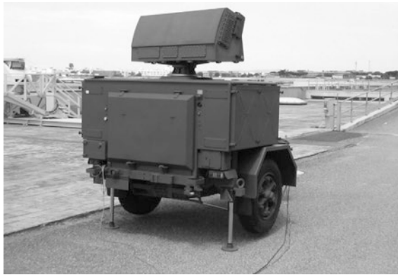
Fig. 7.52 The three-dimensional surveillance radar X-TAR 3D
