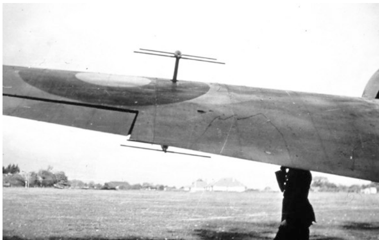
Fig. 6.7 Elevation dipoles of the Blenheim fighter I f
