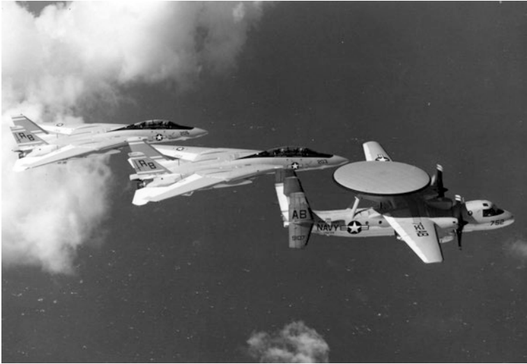
Fig. 6.31 Grumman’s twin turboprop W2F/E-2 Hawkeye ( right ) replaced the E-1B tracer as a carrier all-weather/AEW platform
