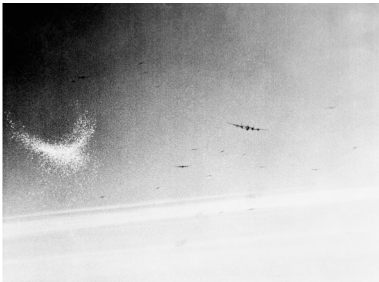
Fig. 5.9 A Royal Air Force Avro Lancaster bomber over Essen dropping “Window” (the white cloud on the left ) to interfere with ground gunners during a bombers raid on the city
