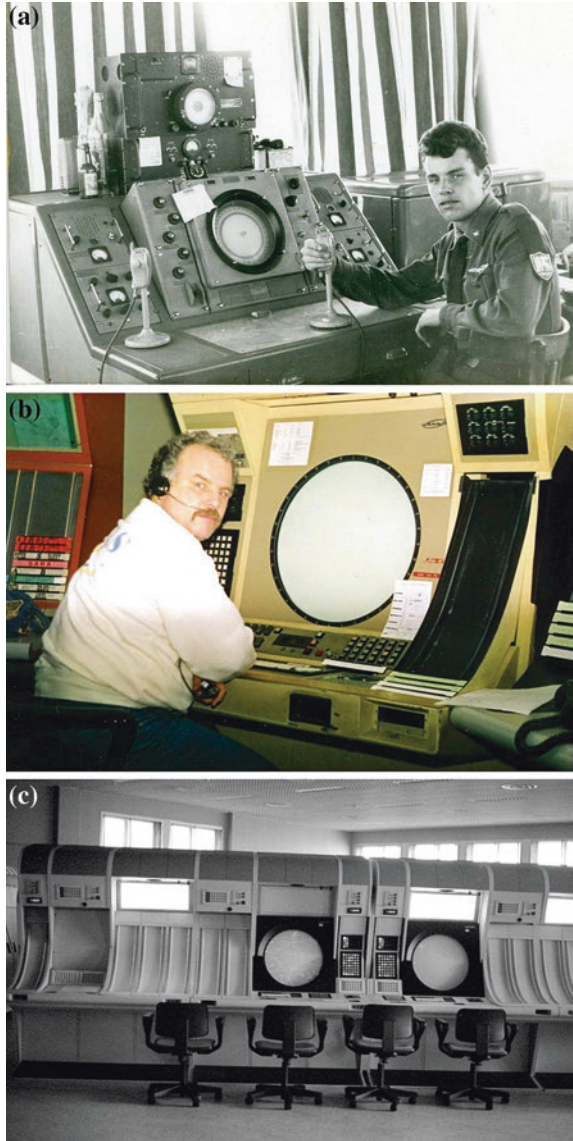
Fig. 5.26 a August 1963: the 18-years-old Franco Iosa, Tower Controller of the Italian Air Force, in the control tower of the military airport in Istrana (Treviso, Italy, ICAO code LIPS), with two radio goniometers, in UHF and (bottom) in VHF. b End of 1980s: the radar controller Franco Iosa in front of a Selenia DDS 80 console in the Area Control Centre (ACC) in Abano/Padova (Italy). c Beginning of 1990s: partial view of the renewed radar room in the Abano/Padova ACC just before the official opening
