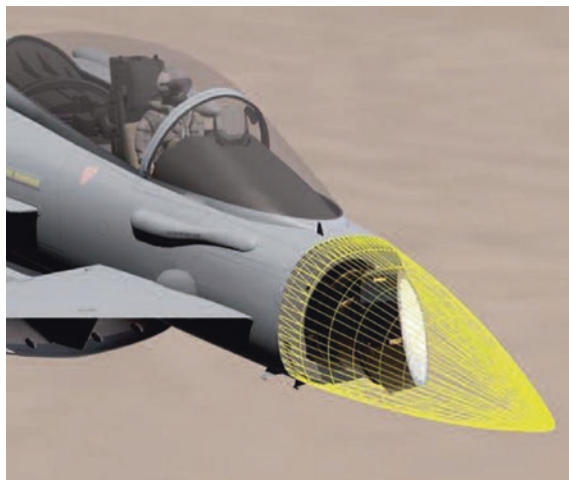
Fig. 6.39 The CAPTOR-E antenna on the Typhoon, with the repositioner shown
