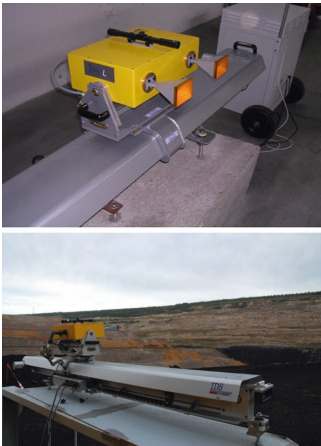
Fig. 7.58 The IBIS, Synthetic Aperture Interferometric radar in the K_u band, by IDS
