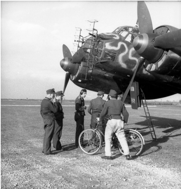
Fig. 6.17 A Junkers Ju 88G with the “ Hohentwiel ” radar
