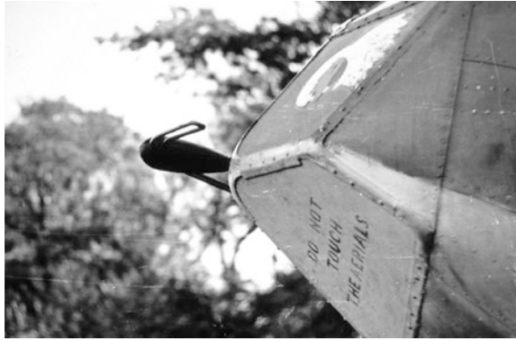
Fig. 6.5 Transmitting antenna of the Blenheim fighter I f
