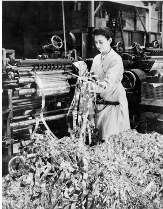
Fig. 5.8 A factory worker producing code-named “Window” (Chaff) foil which was dropped by allied aircraft to jam enemy radar
