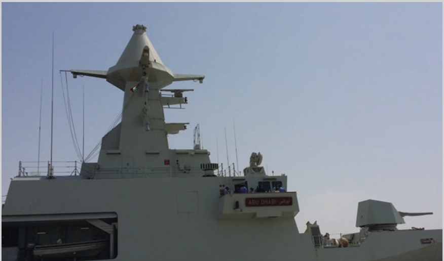
Fig. 7.41 The Kronos naval radar under radome and the RTN-30 X (directing the OTO-Melara 76 mm gun—on the right side ) on board of the anti-submarine warfare ASW vessel ABU DHABI class—Overall length 88.40 m, full load displacement 1650 tons— Courtesy Etihad Ship Building (ABU DHABI, March 2015)
