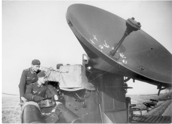
Fig. 5.3 The German FuMG 62D “Würzburg” radar, the first radar with sufficient precision to allow batteries to hit an air target in the absence of optical visibility
