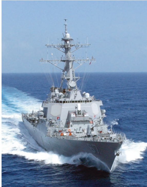
Fig. 9.18 The destroyer USS Cole (DDG-67), Arleigh Burke class: two of the four faces of the antenna of the AN/SPY-1 can be seen. The ship is known to have suffered the terrorist attack on October 12th, 2000 in the port of Aden, with 17 casualties among the crew
