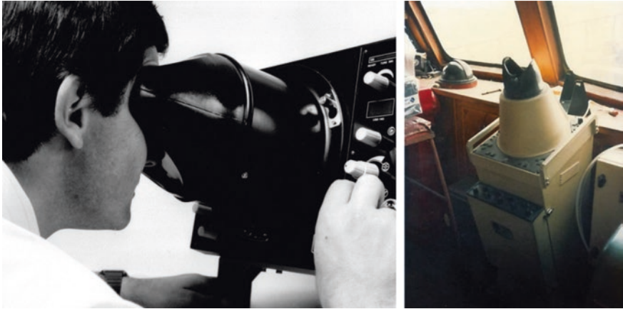
Fig. 7.54 The BX-132/732/1048 scan converter radar system with circular CRT (1985)
