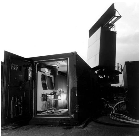
Fig. 7.26 The ground-based, 3D long-range, S-band radar RAT 31 SL
