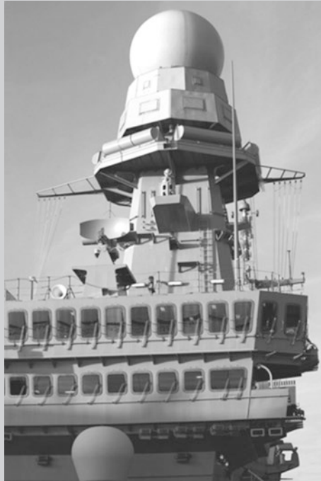
Fig. 7.38 The EMPAR installed on board the aircraft carrier Cavour
