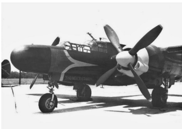
Fig. 6.22 The SCR 720 on the Northrop P61. This set operated on the 10 cm wave, had a 74 cm dish antenna with a main lobe of 10^\circ . The feeder of the antenna was spinning at 360 or 100 rpm. 0.75 \mu\text{s} long pulses were transmitted with a pulse repetition frequency (PRF) of 1500 Hz and a peak power of 3 kW. Range on bombers at 3000 m: 16 km, on fighters: 8 km
