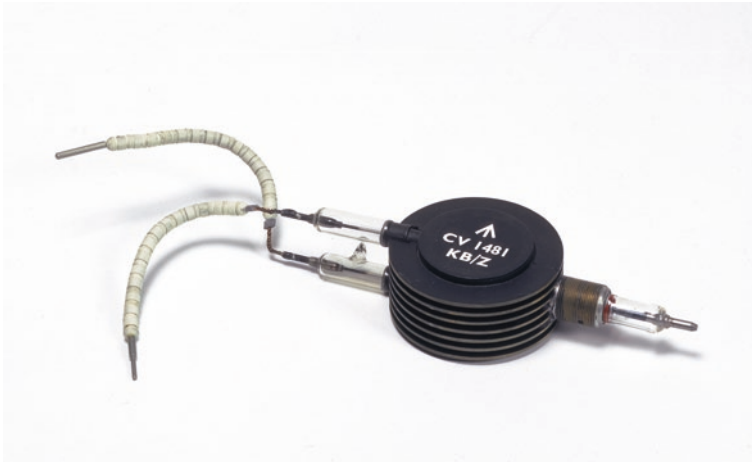
Fig. 5.15 British Magnetron CV1481 (improved version of CV76C ). Nominal frequency 2993 MHz, peak output 450 kW at PRF = 500 Hz, pulse length from 0.7 to 2 \mu s
