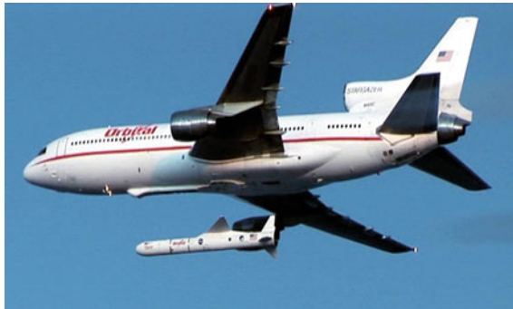
Fig. 3.2 Orbital Sciences employs a modified L-1011 commercial jet to carry its air-launched Pegasus rocket to send commercial and government payloads to low-Earth orbit (image courtesy of NASA/JPL, used with permission)
