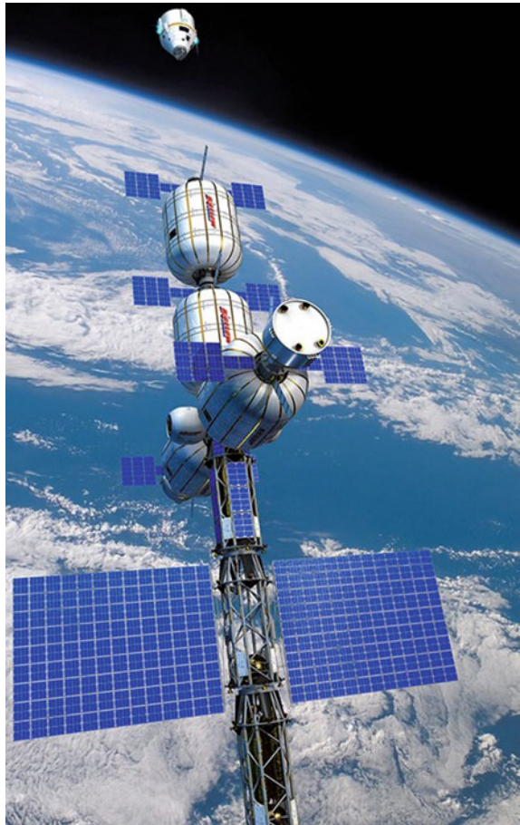
Fig. 6.5 Four Bigelow BA-330 expandable modules are shown as part of a space station, with a Boeing capsule approaching to dock (image courtesy of Bigelow Aerospace, used with permission)
