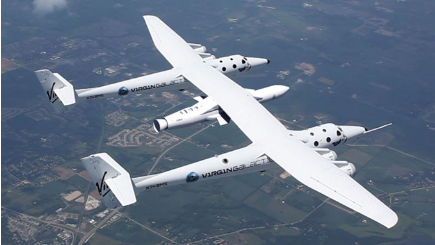
Fig. 3.5 Virgin Galactic uses the same carrier aircraft for its SpaceShipTwo and LauncherOne commercial satellite payloads (image courtesy of Virgin Galactic, used with permission)
