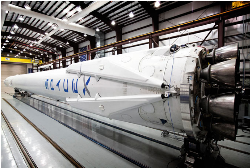
Fig. 2.2 The upgraded Falcon 9 booster features longer propellant tanks and deployable landing legs to permit reusability of the booster (image courtesy of SpaceX, used with permission)
