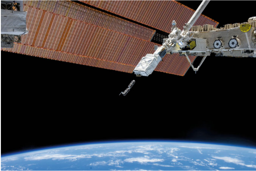
Fig. 5.2 Two cubesats are deployed from the International Space Station by the NanoRacks cubesat deployer on February 11, 2014 (image courtesy of NASA, used with permission)
