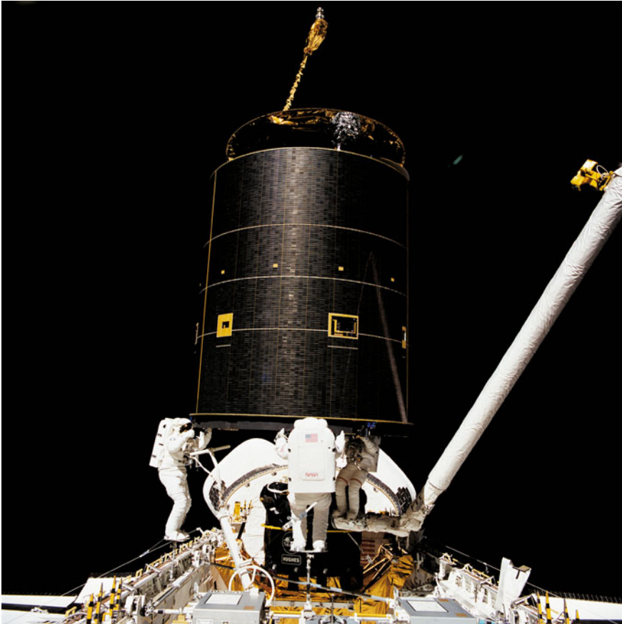
Fig. 1.1 NASA astronauts performed many commercial missions during the space shuttle era. Three astronauts are shown installing a replacement Orbus-21S motor on the Intelsat 603 satellite during mission STS-49 in March 1990 (image courtesy of NASA)
