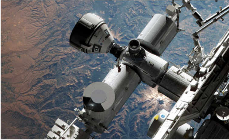
Fig. 4.4 The Boeing CST-100 crew capsule with service module is shown docked to the International Space Station. Boeing plans to include private spaceflight participants on select missions (illustration courtesy of Nathan Koga/NASASPACEFLIGHT.COM, used with permission)
