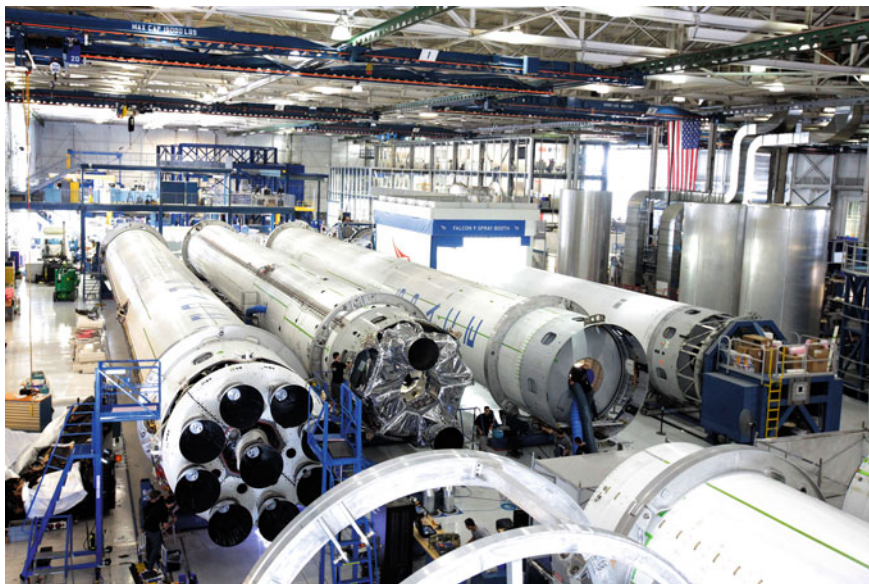
Fig. 2.1 SpaceX Falcon 9 boosters being assembled at the company’s headquarters in Hawthorne, California (image courtesy of SpaceX, used with permission)
