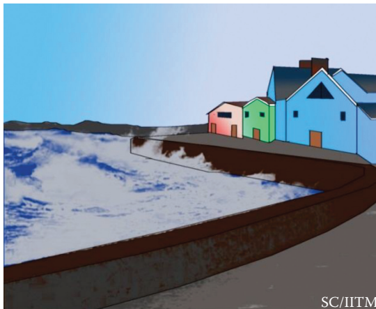
FIGURE 1.71 Seawalls protect houses along the coastal line.
