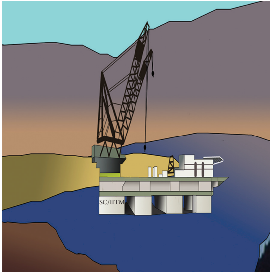
FIGURE 4.26 Heavy-duty crane SSCV Thialf.
