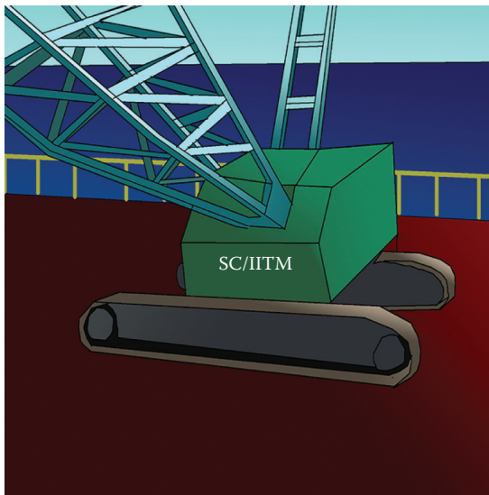
FIGURE 4.27 Crane barge used in upending and erection.
