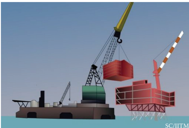
FIGURE 4.19 Deck mating of a jacket platform.
