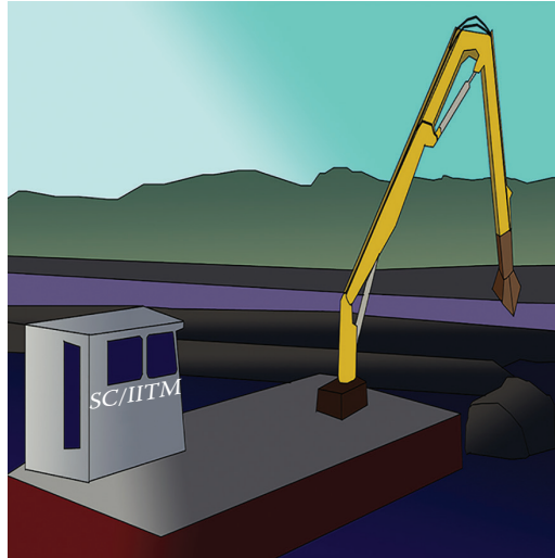
FIGURE 4.64 Dredger in operation: sideline dredging from the pontoon.
