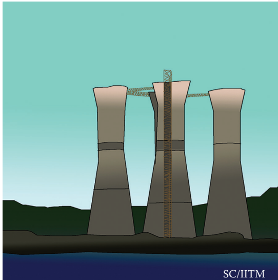
FIGURE 4.16 Towing the tower to the installation site.
