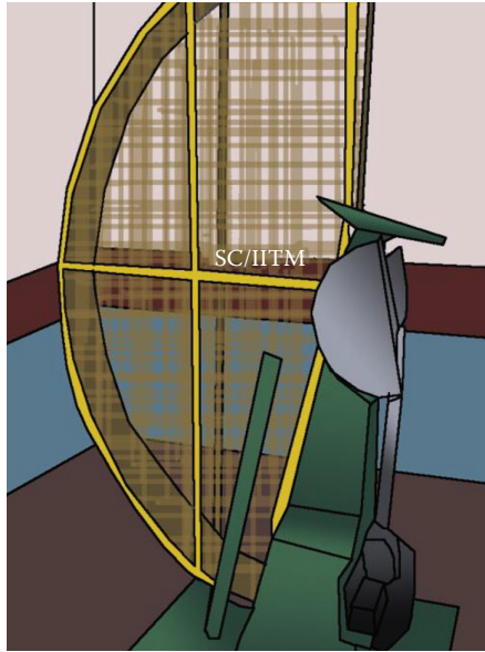
FIGURE 3.4 Schematic view of a Charpy test setup.
