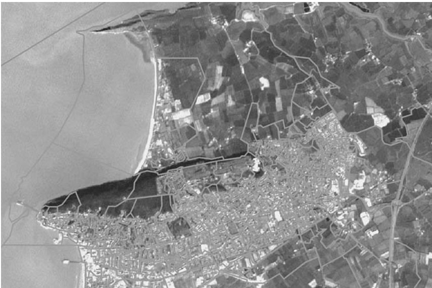
Figure 4.10 By using a GIS to overlay the boundaries of 2001 UK Census output areas onto a remotely sensed image of a coastal region it can be seen that not all the Census OAs are uniformly populated
