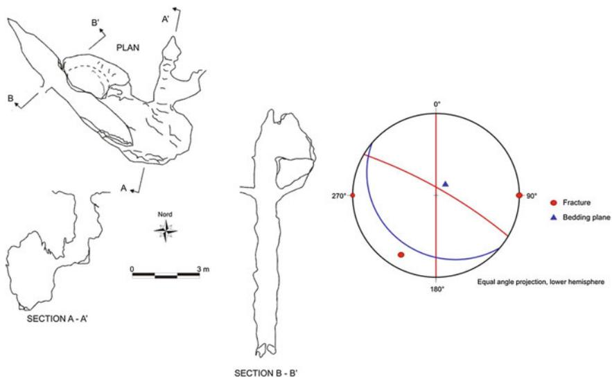
**Fig. 6.241** Map and stereogram of main geological structures
