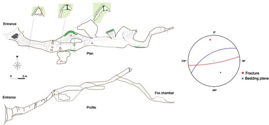
Fig. 6.295 Map and stereogram of the main geological structures in cave
