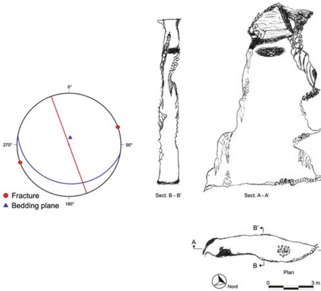
**Fig. 6.204** Map of “Zubbia della Bella Addormentata” and stereogram of the main geological structures in cave
