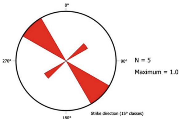
**Fig. 6.199** General Rose diagram of main karstification geological structures in the Piano Zubbia-Mt. Bufara area
