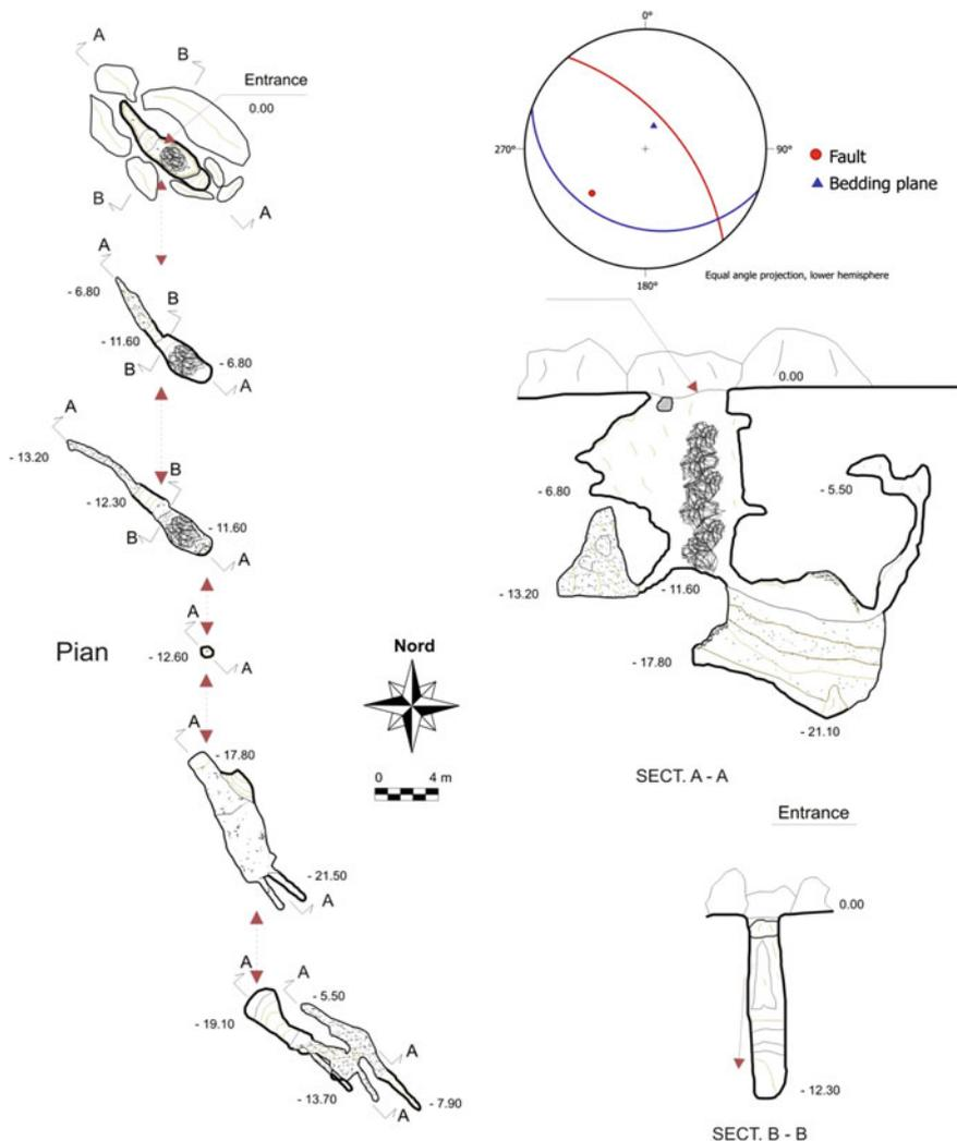
**Fig. 6.210** Map of “Zubbia su Filu Ferru” and stereogram of the main geological structures in cave
