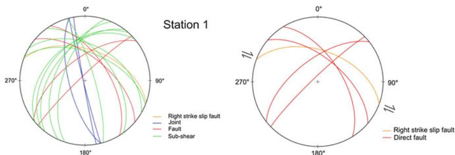
**Fig. 7.16** Stereograms with projection of normal faults (*red*) and right strike slip faults (*yellow*). Station 1 in a quarry in the western foothill sector of Mt. Palatimone
