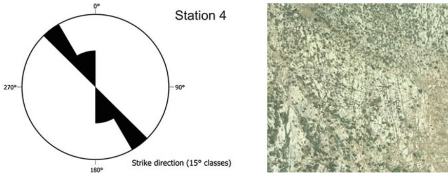
**Figs. 7.21–22** Rose diagram of surface crevasses located in the pediment of the central area of Mt. Palatimone. To the *right* side orthophoto image of the area
