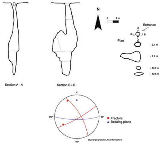
Fig. 6.260 Map and stereogram of the main geological structures in cave
