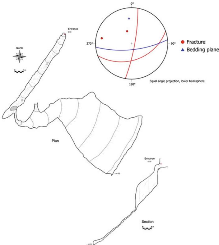
Fig. 6.256 Map and stereogram of the main geological structures in cave
