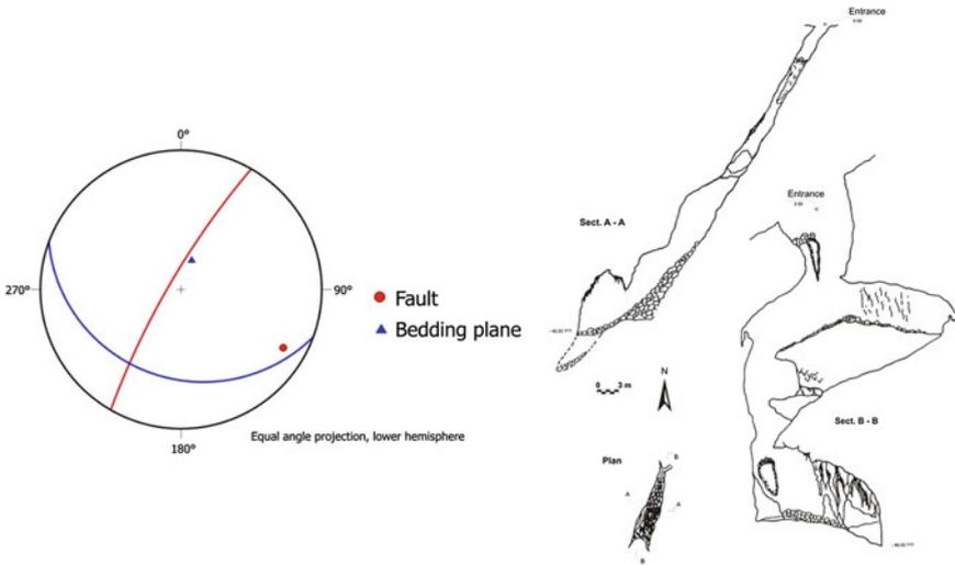
Fig. 6.225 Stereogram of the main geological structures and map of the cave
