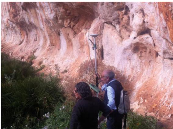
**Fig. 8.7** Survey for intersection by total station Leica TC 905/L of the sea cave Grotta dei Pendenti in the Monte Monaco
