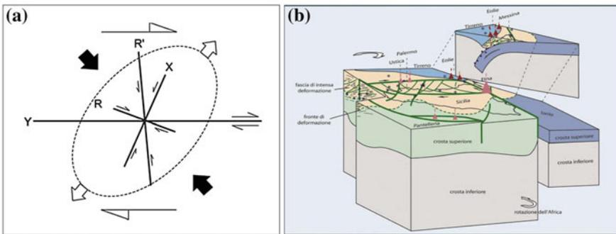
**Fig. 8.2** **a** Two-dimensional geometry of today stress field acting in northwestern Sicily, and structural interpretation of the structures mapped in the studied area (modified after Tondi et al. 2006); **b** 3D model of the Sicilian area showing the most important neotectonic fault system (green), the chain sectors (beige) and the undeformed areas (light grey) (modified after Napoli et al. 2012)
