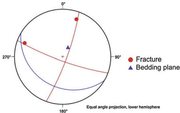
**Fig. 6.238** Stereogram of the main geological structures in cave
