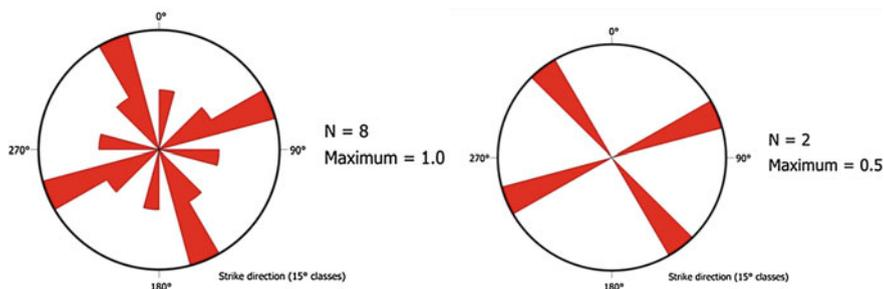
**Figs. 6.266–267** Rose diagram of the main karstified structures surveyed in the caves (*left side*) and of the main structures surveyed in tectonic caves (*right side*)
