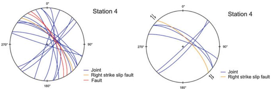
Figs. 7.5–6 Stereogram of data collected in Station 4 (left side); Stereogram with right strike strip fault (right side)
