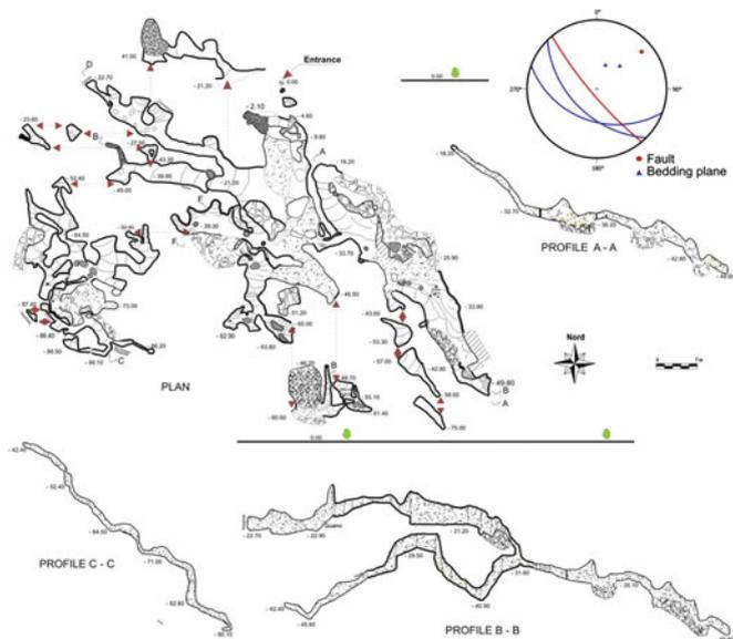
**Fig. 6.178** Map and stereogram of the main geological structures of Grotta Maria SS. di Customaci
