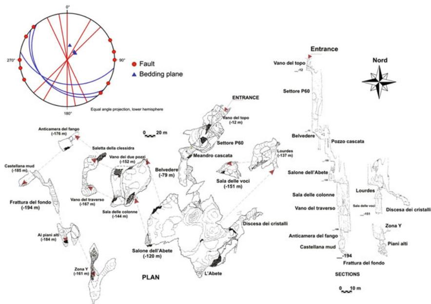
**Fig. 6.231** Map, sections and stereogram of the main geological structures of Abisso del Purgatorio
