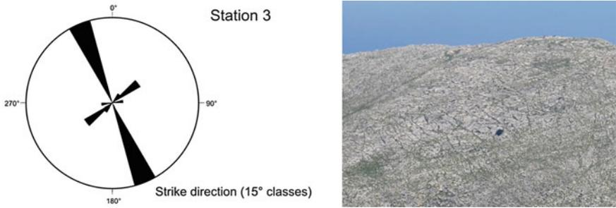
**Figs. 7.19–20** Rose diagram of surface large crevasses of the *upper* central part of the structural slope of Mt. Palatimone (data extracted from orthophotos image); on the *right* sector of Mt. Palatimone with crevasses
