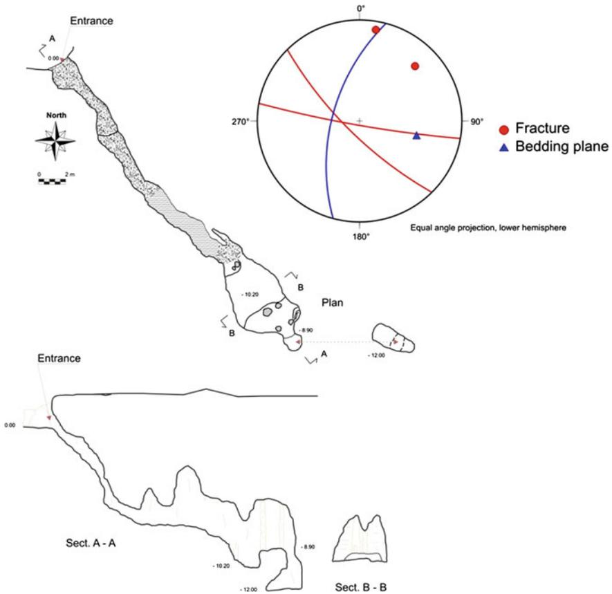
**Fig. 6.258** Map and stereogram of the main geological structures in cave
