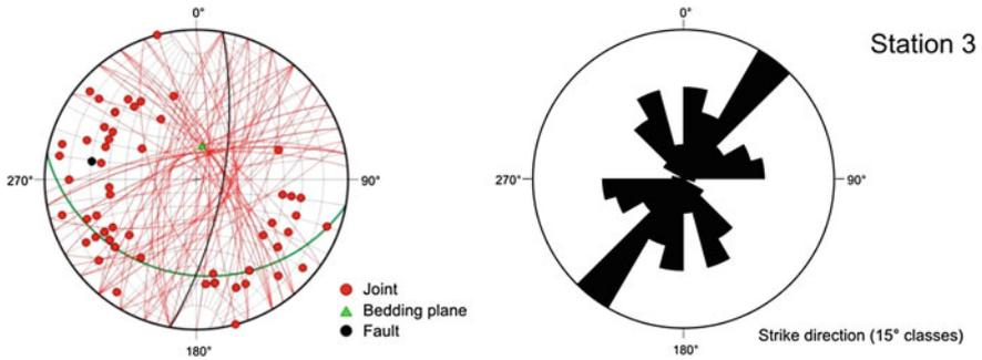
**Fig. 7.26** Stereogram and rose diagram of the structural survey of the eastern part of the polje (Station 3)
