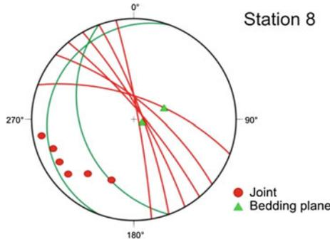
Fig. 7.12 Stereogram of the structures surveyed on the Station 8
