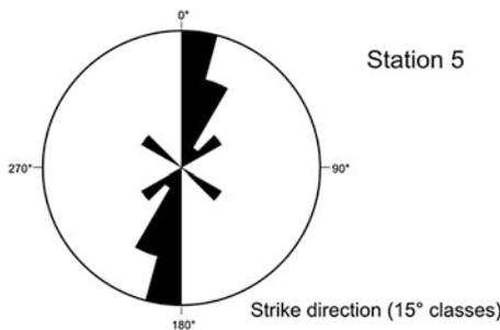
**Fig. 7.23** Rose diagram of the structural slope of the *upper* eastern ridge (data extracted from orthophoto image)
