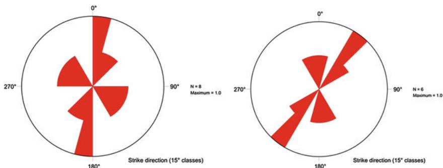
**Figs. 6.249–250** Rose diagram of the cave karstified geological structures of the central (*left side*) and eastern sector (*right side*) of the polje
