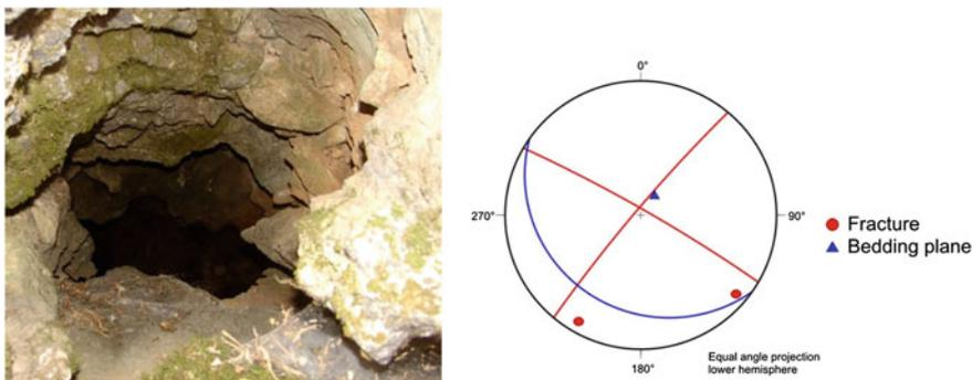
Fig. 6.223 Internal part of the shaft along a fracture with dip to N 30 at 85° and stereogram of the main geological structures in cave
