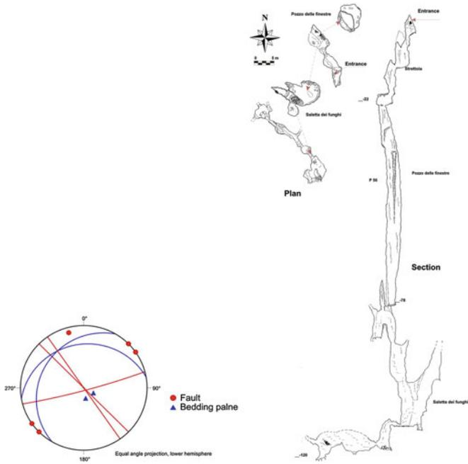
Fig. 6.246 Stereogram of the main geological structures and map of the cave
