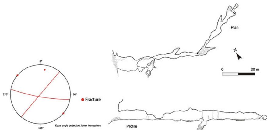
**Fig. 6.293** Map and stereogram of the main geological structures of the Grotta del Riccio
