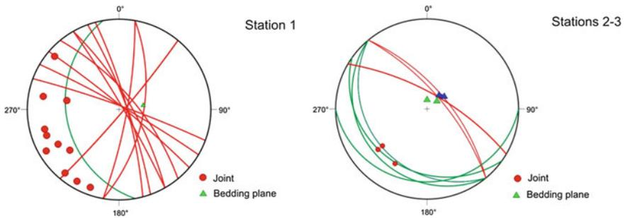
Fig. 7.4 Stereograms of structural data collected from Station 1 (left side) and Stations 2–3 (right side)
