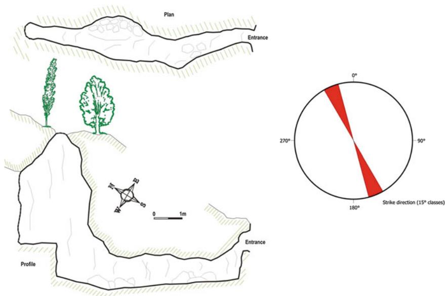
**Fig. 6.287** Map and Rose diagram of the main geological structures in cave
