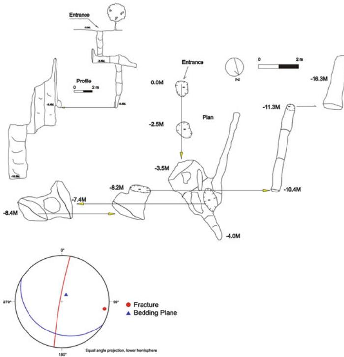
Fig. 6.243 Map and stereogram of the main geological structures in cave
