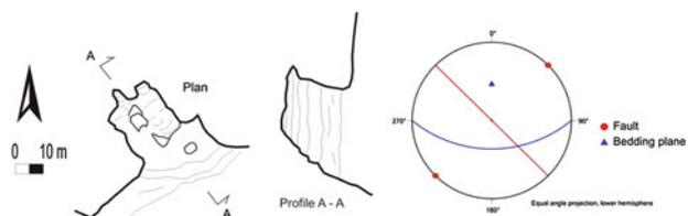
**Fig. 6.262** Map and stereogram of the main geological structures
