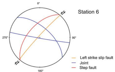
**Fig. 7.10** Slip surface of a fault located in the Station 6: the kinematic indicator suggests a *left*-lateral strike-slip motion for the NE-SW trending structure
