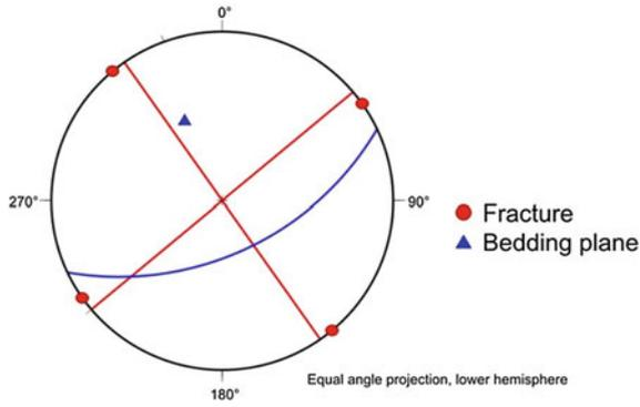
Fig. 6.252 Stereogram of the main geological structures in cave
