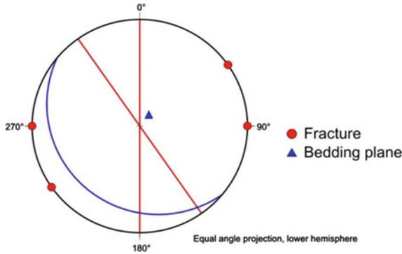
**Fig. 6.236** Stereogram of the main geological structures in cave
