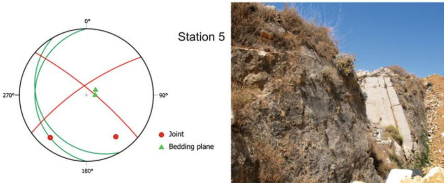
**Figs. 7.7–8** Stereogram of surveyed data in the sites of Station 5 (*left side*); Fault wall near Clava cave (*right photo*)
