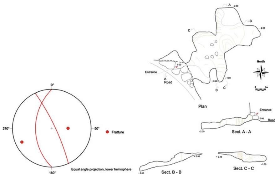
Fig. 6.254 Stereogram of the main geological structures and map of the cave
