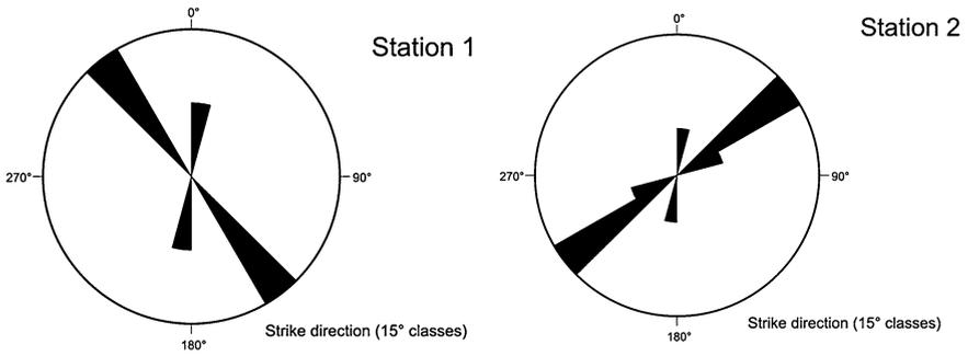
**Fig. 7.25** Rose diagram of the lineations from orthophotos image in the western (*left side*) and in the central part of the polje (*right side*)
