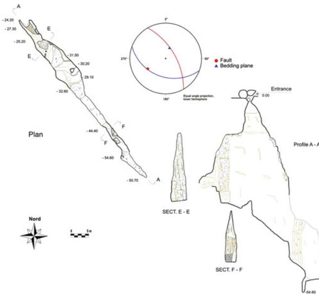
**Fig. 6.205** Map of the “Zubbia delle Meraviglie” and stereogram of main geological structures in cave
