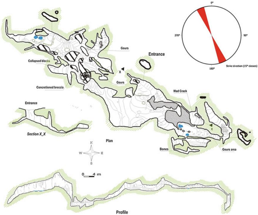
Fig. 6.269 Map of the cave and Rose diagram of the main geological structures
