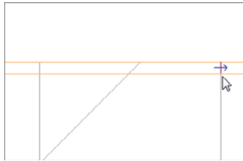
FIGURE 2.62 This line indicates where the wallboard will be cut. The blue arrow indicates the side of the material that will remain.
