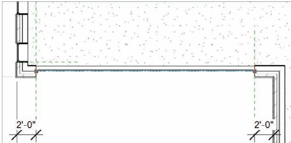
FIGURE 16.28 Drawing the curtain wall at the centerline of the wall between the two reference planes
