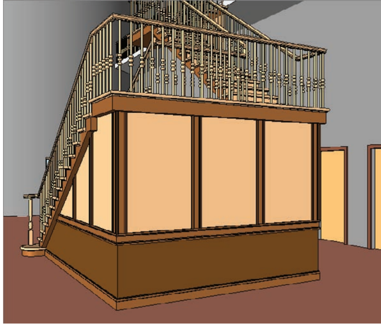
FIGURE 16.21 The final walls with the sweeps added
