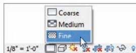
FIGURE 1.35 The detail level control allows you to set different view levels for the current view.
