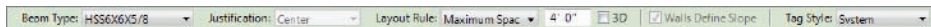
FIGURE 8.41 Setting the maximum spacing and the tag style on the Options bar.
