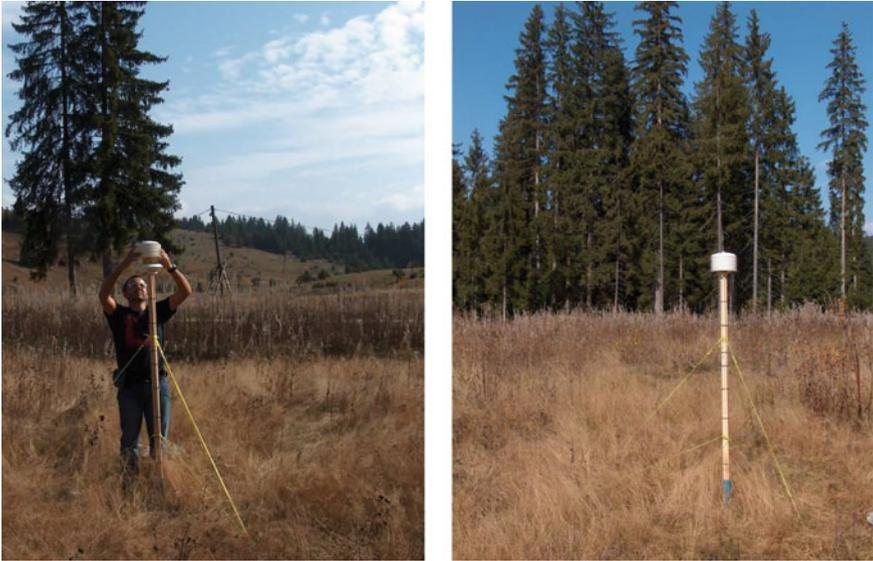
**Fig. 3.2** Mounting of the external temperature data logger. For location refer to Fig. 3.8
