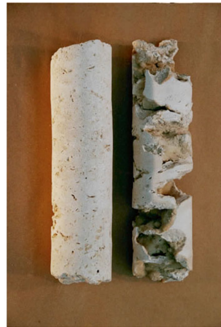
a Core from boring over Lake Surprise b Core from boring within the anomalous area
