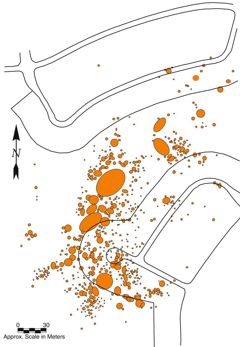
Fig. 7.4 A new housing development in west central Florida 760 sinkholes occurred within 24 h as a result of drilling and completing a well for irrigation purposes
