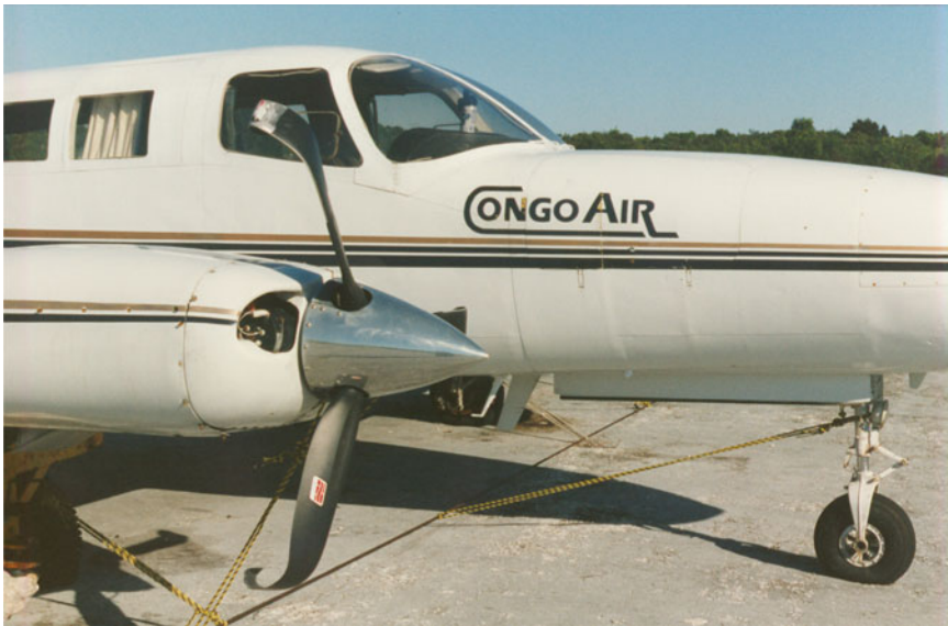
Fig. 7.3 Damage to an airplane propeller that encountered a small sinkhole (banana hole) on the runway at Congo Town airport, Andros, Island Bahamas
