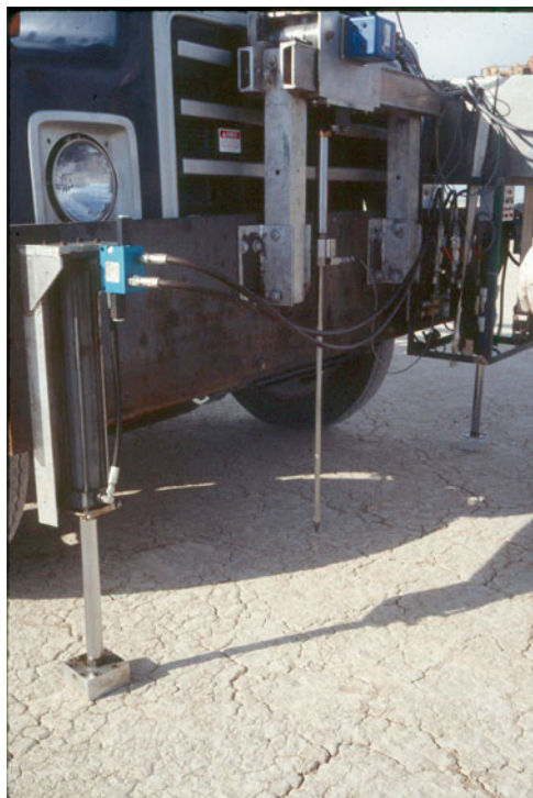
Fig. 17.8 Photo of the specialized shallow CPT system used to evaluate the fissures at Edwards Air Force Base (EAFB)
