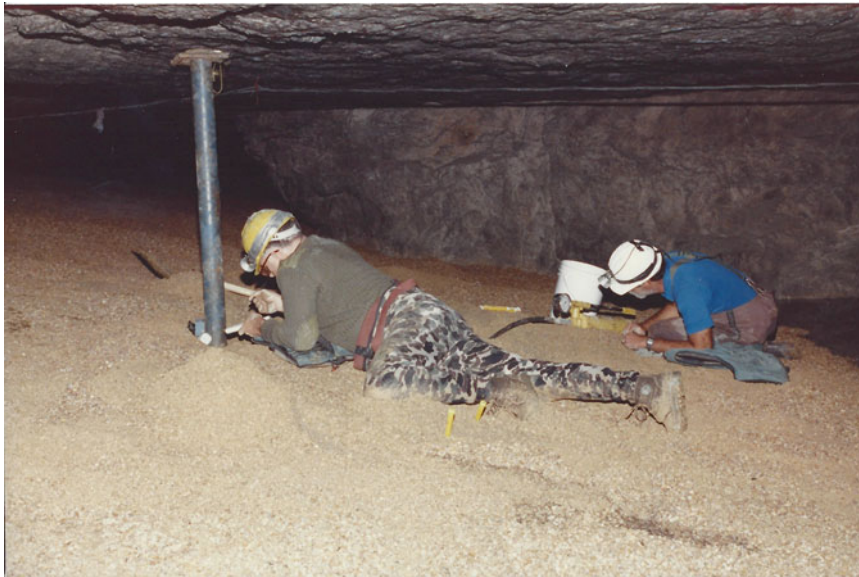
Fig. 25.24 In-situ compression tests were made on the crushed rock fill material
