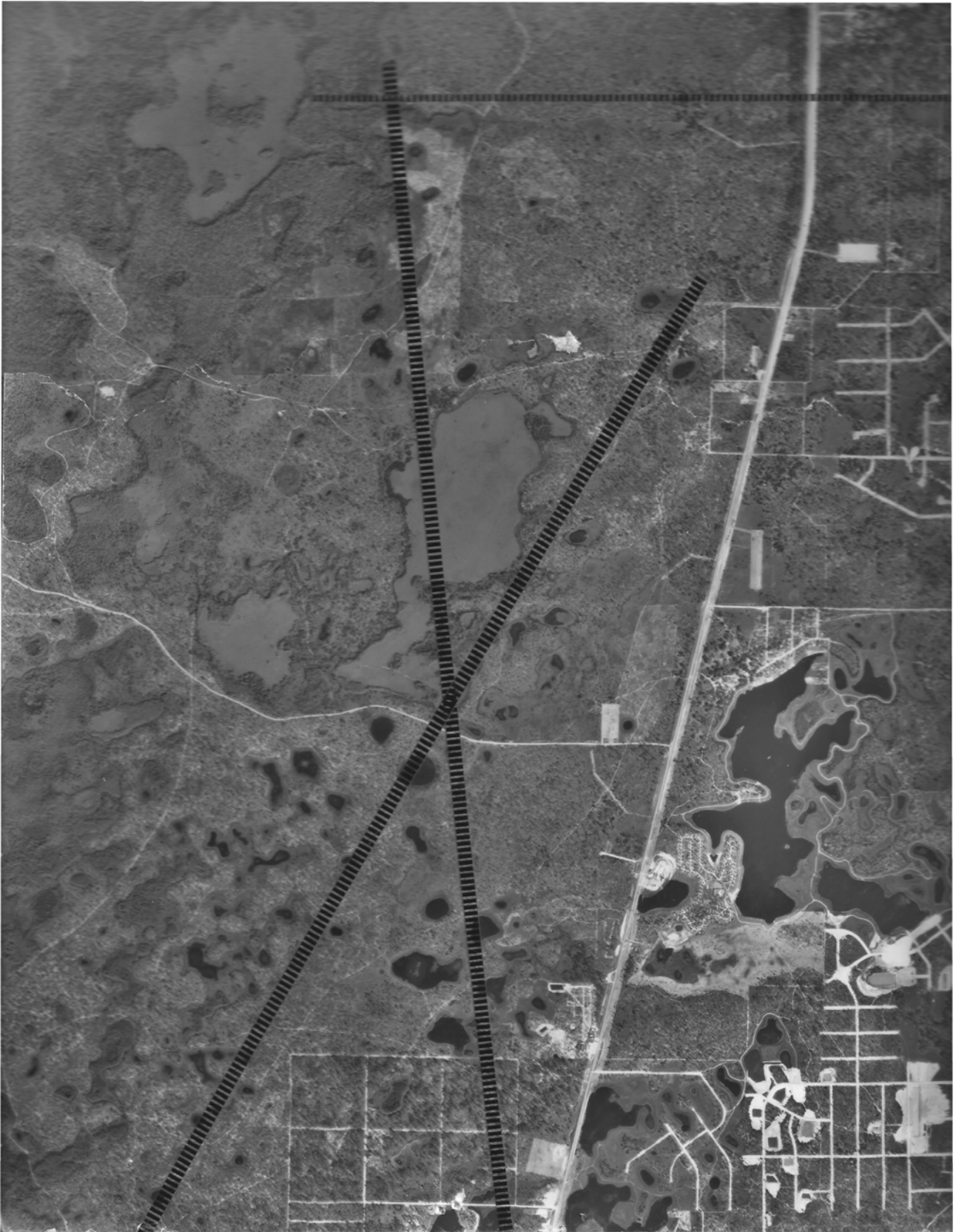
Fig. 14.5 Linear trends associated with in sinkholes along a portion US19 in west-central Florida
