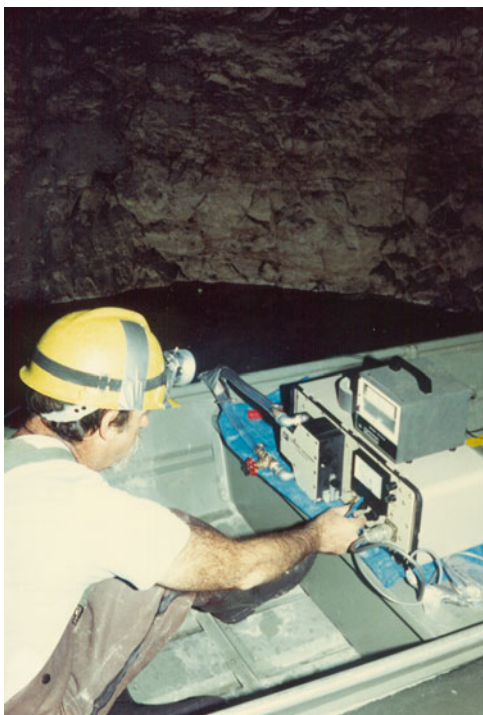
Fig. 22.5 A Turner fluorometer with water being continuously pumped through it to sample for the presence of any dye as the boat moves through the water within the Tobin mine. The results were recorded on a strip chart recorder
