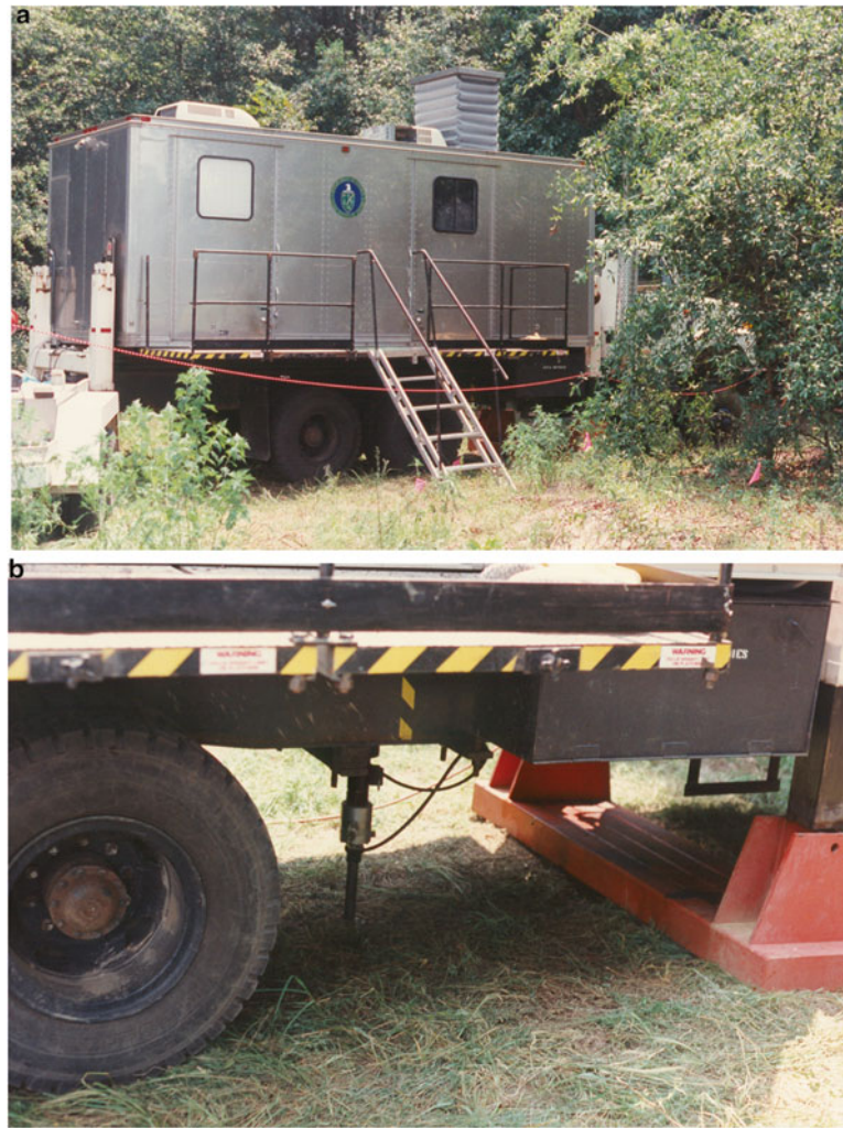
Fig. 17.5 A CPT rig is being used to evaluate soil conditions at a contaminated site in a karst setting (a) and a close-up of the probe beneath the truck (b)
