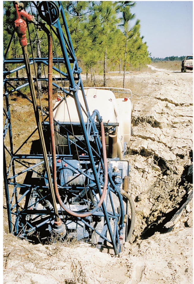
Fig. 8.2 The Guest Sinkhole in west central Florida triggered by drilling a monitor well (Tihansky 1999)
