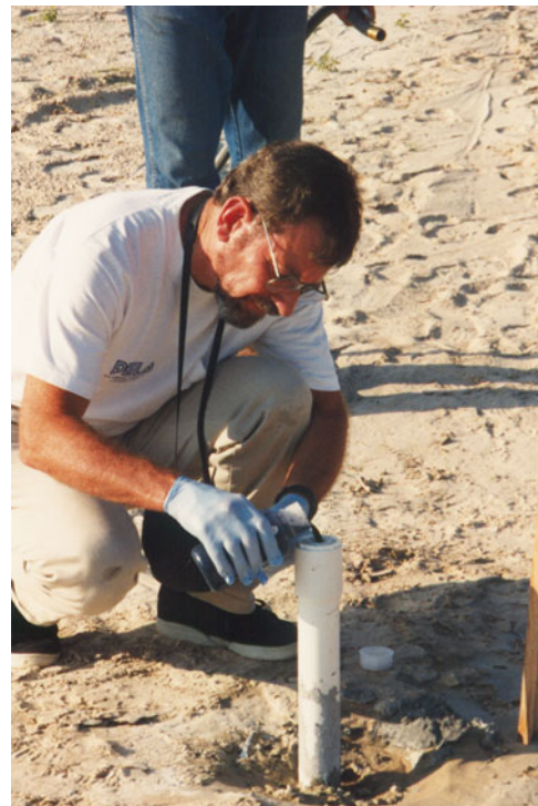
Fig. 22.2 Barry Beck introducing dye into a monitor well at a site in West Central Florida to determine its possible connection to a recent large sinkhole
