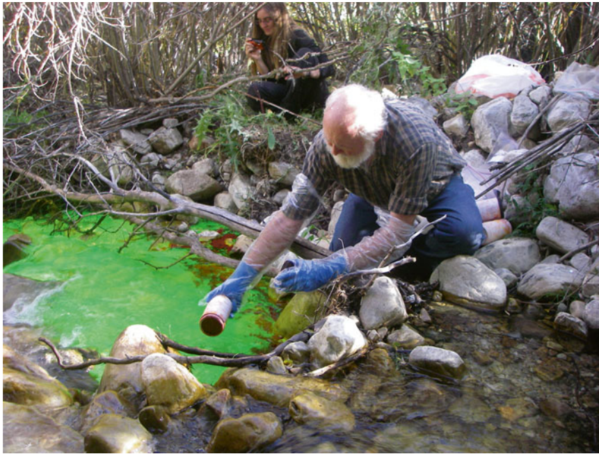
Fig. 22.1 Fluorescein dye being introduced by Tom Aley into a sinking stream in Nevada (Photo courtesy of T. Aley and G. Baker)
