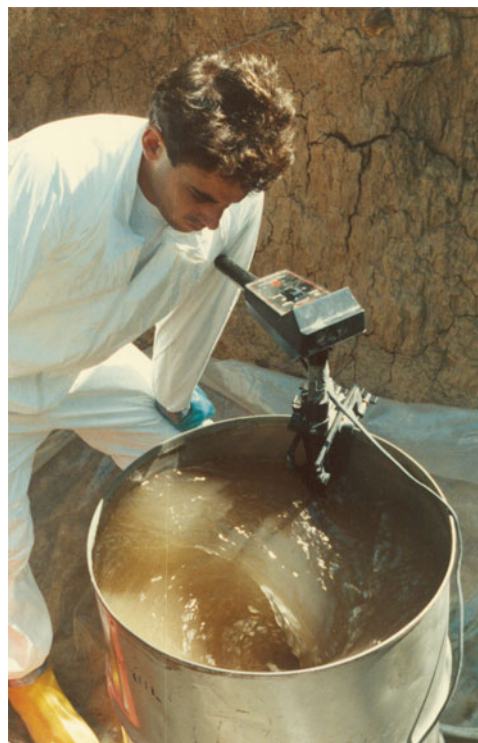
Fig. 22.4 Mixing of fluorescein dye prior to its introduction into a major fracture
