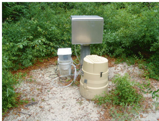
Fig. 22.7 An automated water sampler can be used to obtain discrete samples at programmable intervals
