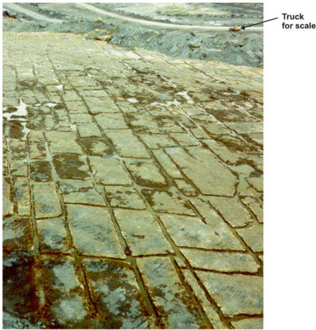
Fig. 15.4 The floor of the Missouri Portland Cement Quarry in Independence, Missouri reveals the extent and spacing of fractures in the Bethaney Falls Limestone
