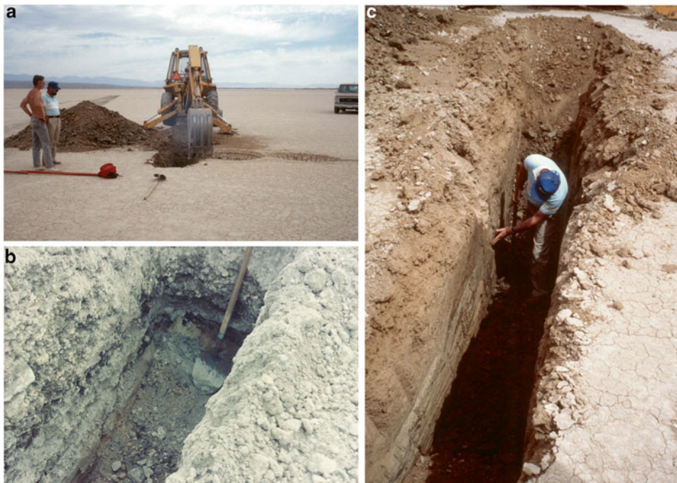
Fig. 17.21 Shallow trenches whether by backhoe (a and c) or dug by hand (b) can provide critical observations in the assessment of subsurface conditions
