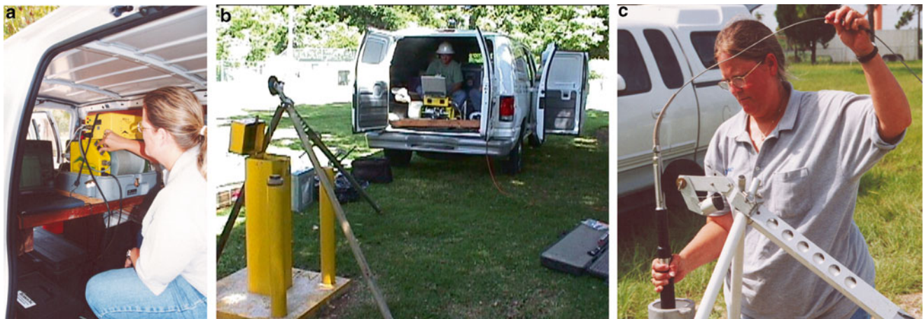
Fig. 18.2 Photos of typical logging system in operation. (a) Control unit, laptop and winch. (b) Tripod over well. (c) Probe being lowered into well
