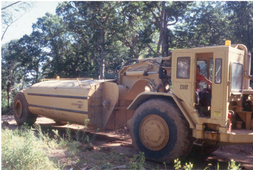
Fig. 22.3 A large water truck used to pre-flush and post-flush the dye introduction site in an unsaturated system
