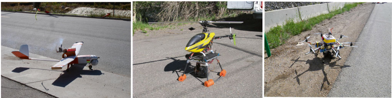
Fig. 14.7 Unmanned aerial systems (UAS), fixed-wing aircraft, a helicopter and hexa-copter used to obtain aerial photos and video (Photos courtesy of the Colorado Department of Transportation)
