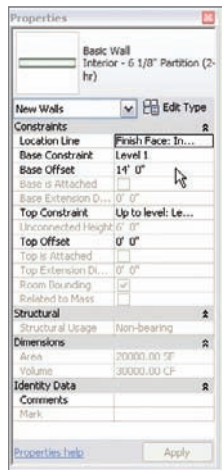
FIGURE 9.27 Modifying the dimensions of the 6 1/8" wall
