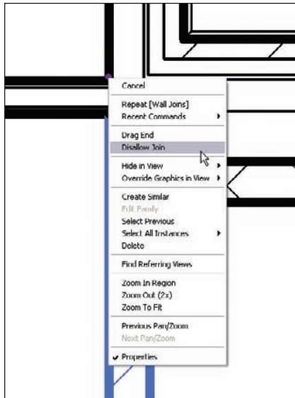
FIGURE 2.57 By right-clicking on the wall's end grip, you can tell Revit to disallow that wall's join function.
