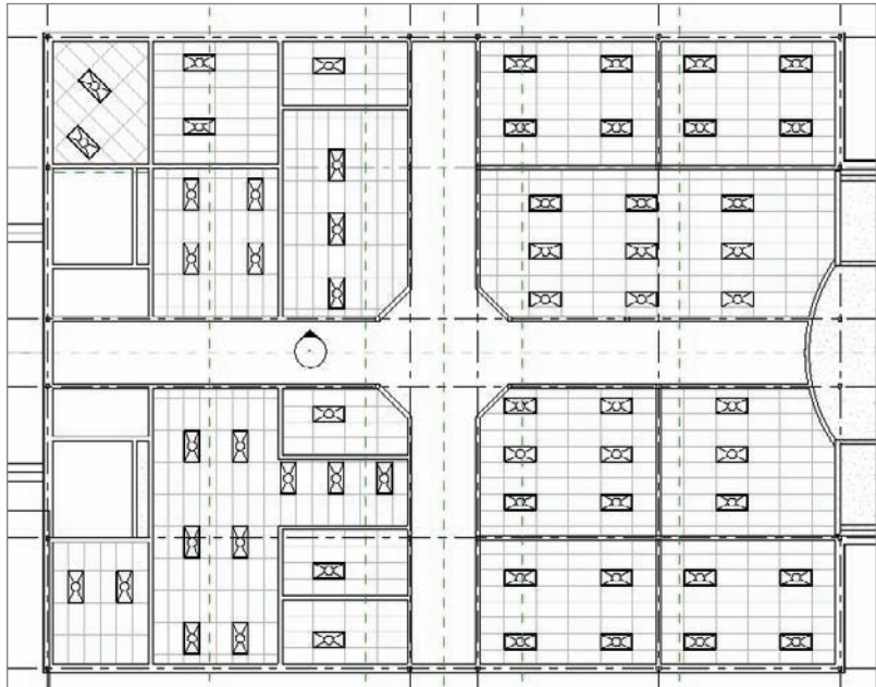
FIGURE 9.48 Adding lights to the rest of the ceilings
