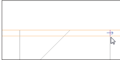
FIGURE 2.62 This line indicates where the wallboard will be cut. The blue arrow indicates the side of the material that will remain.
