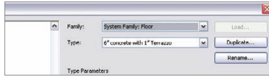
FIGURE 10.56 You must add a floor at the Level 3 floor plan for the stairs to have a landing.
