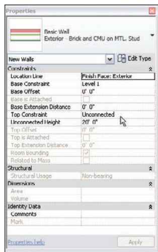
FIGURE 1.12 The Instance Properties will change only the currently placed item or the currently selected item.
