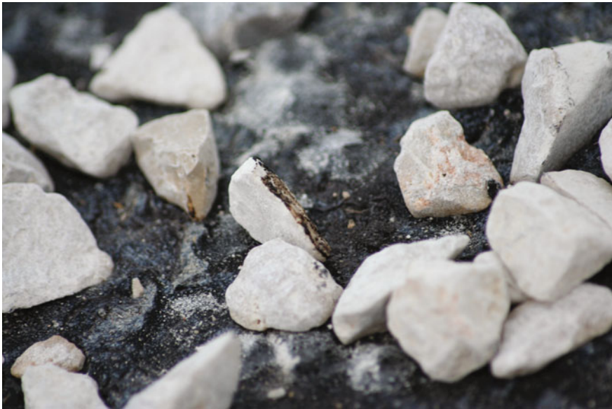
Fig. 3.9 A photograph showing aggregate particles placed on an emulsion surface; the dust particles can be seen interfering with bonding with the emulsion (Photograph by A Bhasin)
