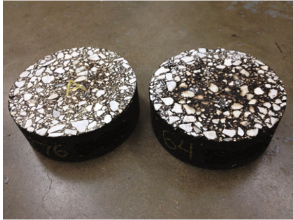
Fig. 7.5 Saw cut cross sections of two asphalt mixture specimens with same binder content, aggregate type and gradation but different binder types; the specimen on the left shows less absorption in the aggregates compared to the specimen on the right; the absorption can be seen in the form of discoloration of the aggregate particles at its interface with the binder (Photograph by A Bhasin)
