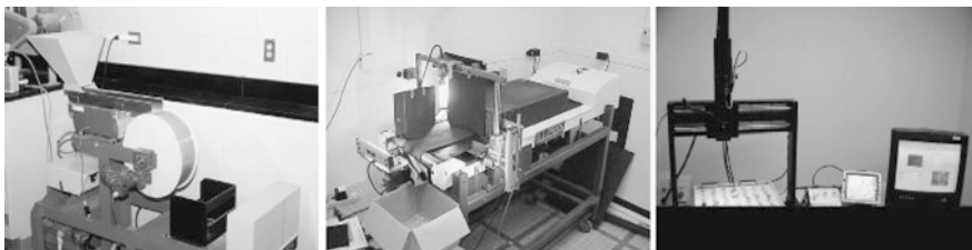
Fig. 3.27 Three different devices used to capture aggregate images to determine shape, angularity and/or texture (With permission from TRB through the National Academy of Sciences, Prowell, B., and Brown, R., Aggregate Properties and the Performance of Superpave-Designed Hot-Mix Asphalt, NCHRP Report 539)
