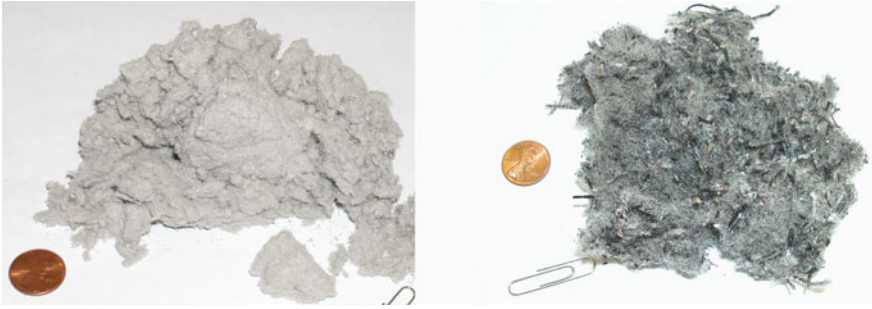
Fig. 3.6 Typical fibers used in the production of SMA mixtures to prevent drain down of asphalt binder (cellulose is shown to the left and long tire rubber fiber on the right ) (Chowdhury et al. 2006).
