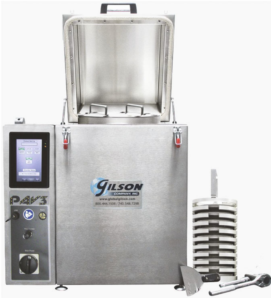
Fig. 2.15 Image of a typical PAV device for long-term aging (Image courtesy of Gilson Company Inc., USA)
