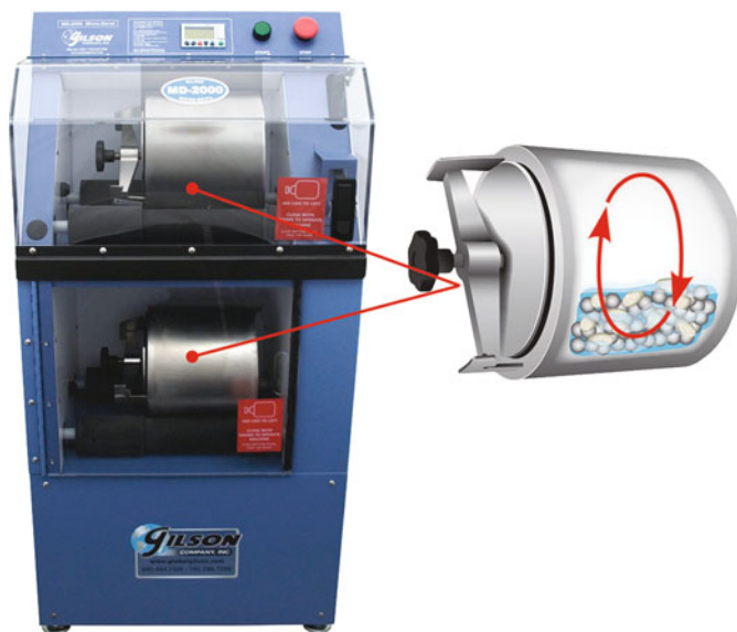
Fig. 3.14 A photograph showing the micro-deval apparatus ( left ) and a schematic of the abrasion process ( right ) (Image courtesy of Gilson Company Inc., USA)
