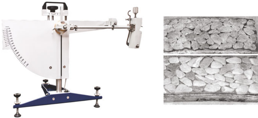
Fig. 3.13 A photograph showing the British pendulum ( left ) and a test coupon before ( top right ) and after ( bottom right ) being swung over a rubber test pad for a specified number of times (British pendulum image courtesy of Gilson Company Inc., USA; Polished coupon: Gatchalian et al. 2006)
