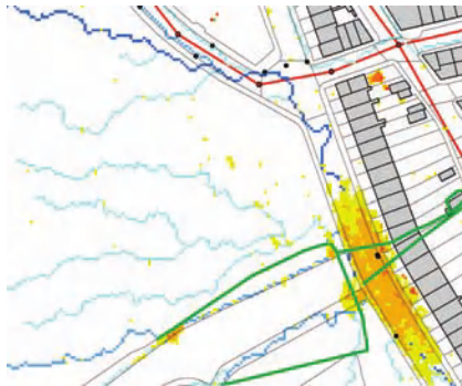
Fig. 13.11 Ponds and flowpaths derived from the digital elevation model (DEM). Flowpaths in blue; location of ponds in yellow; surface water system in green; combined sewer system in red; node manholes as small black circles; gullies identified as dots by the kerb lines.
