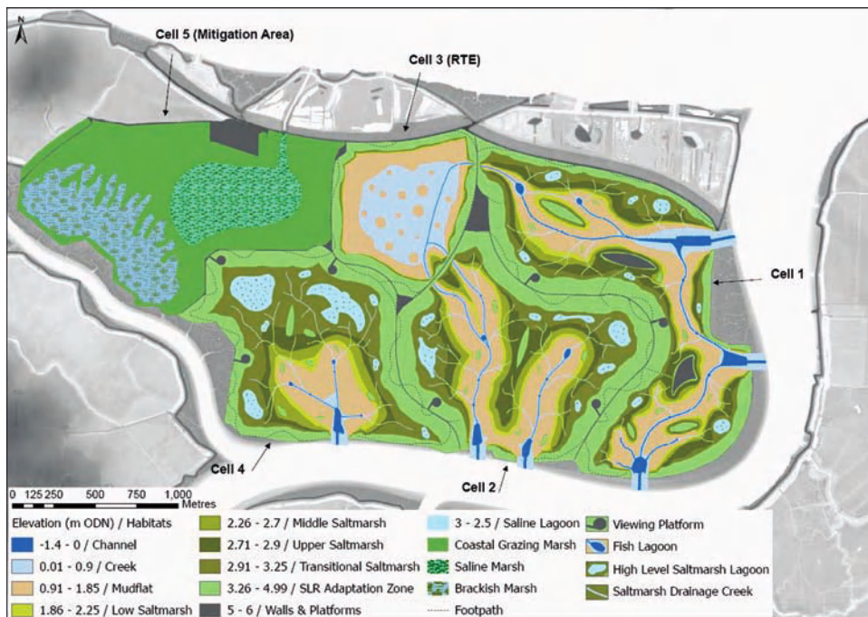
Fig. 4.4 Example of dendritic network design for a more extensive realignment on the Wallasea site.
