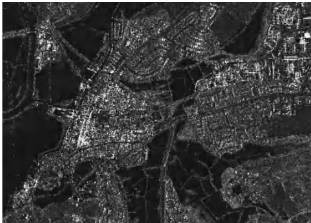
Fig. 11.4 A 3-m-resolution TerraSAR-X image of flooding in Tewkesbury, UK, in July 2007 (dark regions are water and radar shadow areas). © DLR (2007).
