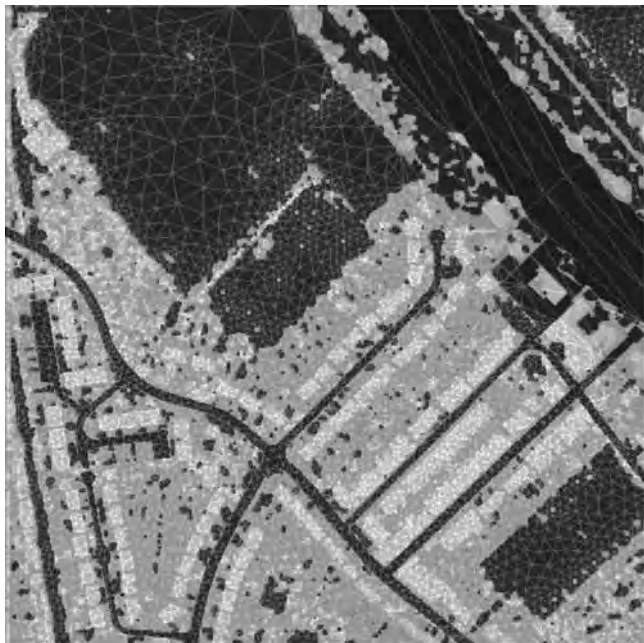
Fig. 11.3 Mesh constructed over vegetated urban area (red = mesh, blue = building/taller vegetation heights; a river is present in the northeast corner). After Mason et al. (2007a). (See the colour version of this figure in Colour Plate section.)
