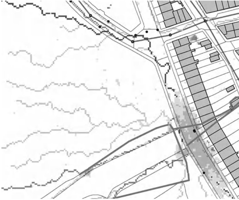
Fig. 13.11 Ponds and flowpaths derived from the digital elevation model (DEM). Flowpaths in blue; location of ponds in yellow; surface water system in green; combined sewer system in red; node manholes as small black circles; gullies identified as dots by the kerb lines. (See colour version of this figure in Colour Plate section)
