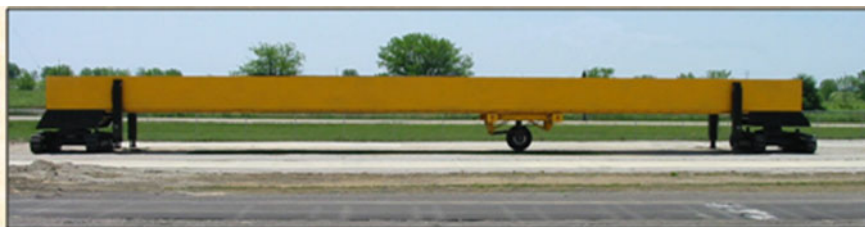
Fig. 1.20 Accelerated Loading and Testing Assembly (ATLAS)
