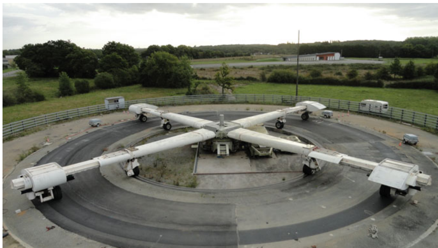
Fig. 1.9 View of the LCPC fatigue test track [15]
