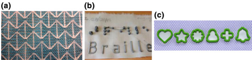
Fig. 3 Published examples of 3D printing on textiles: a auxetic print [18], b braille print [2], and c grommets [17]
