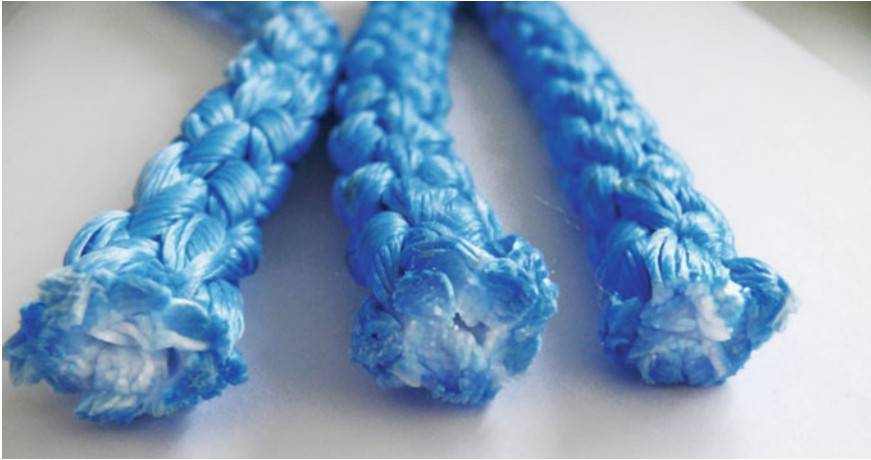
Fig. 1 Insufficient coating input into PES-rope (white core), diameter 20 mm
