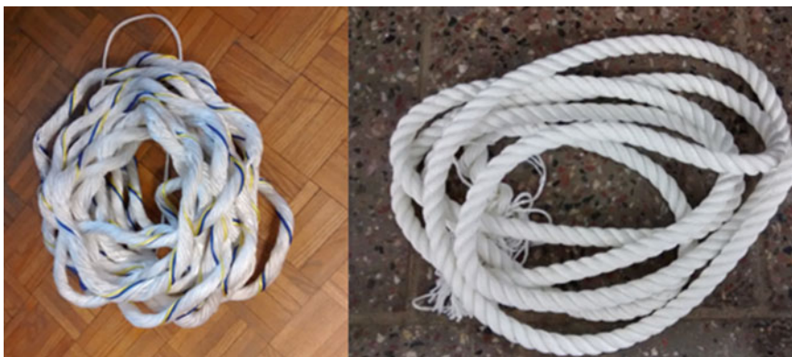
Fig. 3 Left side mixed rope made from PES-PP, right side pure PES-rope
