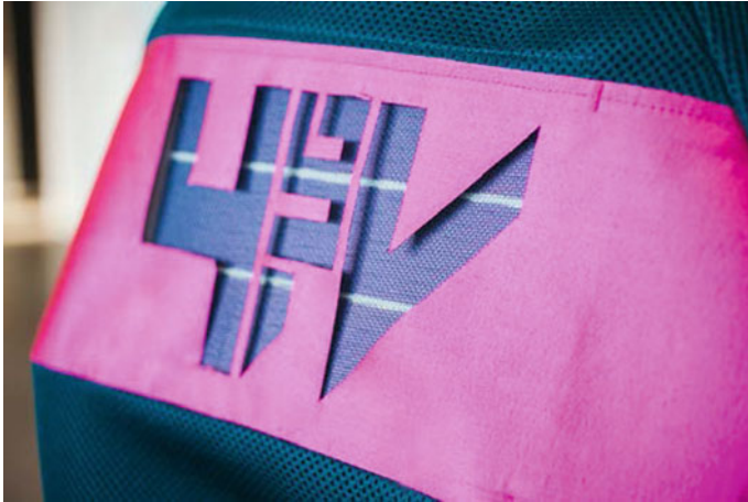
Fig. 5 Laser-cut pattern placed on the solar module, fixed on a net-lace fabric
