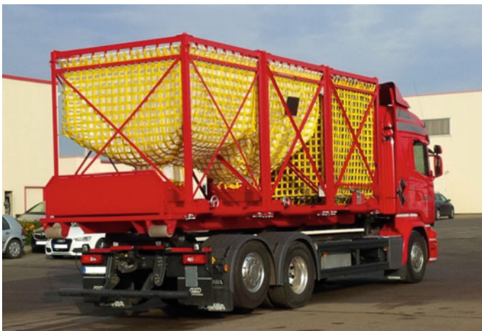
Fig. 13 Modular, mobile silos on truck
