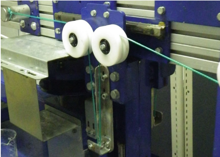
Fig. 1 Setup for abrasion tests
