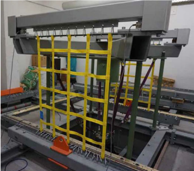
Fig. 2 Tensile tests on two network segments
