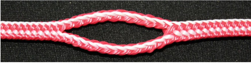
Fig. 4 Pattern 1—Crossing loop for 1 \times 16 to 2 \times 8 to 1 \times 16 geometry
