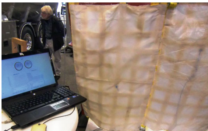
Fig. 8 Textile segments with integrated sensors and PC system
