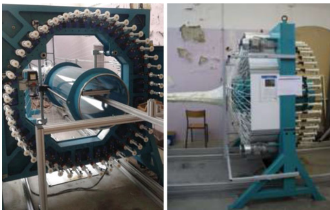
Fig. 1 Braiding loom (back and side view)
