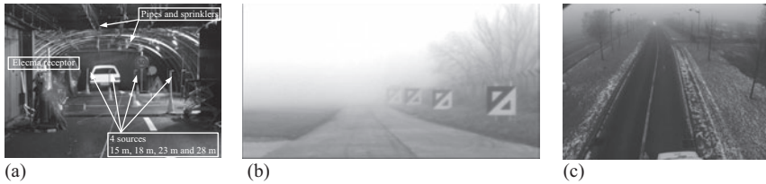
Figure 8.7 Tools used to test and validate the performance of the fog and validate camera-based fog detection and visibility range estimation algorithms. (a) Artificial fog chamber of Clermont-Ferrand. © 2010 IEICE. Reprinted with permission from Gallen R., Hautière N., Dumont E. “Static Estimation of the Meteorological Visibility Distance in Night Fog with Imagery”. Transactions on Information and Systems , E93-D (7): 1780–1787; (b) Calibration test bench. © 2006 IEICE. Reprinted with permission from Hautière N., Labayrade R., Aubert, D. “Estimation of the Visibility Distance by Stereovision: A Generic Approach”. Transactions on Information and Systems , E89-D (7): 2084–2091, 2006; and (c) Open road test: static acquisition
