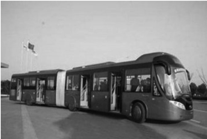
Figure 15.6 Biarticulated buses. © The Institute for Transportation and Development Policy (ITDP) www.itdp-china.org/en/city/yichang (Accessed on 30 March 2016)
