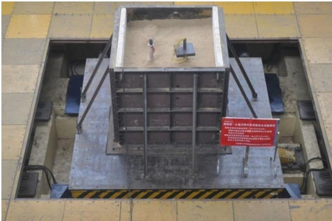
**Fig. 4** Setup of shaking table test on soil-micropile interaction
