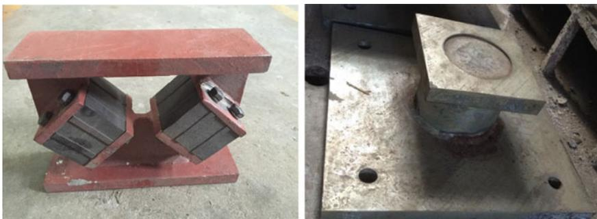
**Fig. 2** Scale models of new anti-vibration bearing and steel bearing
