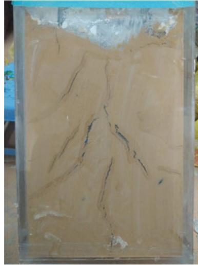
other two sides. The water was drained out along the electrode, and it flowed from the middle portion to the electrode. The soil shrank along the direction of the cross section and formed cracks along the vertical direction. Furthermore, the cracks extended from the middle section to the electrode direction with the vacuum pressure from the top surface of the soil (Fig. 21).
