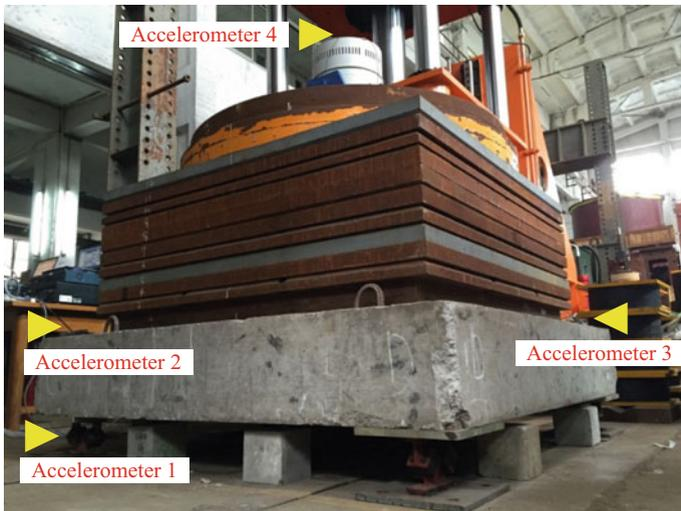
**Fig. 3** Test scheme of scale model test
