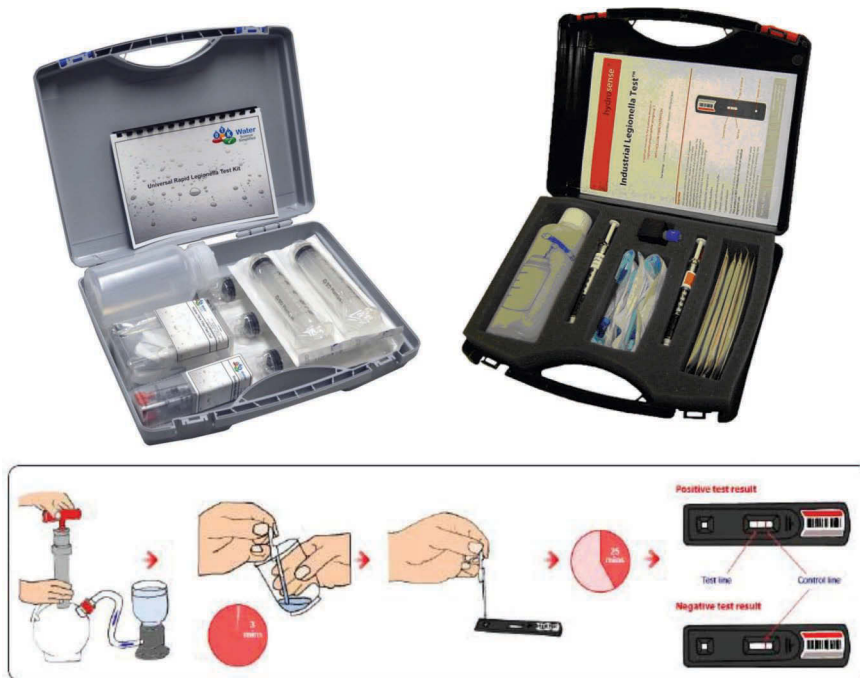
Figure 3.7 Legionella kits from Drop Test Kit and the evaluation of the lateral flow immunochromatographic assay (DTK, 2015).
