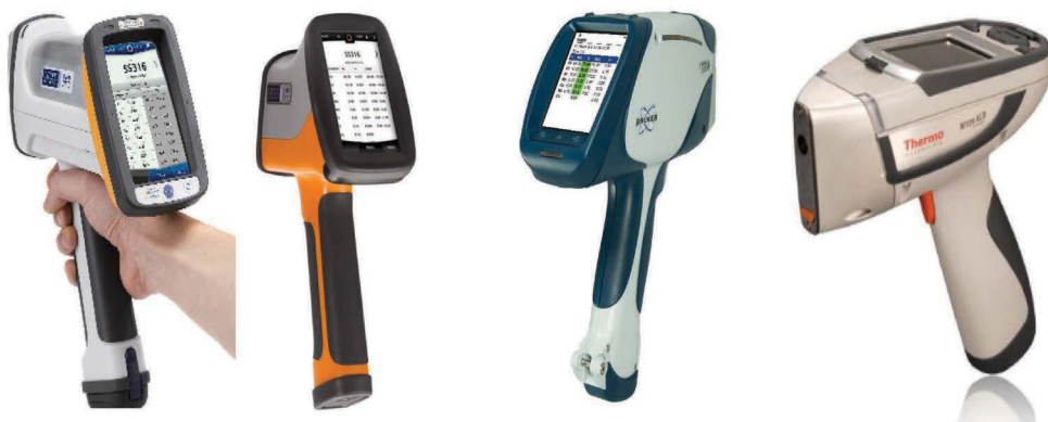
Figure 4.10 X-Met 8000 (Oxford), Delta (Olympus), S1 Titan (Bruker) and Niton XL3t (Thermo Analytics) handheld XRF devices.
