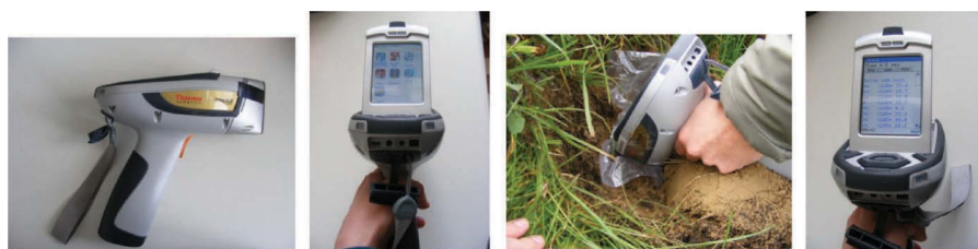
Figure 4.16 Portable XRF equipment, menu on the display, in situ field use and the results on the screen (Thermo Scientific, 2015).
