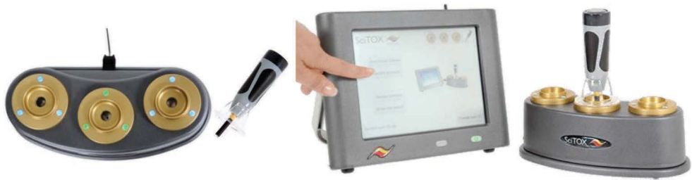
Figure 3.13 The SciTOX electrochemical sensor detects the signal of an artificial electron-acceptor which captures the electrons from the energy-producing process of the microorganisms (SciTox, 2015).
