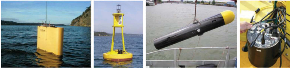
Figure 3.10 Compartments of the SMHI Måseskär buoy: the Sea Tramp, a surface and a subsurface buoy and the SeaMoose (Ocean Origo, 2015).
