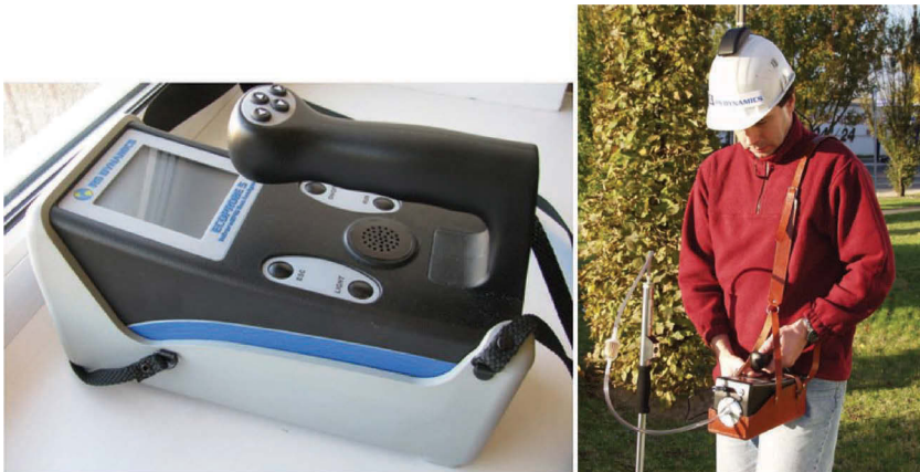
Figure 4.4 Ecoprobe 5 equipment and its application in the field (Ecoprobe 5, 2015).
