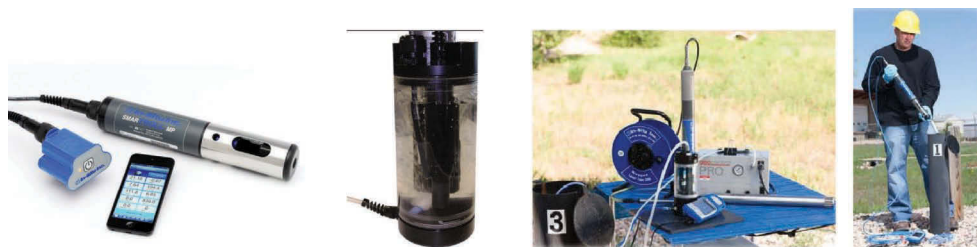
Figure 4.8 TROLL® 9500 sensor system; flow-through chamber; field installation; measuring in a groundwater well (TROLL 9500, 2015).
