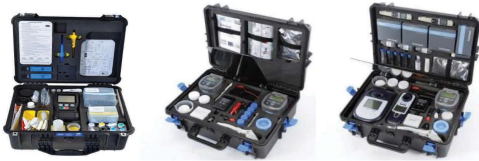
Figure 3.5 Rapid Response Test Kit (Eclox, 2015), Portable Microbiological Water Quality Laboratory (Potatest®, 2015) and Portable Water Quality Laboratory (Potatech®, 2015).
