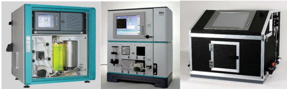
Figure 3.9 AlgaeTox, DaphTox, FishTox: online toxicity assessing equipment from bbe Moldaenke (TOX, 2015).
