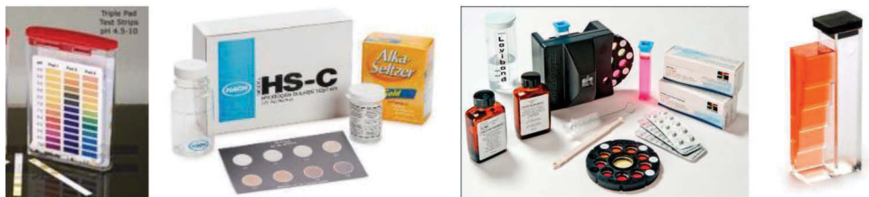
Figure 3.4 Test strips for sensitive pH measurement (Indigo, 2015), color chart for hydrogen sulfide analyses with reagent paper (Hach, 2015), comparator color discs (Comparator disc, 2015) and cube for iron (Comparator cube, 2015).
