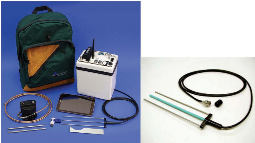
Figure 4.6 MiniTrase Kit portable soil moisture measuring instrument using Time Domain Reflectometry (TDR). The kit and the TDR sensor (Photos: MiniTrase Kit, 2015).
