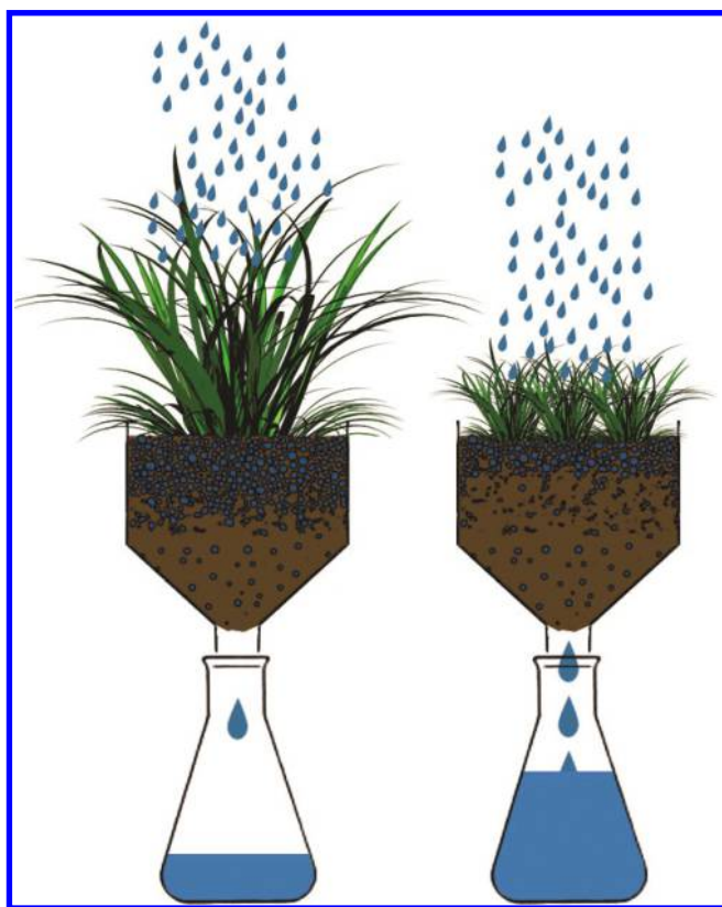
Figure 8.20 Principle of the lysimeter: water filtrating through the soil is collected and analyzed.
