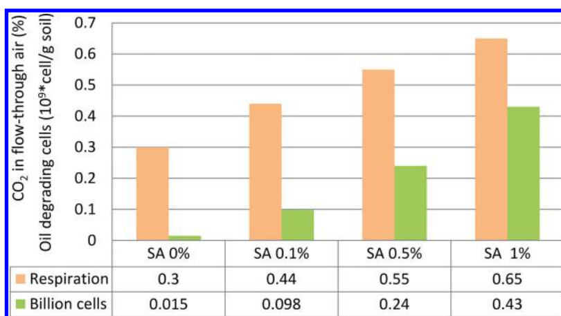
Figure 2.12 Increase in transformer oil-degrading cell concentration and respiration rate due to treatment with a bioavailability-enhancing agent (Molnár, 2006).
