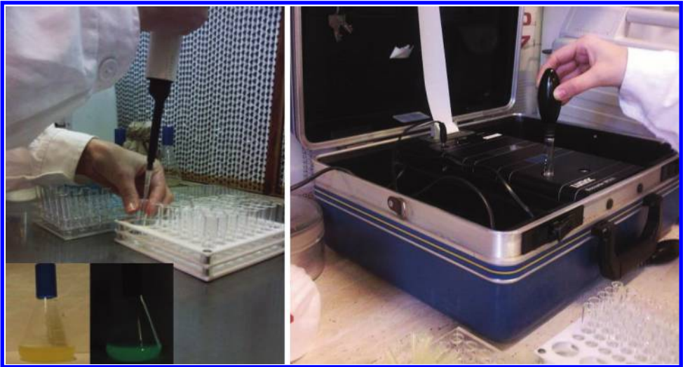
Figure 5.18 Luminescence inhibition of contaminated soil measured by a portable luminometer.
