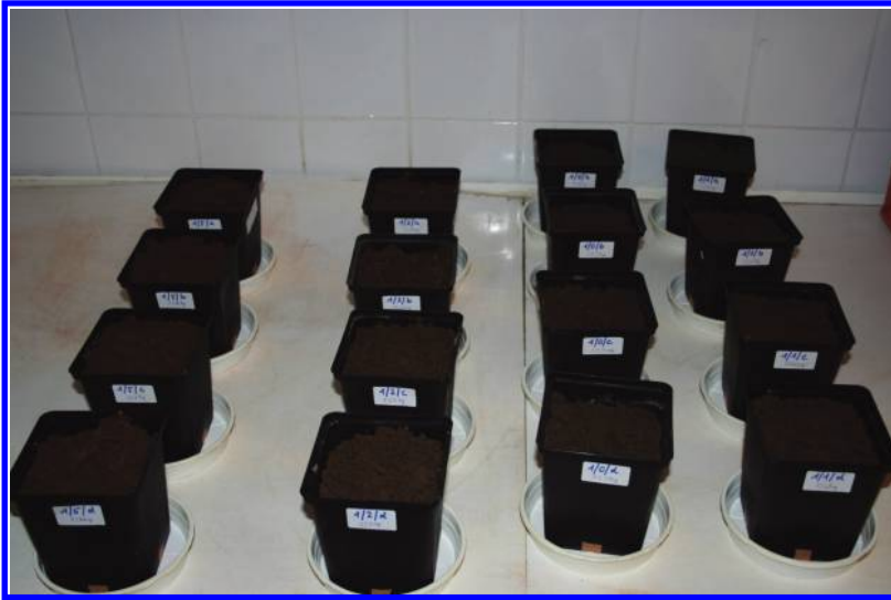
Figure 8.9 Test series for screening biodegradation in soil and the effect of enhancing additives.
