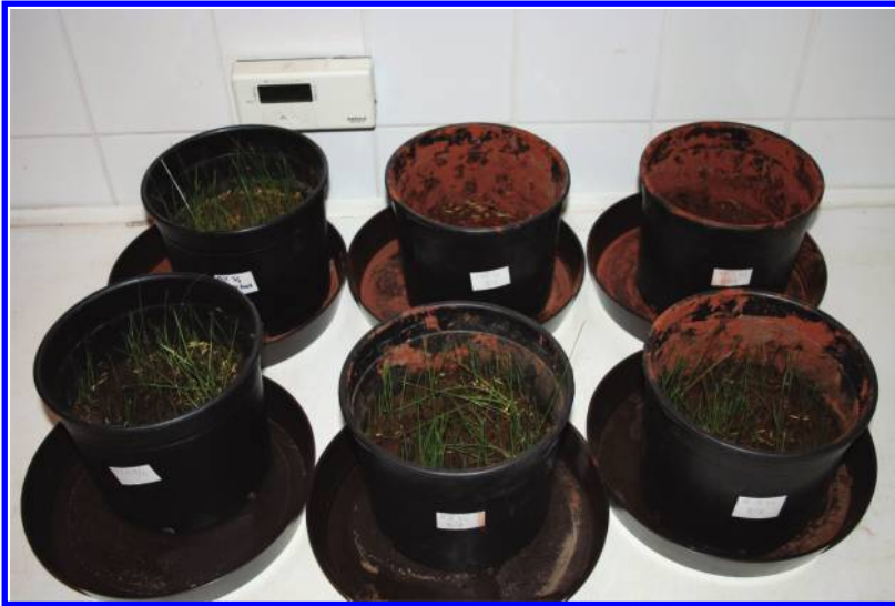
Figure 8.10 Serial tests in static microcosms: soil contaminated with increasing concentrations of red mud.
