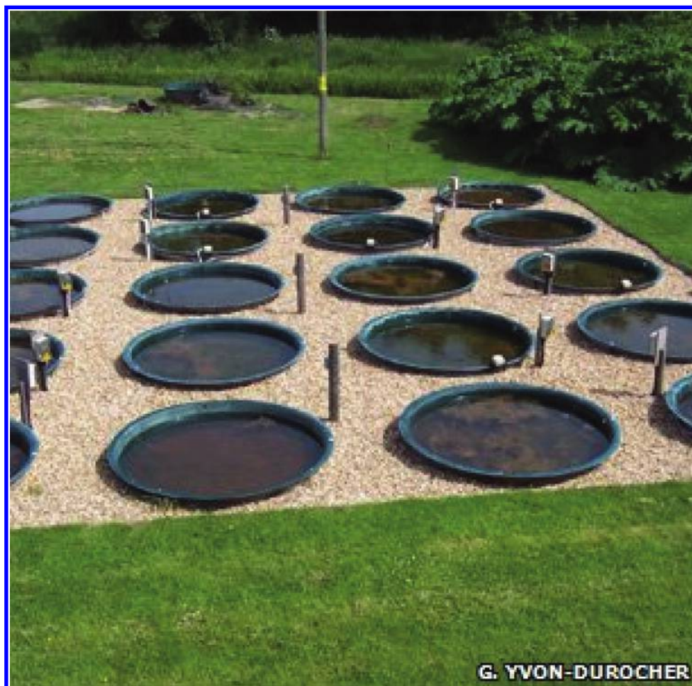
Figure 8.3 Microcosms for investigating the impact of warming on a freshwater ecosystem (Yvon-Durocher, 2013).
