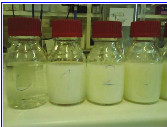
Figure 8.11 Solubilization of groundwater contaminants using tensides and cosolvents in increasing concentration from left to right.
