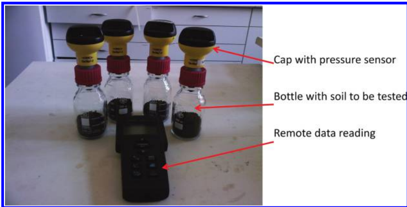
Figure 2.6 Closed bottle for testing the respiration rate in soil based on manometry. The pressure decrease is detected by the sensor in the cap and read remotely.
