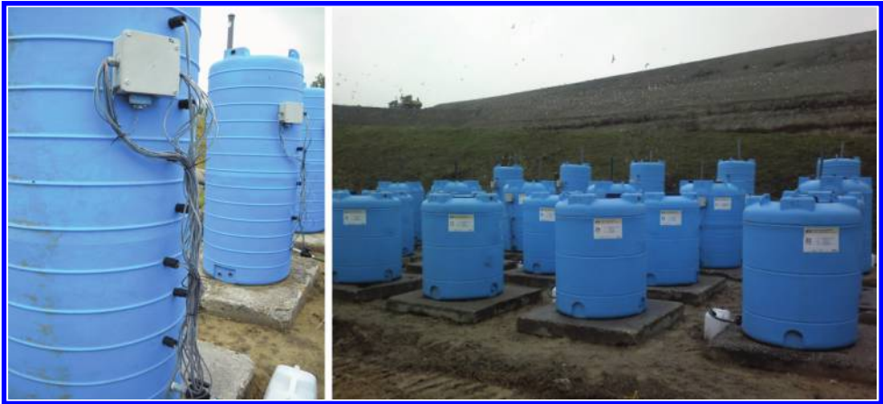
Figure 5.31 Lysimeters filled with soil above the surface with built-in sensors.
