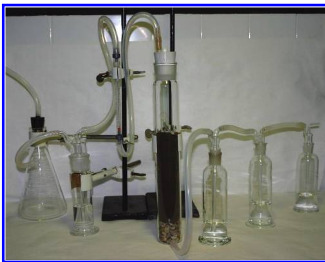
Figure 8.14 Dynamic soil microcosms with flow-through column reactors.
