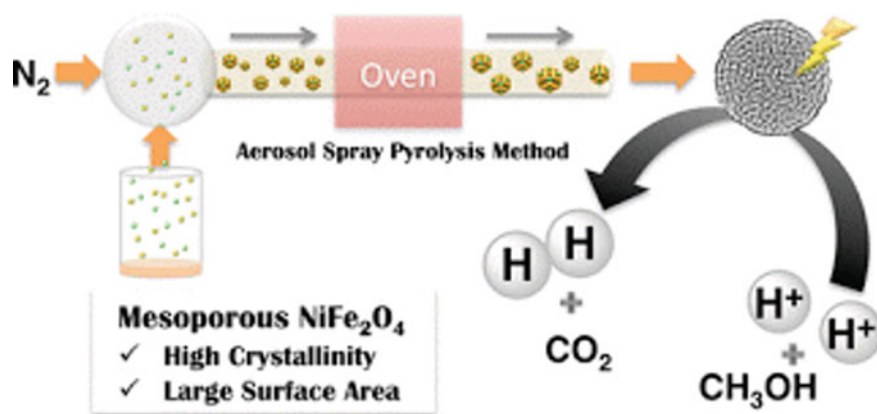
Fig. 2.14 Synthesis of \text{NiFe}_2\text{O}_4 via LF-FSP. Reproduced with permission from Ref. [112]. Copyright (2014) American Chemical Society
