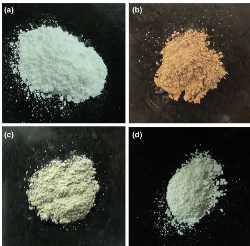
Fig. 4.67 MOF A520 as-synthesized (a), A520-723 K (b), A520-823 K (c), A520-923 K (d). Reproduced with permission from Ref. [484]. Copyright (2016) Elsevier
