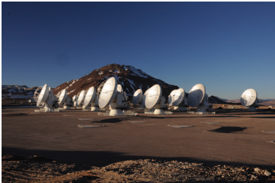
FIG. 14.1 The Atacama Large Millimeter Array at its 16,500-foot elevation site in northern Chile. At the time of this photo, 19 radio telescopes were in the Compact Array. Today, 66 radio telescopes are spread out across up to 15 km in the Atacama Desert. (Credit: W. Garnier, ALMA (ESO/NAOJ/NRAO/NSF))
