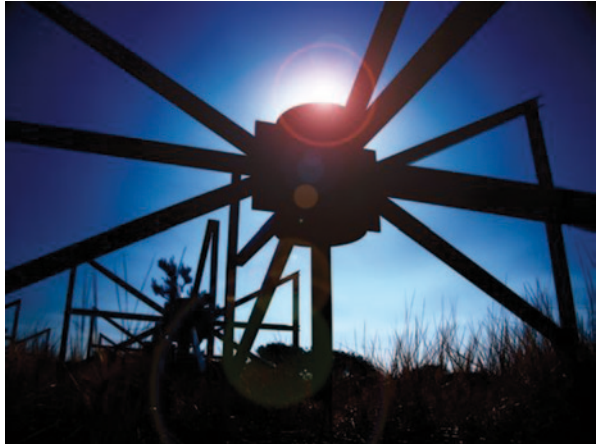
FIG. 15.7 A close-up silhouette of a spider-like MWA dipole antenna, an element of a tile such as seen in Fig. 15.6. (Credit: Natasha Hurley-Walker; ICRAR, Curtin University)
