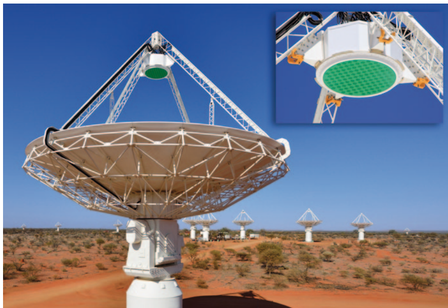
FIG. 15.5 CSIRO's ASKAP antennas at the Murchison Radio-astronomy Observatory showing a close-up on the innovative new 'radio camera,' the green honeycomb structure, that gives the telescope its world-class sensitivity and speed. It acts as if there were 96 small antennas situated at the focus. That gives 96 beams on the sky, each collecting data and for a survey instrument this greatly speeds up the data collection process, and also gathers staggering amounts of information. (Credit: CSIRO)
