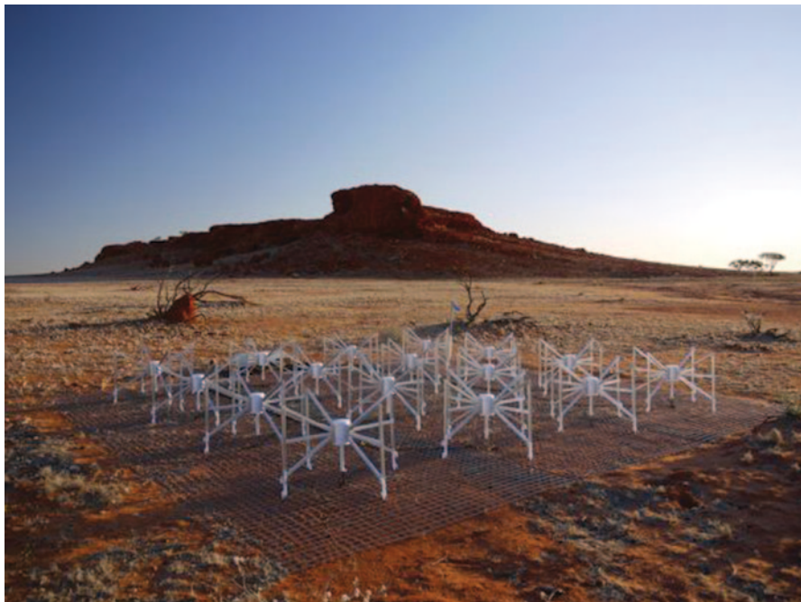
FIG. 15.6 A 'tile' consisting of 16 dual-polarization dipole antennas, one of 128 that make up the Murchison Wide-field Array. The MWA is being used to find evidence for the Epoch of Re-ionization and will hopefully detect the birth of the first stars and galaxies in the universe. (Credit: Natasha Hurley-Walker; ICRAR, Curtin University)
