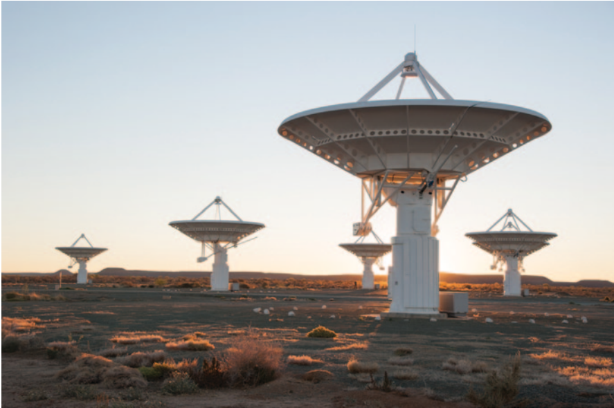
FIG. 15.2 The KAT7 array in South Africa, the pathfinder for MeerKAT, at the SKA site consists of seven dishes, each 13.5 m in diameter. The stark semi-desert terrain of the Karoo in the Northern Cape assures that the observatory is well away from civilization with its penchant for producing unwanted radio interference from cell phones and the like. (Credit: SKA South Africa)
