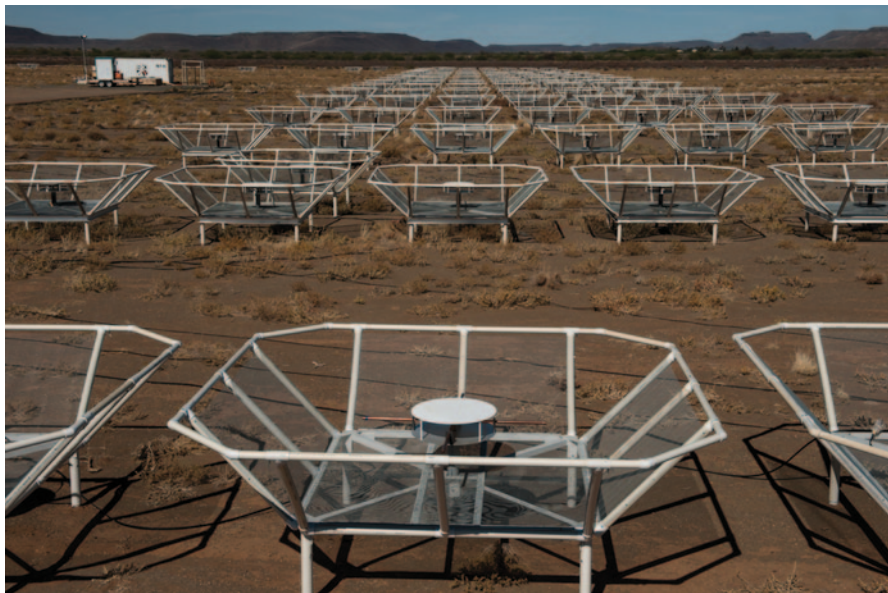
FIG. 15.8 The antennas of PAPER at the South African SKA site, each consisting of crossed dipoles in a frame that is called a ground screen, which shields against radio emission from the ground below. (Credit: SKA South Africa)
