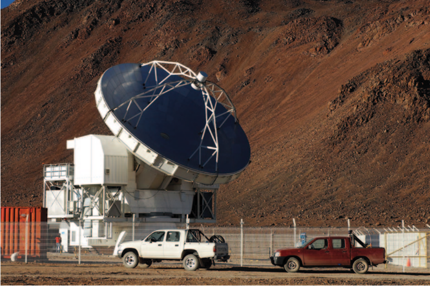
FIG. 14.6 The sturdy APEX radio telescope at the desolate ALMA site in Chile. The 12 m antenna surface is so accurate that its surface is shiny and you can see reflection of a feed support leg in the dish. (Credit: ESO/F. Kamphues)
