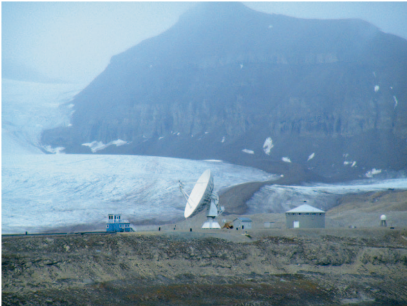
FIG. 1.6 A 78^{\circ} 55' North latitude the radio telescope in Ny Ålesund in the Spitsbergen islands, also known as Svalbard, forms part of the European VLBA Network and is used mainly for geodesy. Regular observation of quasars allows the annual shift in location of the island to be determined. In the background a glacier seems to threaten its existence. (Photo by the author taken from a cruise ship in King's fiord)
