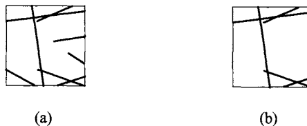
Fig. 8.17 (a) Domain C in Fig. 8.14 containing 8 discontinuities; and (b) 5 discontinuities in domain C are interconnected.
