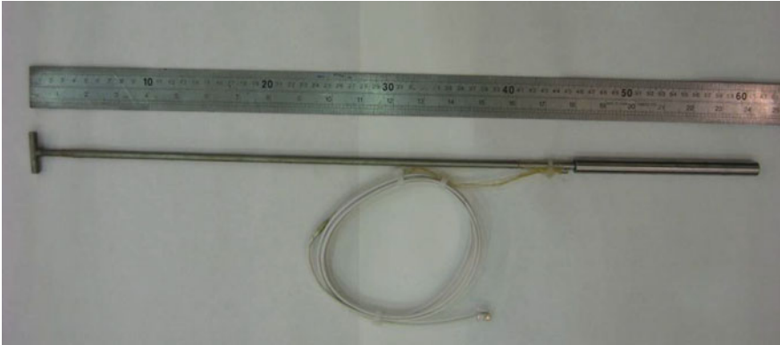
Fig. 5.1 The T-bar penetrometer used in the test
