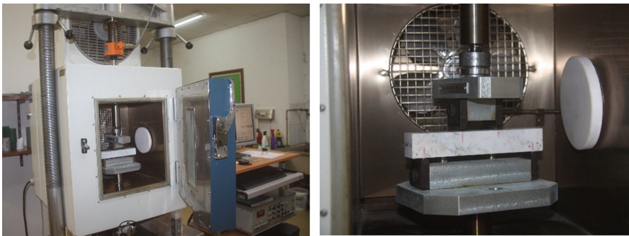
Fig. 3. Experimental setup for fracture toughness tests at different temperatures.
