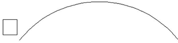
FIGURE 8.19 Setup for a Path Array.
