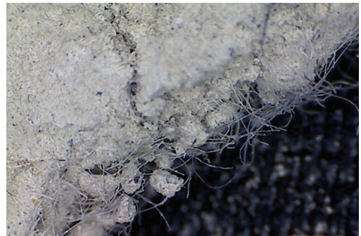
Figure 2. Artificially cemented soil stabilized with recycled fibers from scrap tires.
