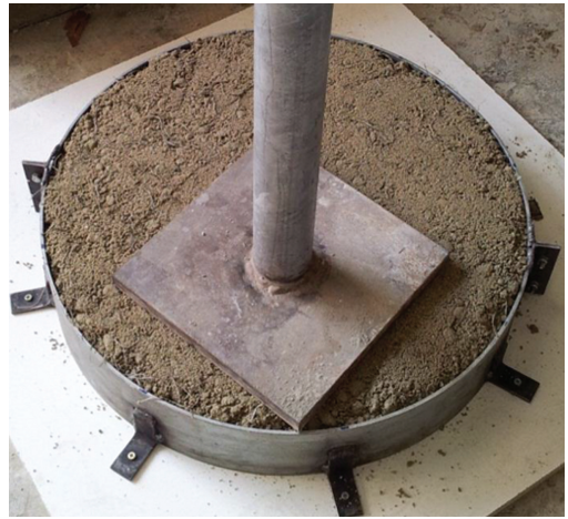
Figure 3. Initial manual compaction of specimen.
