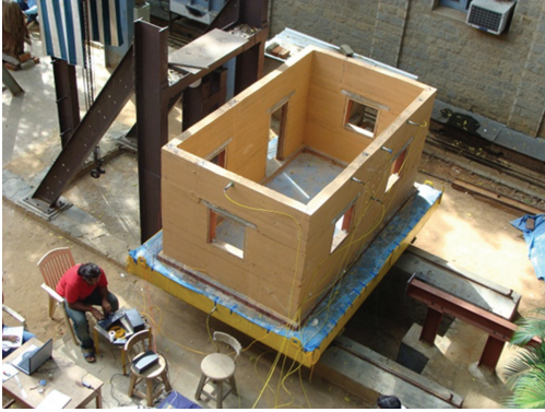
Figure 3. View of building model with instrumentation ready for testing.
