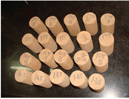
Figure 2. Sand cylinders made by MICP.
