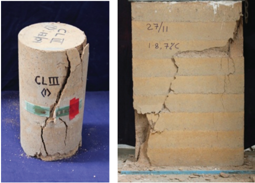
Figure 5. Typical failure patterns.
