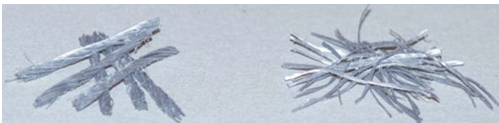
Figure 2. Macro-synthetic fibres used. On the left: bundles; on the right: individual strands.
