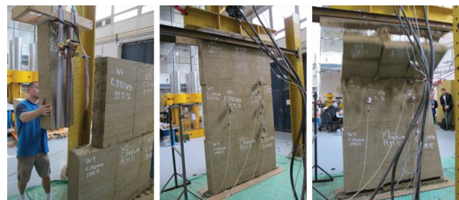
Figure 4. Assembling of the testing wall and final collapse.
