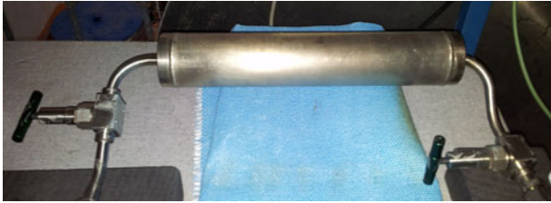
Figure 3.4: A photograph of the small purifier cartridge originally used for the recirculation system of MEDIUM ARGONTUBE [24].
