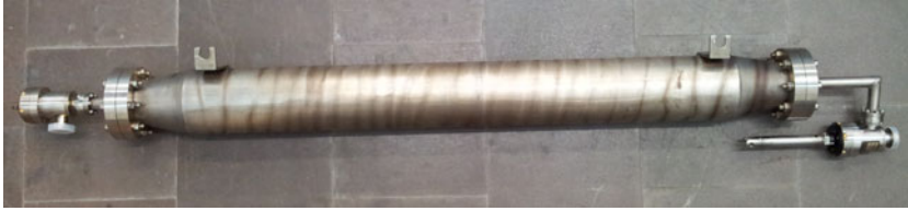
Figure 3.1: A photograph of one of the argon purifiers that are installed in the ARGONTUBE recirculation system. Both, filter in- and outlet are closed by all-metal angle valves 1 which are compatible with cryogenic liquids.
