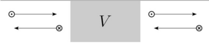
Fig. 8.4 Scattering of an edge state on a time-reversal symmetric defect V . In a two-dimensional time-reversal invariant topological insulator with \hat{\mathcal{T}}^2 = -1 , having a single Kramers pair of edge states, the incoming electron is transmitted through such a defect region with unit probability
