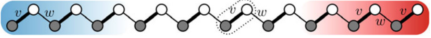
Fig. 1.1 Geometry of the SSH model. Filled (empty) circles are sites on sublattice A ( B ), each hosting a single state. They are grouped into unit cells: the n = 6 th cell is circled by a dotted line. Hopping amplitudes are staggered: intracell hopping v (thin lines) is different from intercell hopping w (thick lines). The left and right edge regions are indicated by blue and red shaded background
