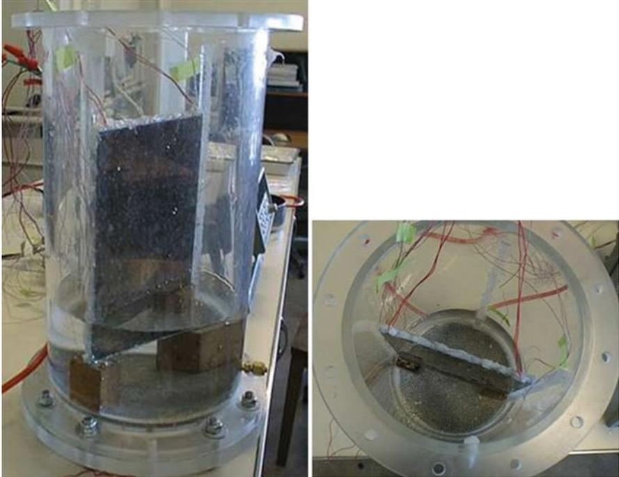
Fig. 4.2 Container with heater-plate assembly
