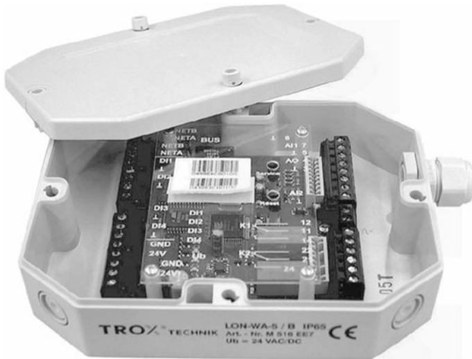
Fig. 4.7 LON component for controlling an airflow regulator [15]
