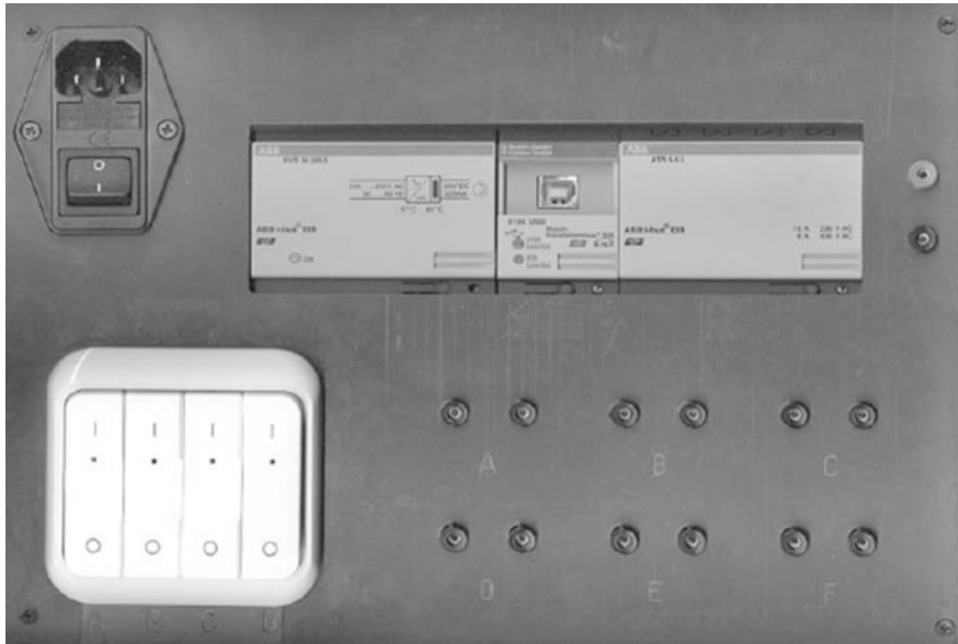
Fig. 3.39 A basic KNX system with an IEC power socket, power supply [9], USB interface [13], a six-gang switch actuator [9], a four-gang switch (rocker) sensor [13], and six output sockets (relays) A–F
