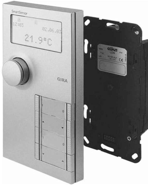
Fig. 4.2 Room operating device with LON interface for decentral installation [5, 6]
