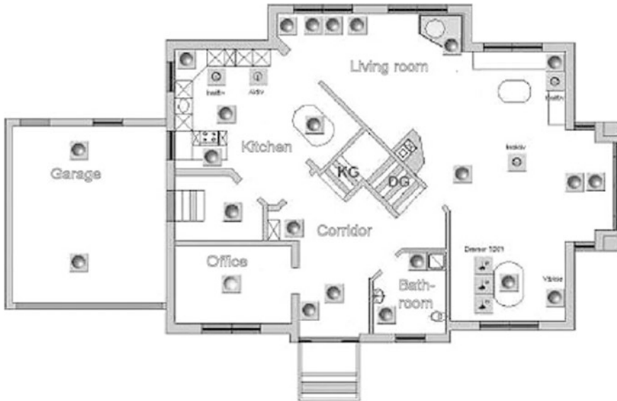
Fig. 3.58 An image on a touch-screen control panel showing the first floor lighting control system in the CIBEK show house in Limburgerhof, Rhineland-Palatinate, Germany [14]
