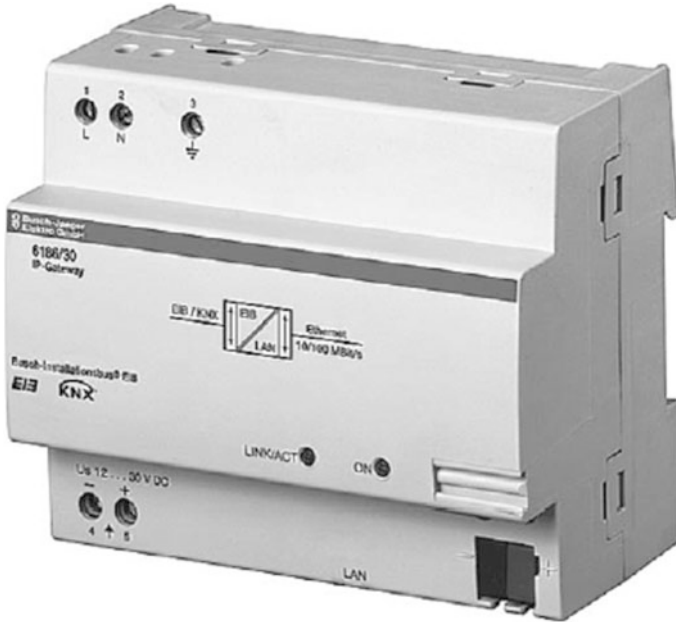
Fig. 3.59 IP Gateway [Busch-Jaeger Elektro]
