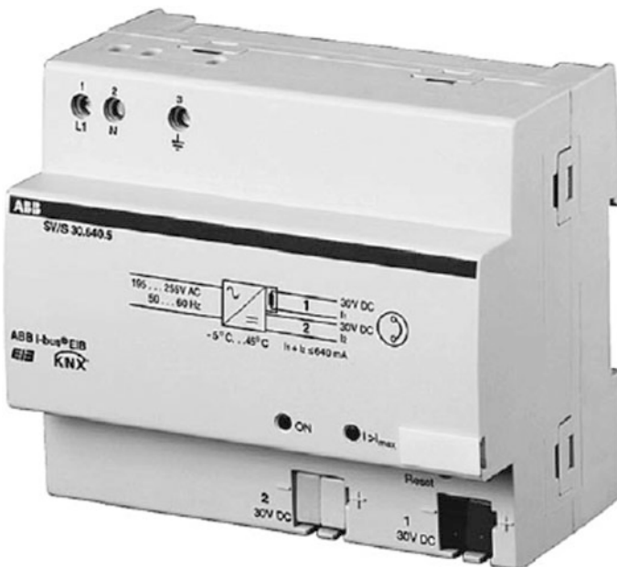
Fig. 3.12 A power supply unit 640 mA (RM) with an integrated choke and two 30 V DC outputs [9]
