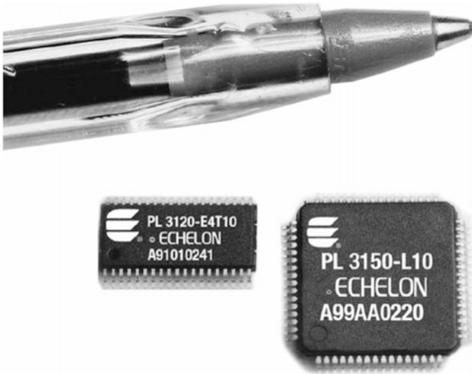
Fig. 4.11 The neuron chip [4]
