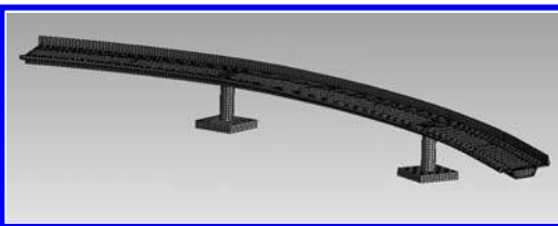
Figure 2. Shell/solid FE model.
