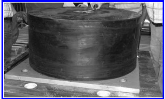
Figure 2. Lead rubber bearing after dynamic prototype test.
