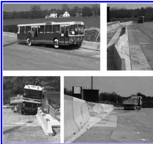
Figure 1. H2/TB51 test with 13 ton bus and H4b/TB81 test with 38 ton truck.
