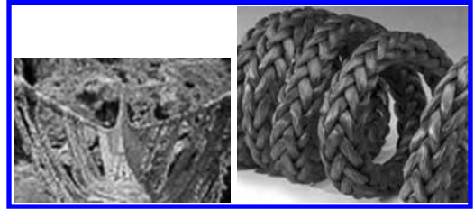
Figure 1. Last surviving hemp rope Inca Bridge. Figure 2. Synthetic Rope used for mooring.
