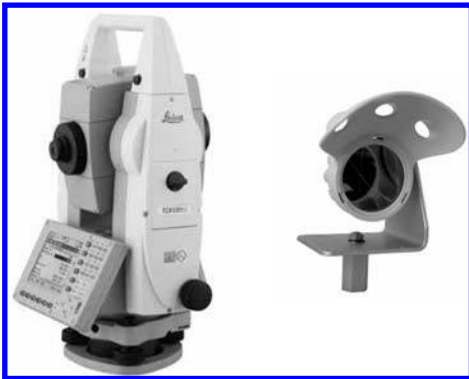
Figure 1. Automated TPS: Leica TCA1201M and Reflector.
