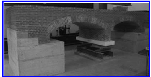
Figure 1. The experimental model of the twin-spans masonry arch bridge built in the laboratory.
