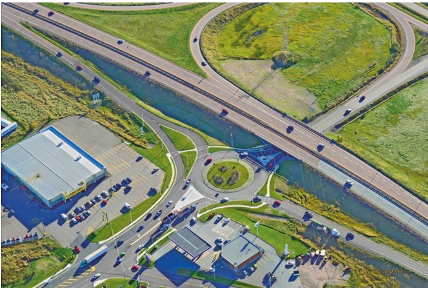
Fig. 3.50 Typical Canadian one-lane roundabout
