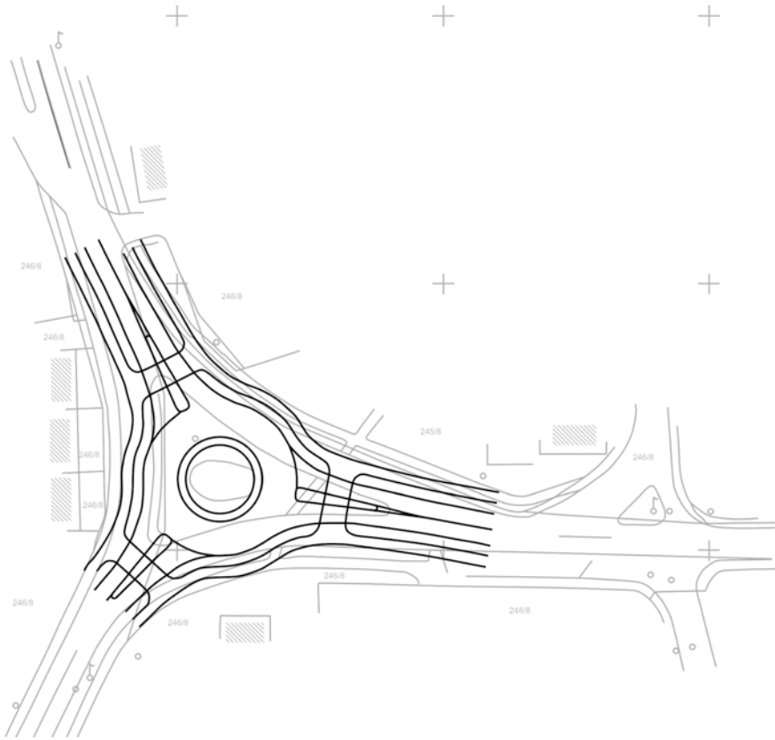
Fig. 3.1 Verification of the spatial criterion for a roundabout on an existing Y intersection; City of Poreč, Croatia
