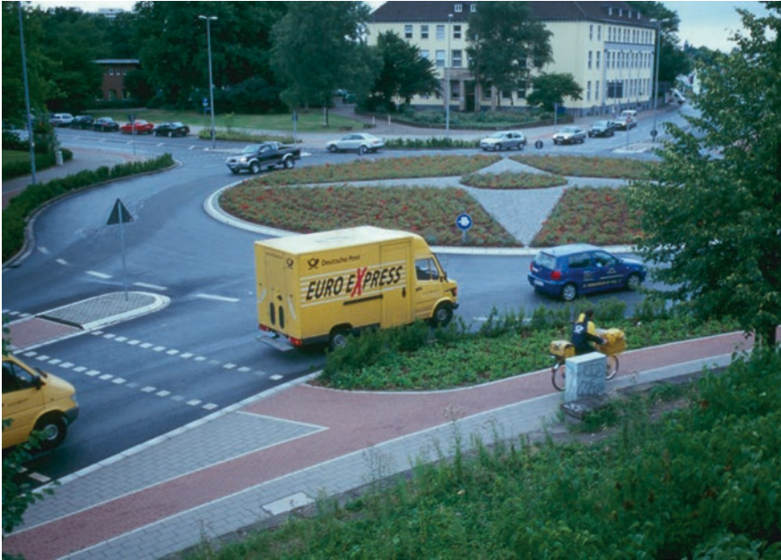
Fig. 3.23 Typical German compact semi-two-lane roundabout; Oberhausen
