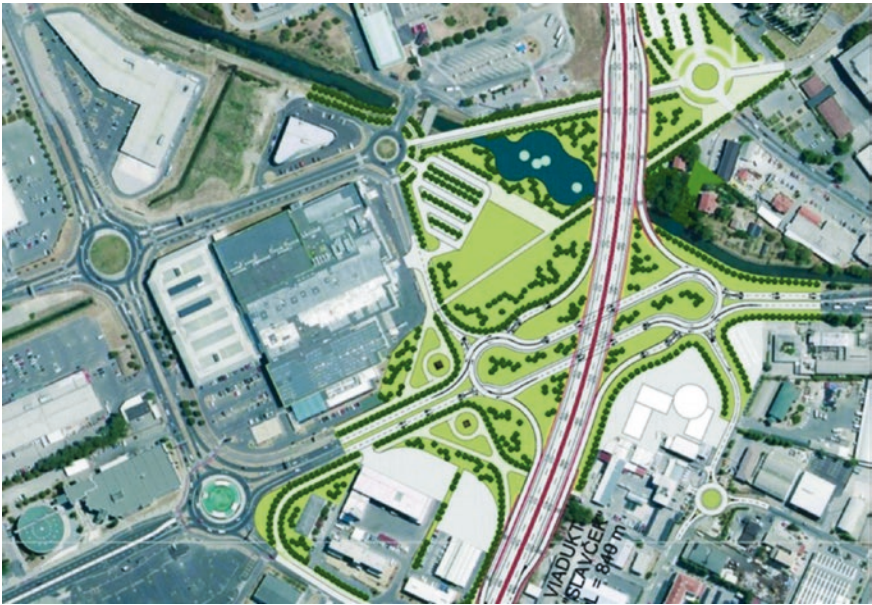
Fig. 4.42 The first Slovenian idea for a solution that included the dog-bone roundabout; city of Koper
