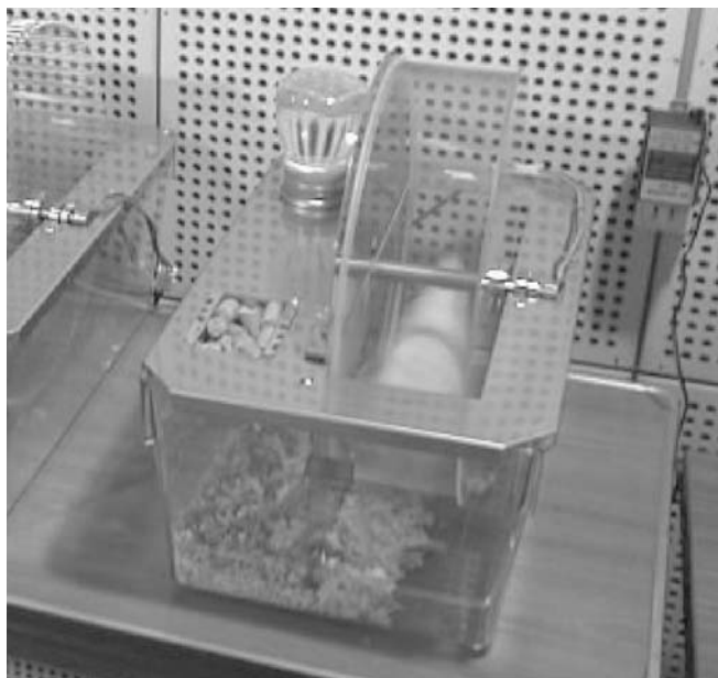
Fig. 1. Home cage equipped with running wheel (diameter 30 cm). Rats were housed individually with a 12-h light/dark cycle and had free access to food and water. They could enter the running wheel at any time, and the number of wheel turns per minute was counted continuously using an analog/digital interface and computer software
