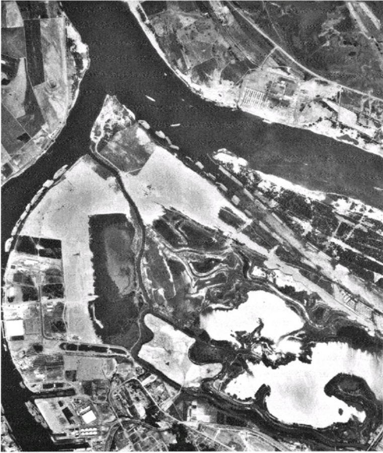
Figure 5.6. Aerial photographs are acquired by the government on a regular basis and are available from archives. Here the presence of riverine systems of the Columbia and Willamette have formed deposits which were developed into urban and industrial areas, including a port. Note the presence of lacustrine and riverine wetlands near Portland, Oregon.
