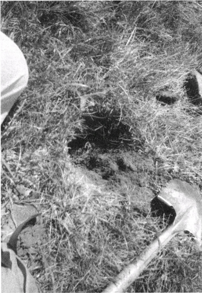
Figure 3.3. A good method to use in evaluating soils for wetland indicators is to dig a hole approximately 18 inches deep, and view subsequent seepage and/or standing water.
