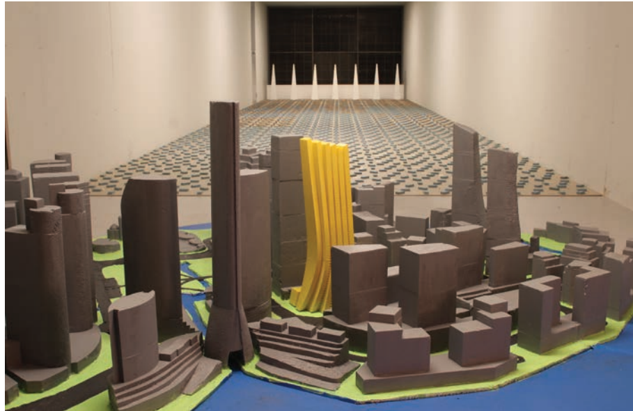
▲ Figure 3.3: Empire Tower, Reem Island, Abu Dhabi (future surrounds case). Wind tunnel testing performed in March 2009. © Windtech Consultants Pty. Ltd.
