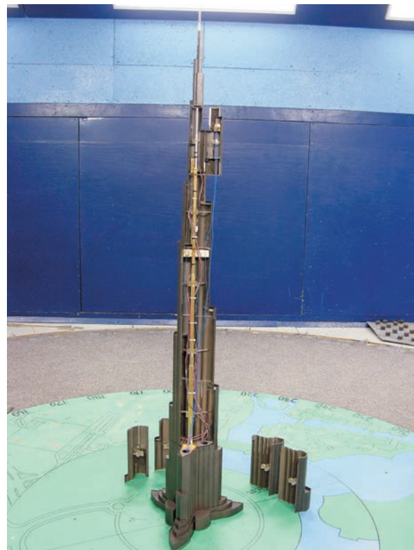
▲ Figure 3.8: Example of aeroelastic model illustrating inner spine for providing stiffness scaling, and segmented outer shell to provide shape and mass scaling. © RWDI
