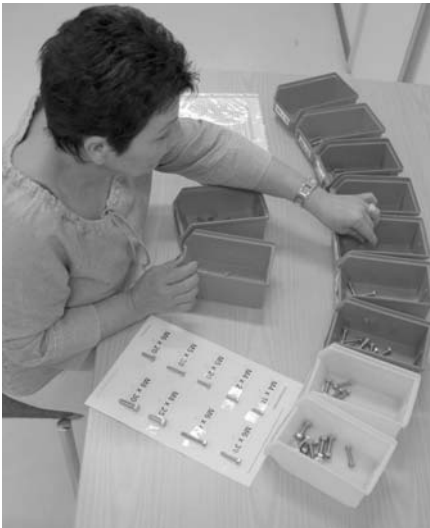
Fig. 5 – Standardised workstation for sorting and assembly (screws and nuts).
