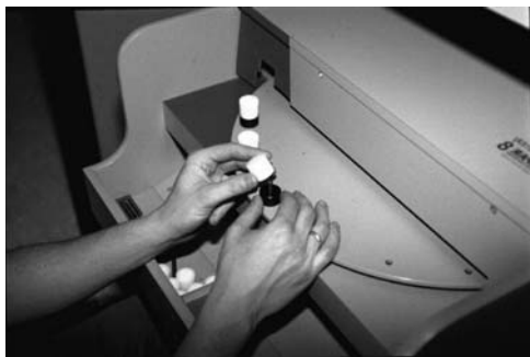
Fig. 7 – Standardised assembly work station (3 components) – performance standing or sitting.
