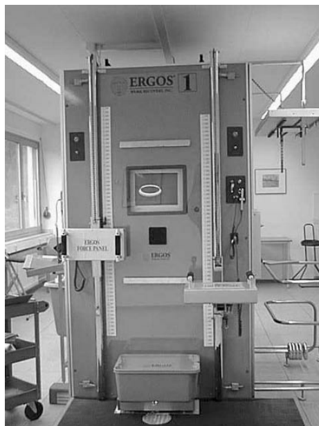
Fig. 4 – ERGOS: Test station for static and dynamic lifting.
