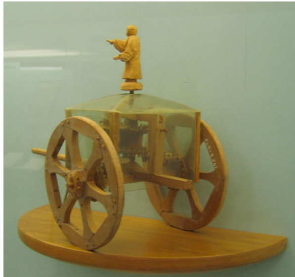
Fig. 15 South-pointing Chariot (Andy Dingley Creative Commons license via Wikimedia Commons)
