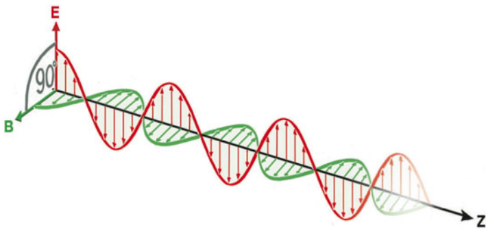
Fig. 3 Linearly polarized electromagnetic wave, a combination of equal amounts of RCP and LCP (C. Phipps/F. Wicke)
