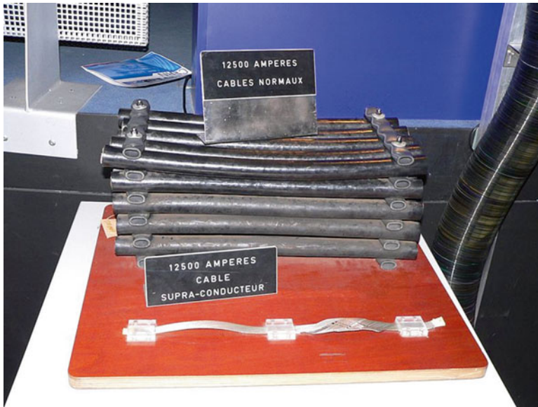
Fig. 26 Normal vs. Superconducting cables, both rated for 12,500 Amps. (Rama Wikimedia Commons)
