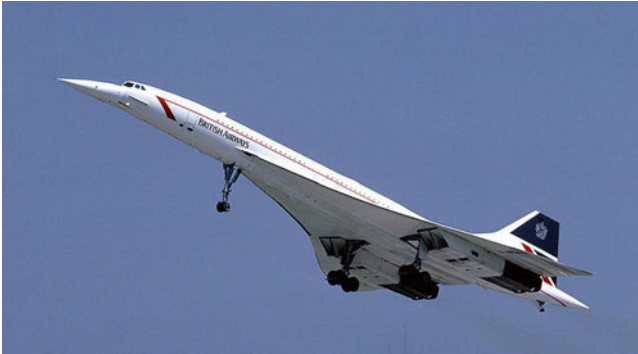
Fig. 15 The Concorde. The droopy nose gave the pilot a better view for takeoff and landing (Eduard Mamet, permission under Creative Commons Attribution-ShareAlike 3.0 Unported License)
