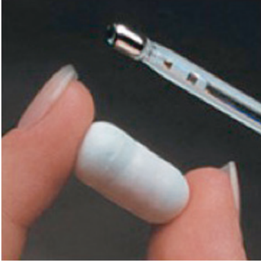
Fig. 6 CofTemp ingestible sensor
