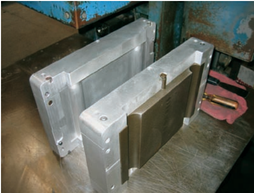
FIGURE 15.8 The next five figures document the casting process for the cable clamps. Shown here is the mold for making the wax patterns. The die is open, showing a pattern ready to be removed.
