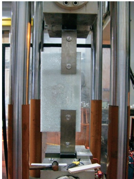
FIGURE 17.11 Pull testing was conducted to determine the capacity of the laminated panels.
