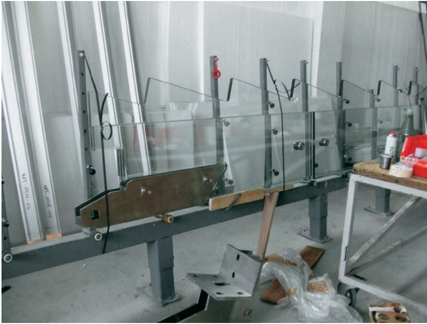
FIGURE 17.6 The glass beams were fully assembled by the fabricator of the laminated glass panels and shipped in 30 ft (9.1 m) lengths to the job site.
