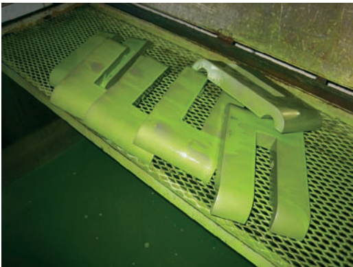
FIGURE 15.12 Each casting is tested for surface cracks using a die-penetrant technique. A percentage of parts are also radiographed to detect the presence of voids.
