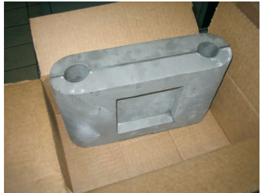
FIGURE 15.11 The ceramic is broken away to reveal the cast metal.
