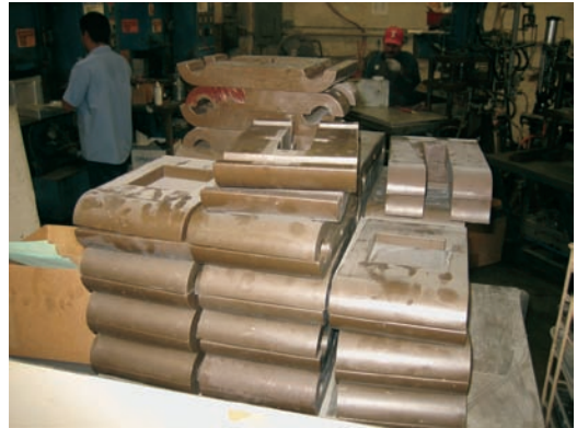
FIGURE 15.9 A pattern is made for each part to be produced.
