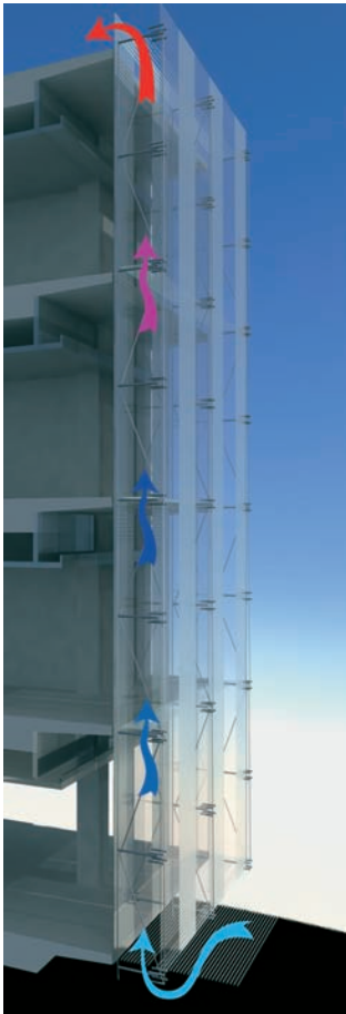
FIGURE 13.10 Diagram of airflow through cavity wall.
