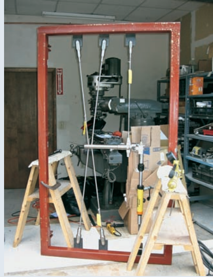
FIGURE 11.14 Test setup to simulate the rotation problem identified during mockup testing.
