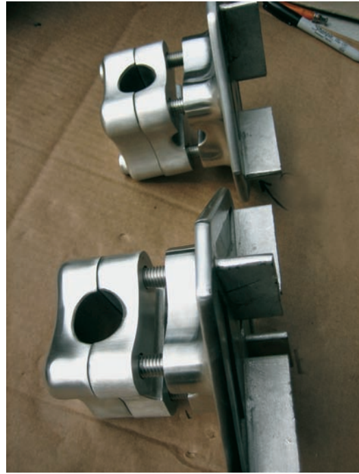
FIGURE 14.8 Four-part cast stainless steel cable clamp and glass-fixing assemblies (minus the cap plate). The glass sits on the blades to the right of the assembly.
