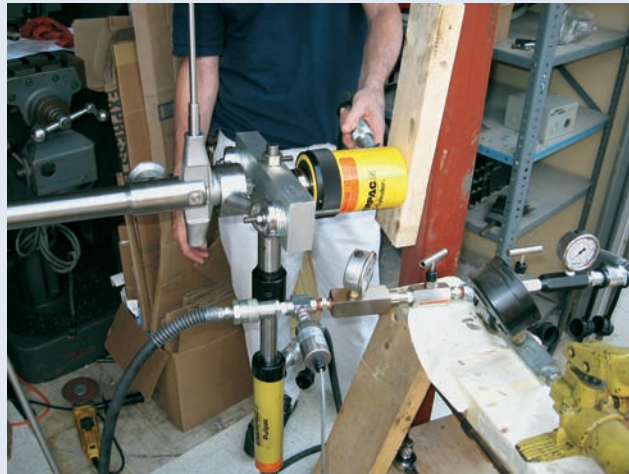
FIGURE 11.15 A hydraulic cylinder at the strut end accommodates the simulation of dead and wind loads on the rod truss–glass system interface.
