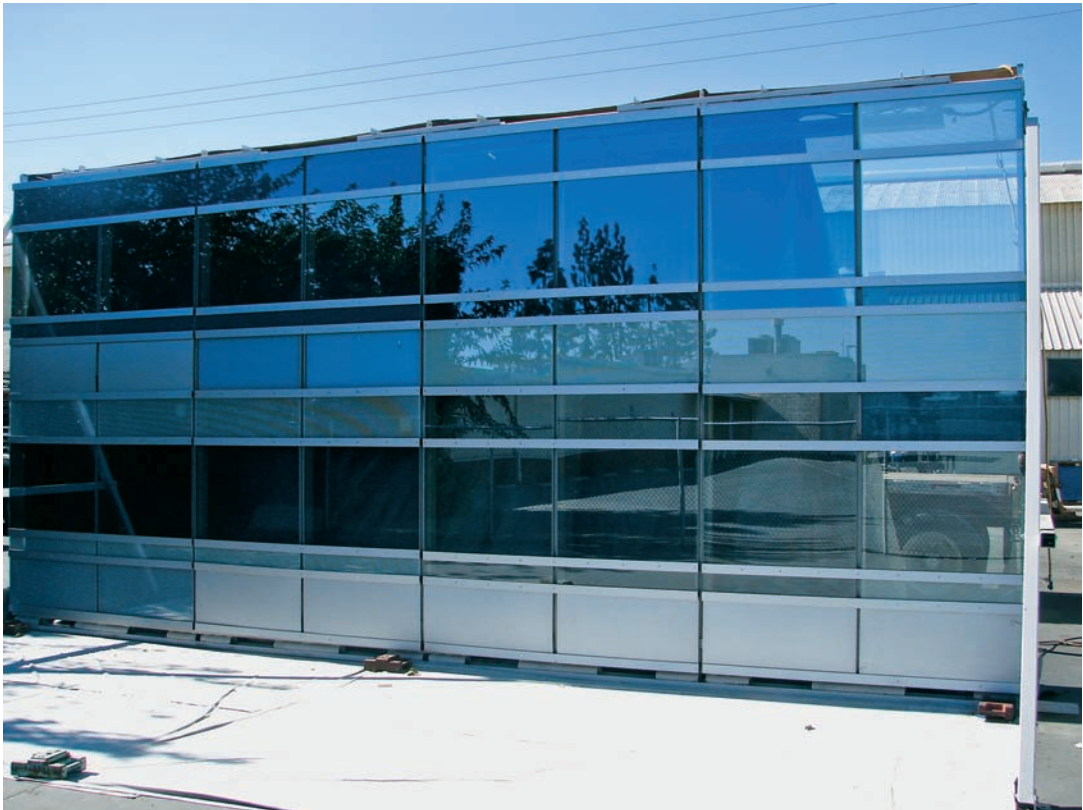
FIGURE 7.14 It is always a challenge to anticipate what the many variations of glass will look like in place. Enclos constructed a gimbaled rack for the simultaneous evaluation of large glass mockups under varying light conditions.
