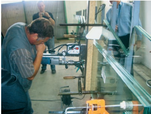
FIGURE 6.9 Three two-ply laminates are aligned at the pin locations, and a jig and a magnetic drill are used to core a high-tolerance hole through all six layers of disk material.
