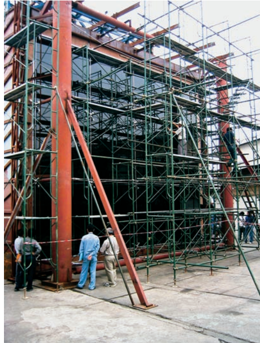
FIGURE 8.13 Extensive testing was carried out on this large facade mockup.
