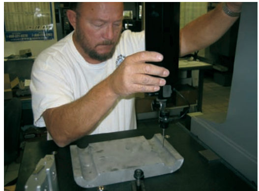
FIGURE 15.13 Each casting is inspected to ensure conformance with the required tolerance prior to machining.
