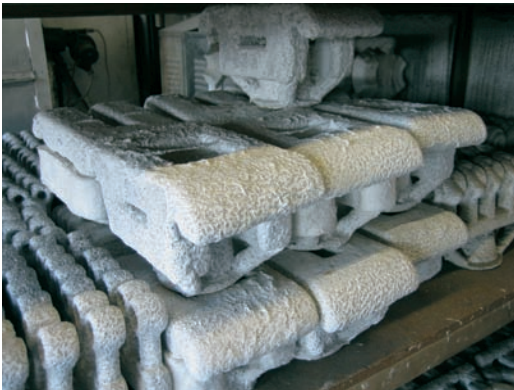
FIGURE 15.10 A ceramic slurry creates a shell around the pattern, which is fired to harden the ceramic and melt out the wax; molten metal is then poured into the void.
