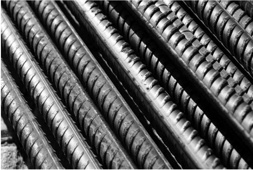
Figure 7.5 Rebar showing the ribbed surface designed to improve the bond with concrete.
