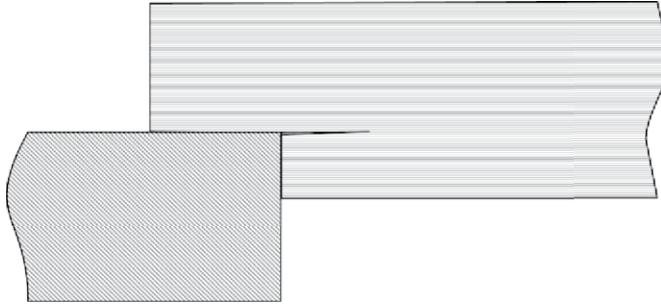
Figure 11.4 Splitting of a timber beam with a notched end.
