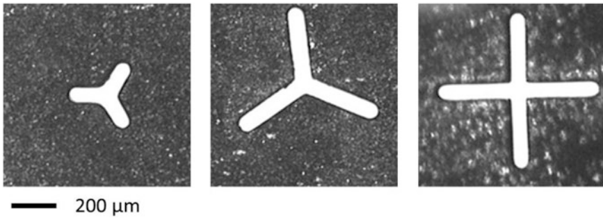
Fig. 11 Three different cross-sectional shapes of the capillary holes of the spinneret (trilobal short, trilobal long, cruciform); bar 200 \mu\text{m} . (Data source: Leibniz-Institut für Polymerforschung Dresden e. V.)
