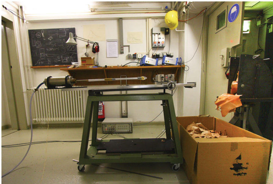
Fig. 2.4 Air gun for the projectile experiments. A detailed description, including all measurements can be found in Iovita et al. (2014)
