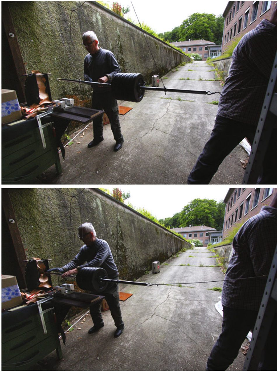
Fig. 2.5 Thrusting pendulum, in this photo loaded with six 10 kg weights
