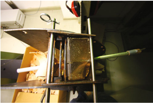
Fig. 2.3 View from above of the target with the spear having exited at the back. Note the four layers, from left to right: Leather, gelatin, polyurethane “bone” plate, gelatin
