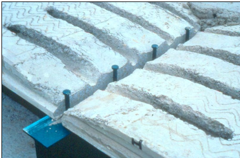
Figure 4.3 Composite beams supporting precast hollow-core units
